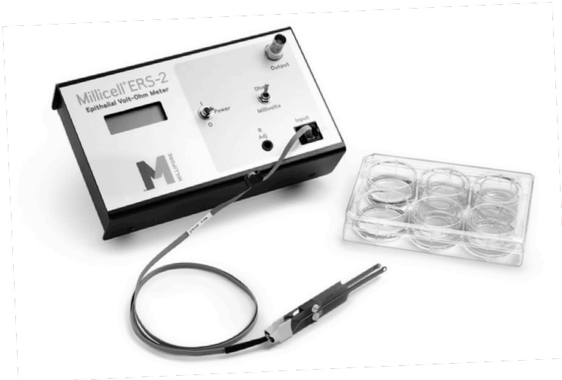
Figure 2.3; The Millicell ERS-2 voltohmmeter and chopstick electrodes from the product literature of the manufacturers, Merck Millipore. To measure TEER, the electrodes are placed at a perpendicular angle to the surface of the monolayer, with the long chopstick arm in the basolateral well and the short chopstick arm in the apical well, just above the monolayer.
