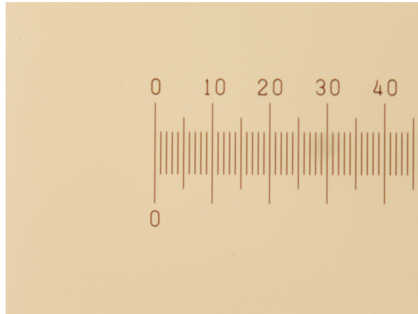
Figure A.1: Image of a graticule slide taken at x100 magnification using an epifluorescence microscope (Olympus BX40) fitted with a digital camera (Olympus E-400). The rule has 1mm/0.01 divisions (10 \mu\text{m} ). From this image, the image height has been determined as 0.55 mm.
