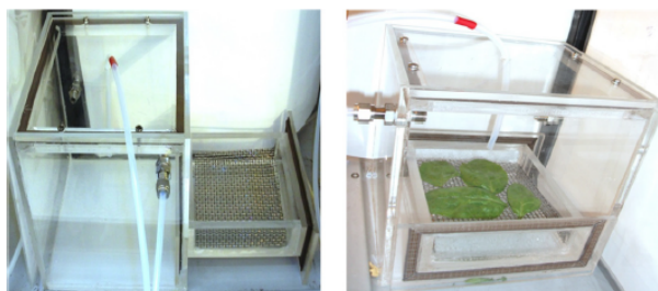
Figure 10. Modified ozone fumigation system.
