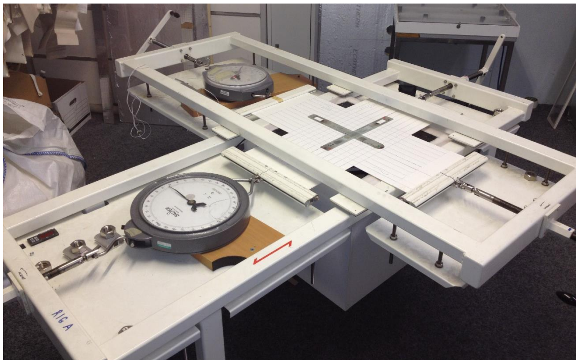
Figure 2.11 Floating biaxial test rig developed by Architen Landrell
