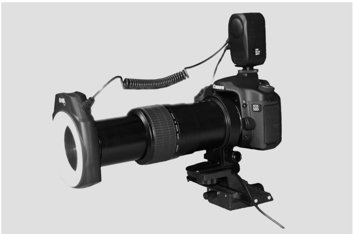
Figure 5.8 Canon EOS 50D digital SLR camera coupled with a Canon MP-E 65mm 1-5x extreme macro lens, a LED ring light is shown mounted on the front of the lens
