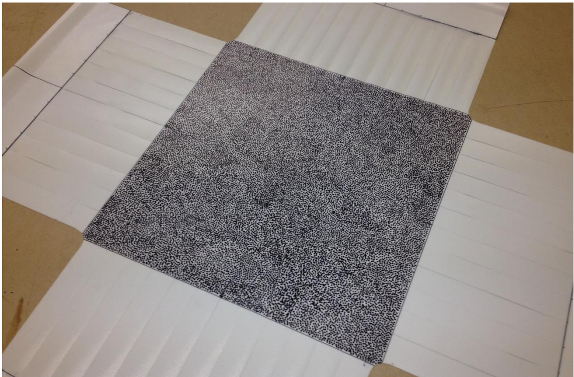
Figure 3.15 Biaxial cruciform specimen (CMX220) prepared for shear test with stochastic speckle pattern for Digital Image Correlation (DIC) analysis. The pattern has been applied to the specimen with a permanent marker pen. While more rapid methods of applying the pattern are available, e.g. spray paint, the pen method reduces the risk of scrapping the specimen.
