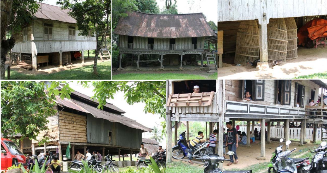
Figure 6.05 Multi-purposes of the gap under the house Serves as a temporary storage space (above), Used as a space for social activities (below)
