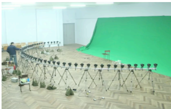
Arc of still cameras used to create a time-slice film
