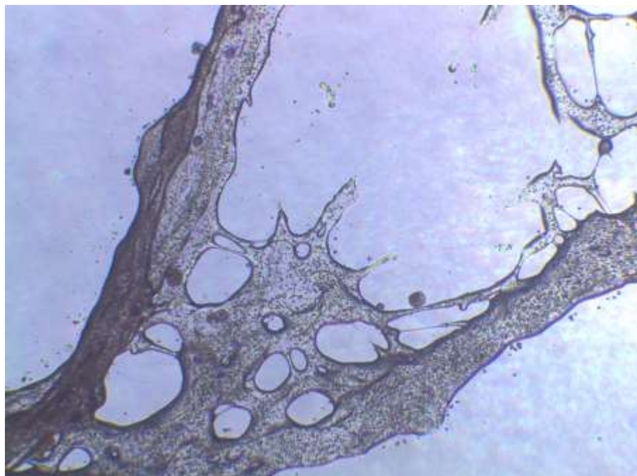
Figure 3.17 Shows the surface of high concentration [40mg/ml] polyHEMA coating which was broken after 14 days
