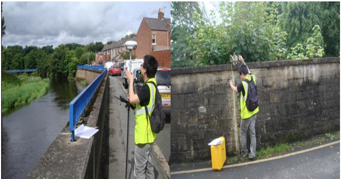
Figure 4.13 The field work to measure the height of the flood defences in Morpeth.
