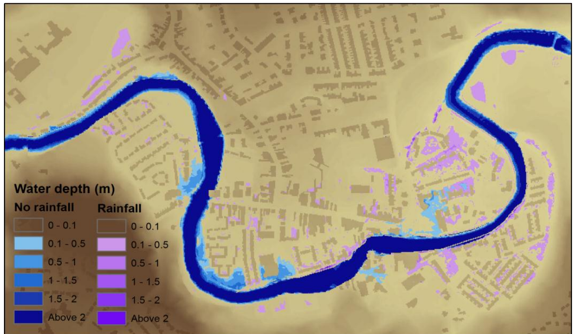
Figure 5.32 Inundation maps at 11am with and without rainfall in the town centre domain.
