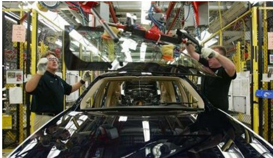
Figure 1.1 Installing the front windshield
