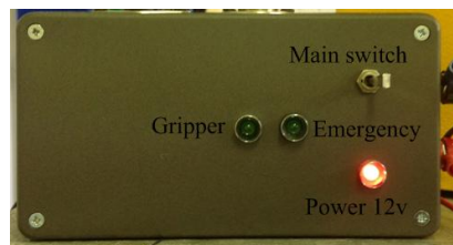
Figure 4.17 A stand-alone signal conditioning box for the robot gripper located on the robot controller
