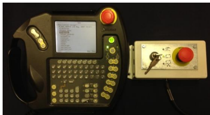
Figure 4.18 Emergency stop buttons from MCP and external control box
