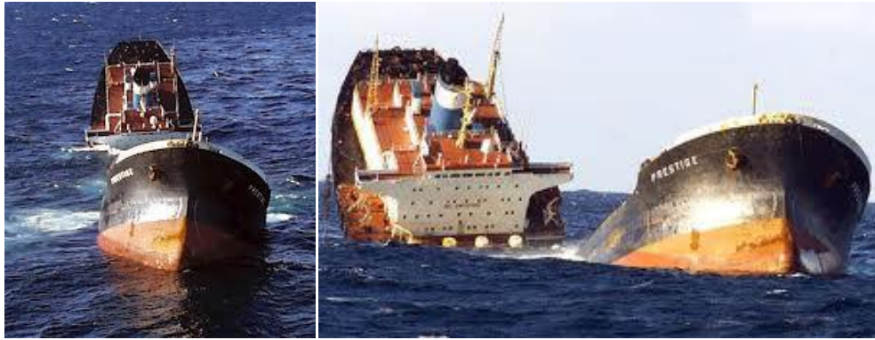
Figure 10: The Prestige and her structure failure
