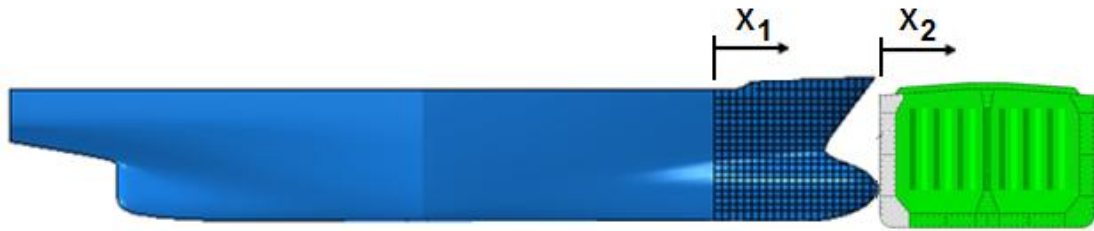
Figure 133: The simplified energy dissipation system of ship model for deformable ship-ship collision.
