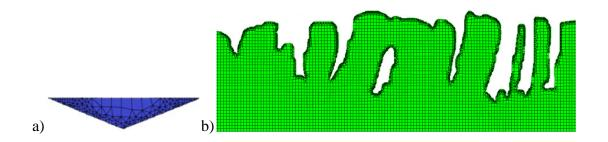
Figure 6-21. Meshes produced by OOF2 modelling (a) diamond indenter and (b) annealed Cu-Sn coating with low density.
