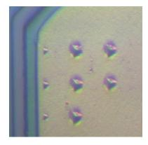
Figure 5-24. Microscopic image of the Au thin film, presenting visible large indentations illustrating reduction in stiffness.
