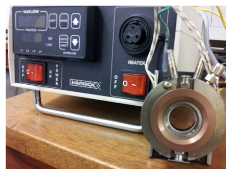
Figure 4. Picture of the high-temperature cell and the temperature controller used in this work.
