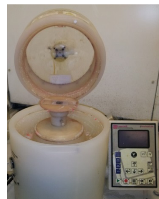
Figure 10. Photograph of the spin coater used to prepare polymer films.
