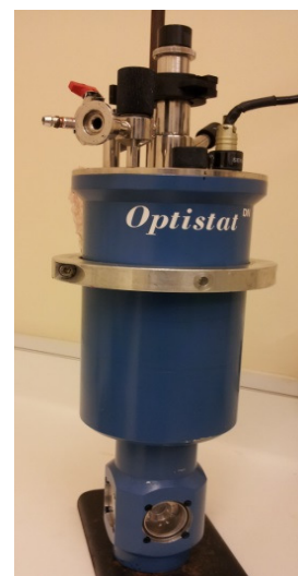
Figure 3. Photograph of the cryostat used for low-temperature studies.
