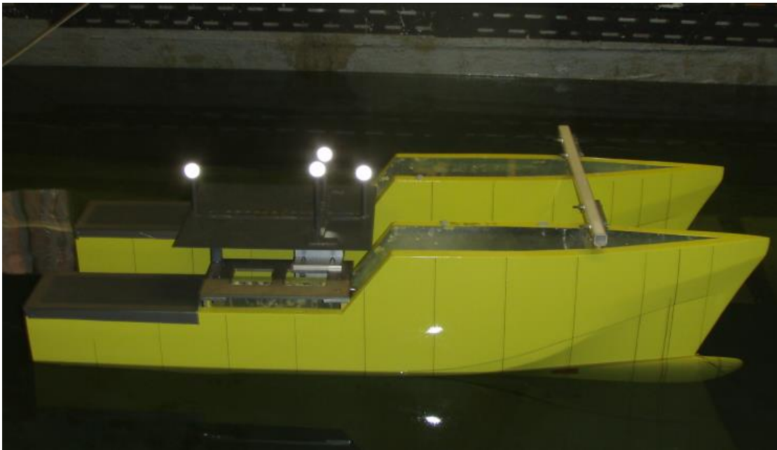
Figure 4.8: Rigid model in position during zero speed motions response measurements
