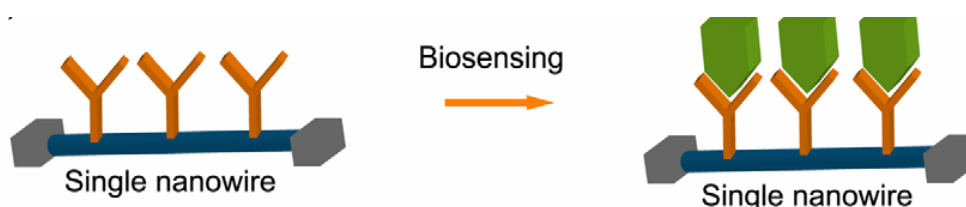
Scheme 1.1. When functionalized with appropriate ‘capture probes’ (left), nanowires can act as transducers for label-free electrical detection of chemical and biological species (right). Reproduced from reference 45
