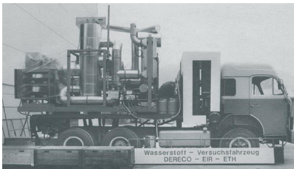
Figure 2-6: A prototype truck running on the MTH system, built by Taube et al , 1985 46
