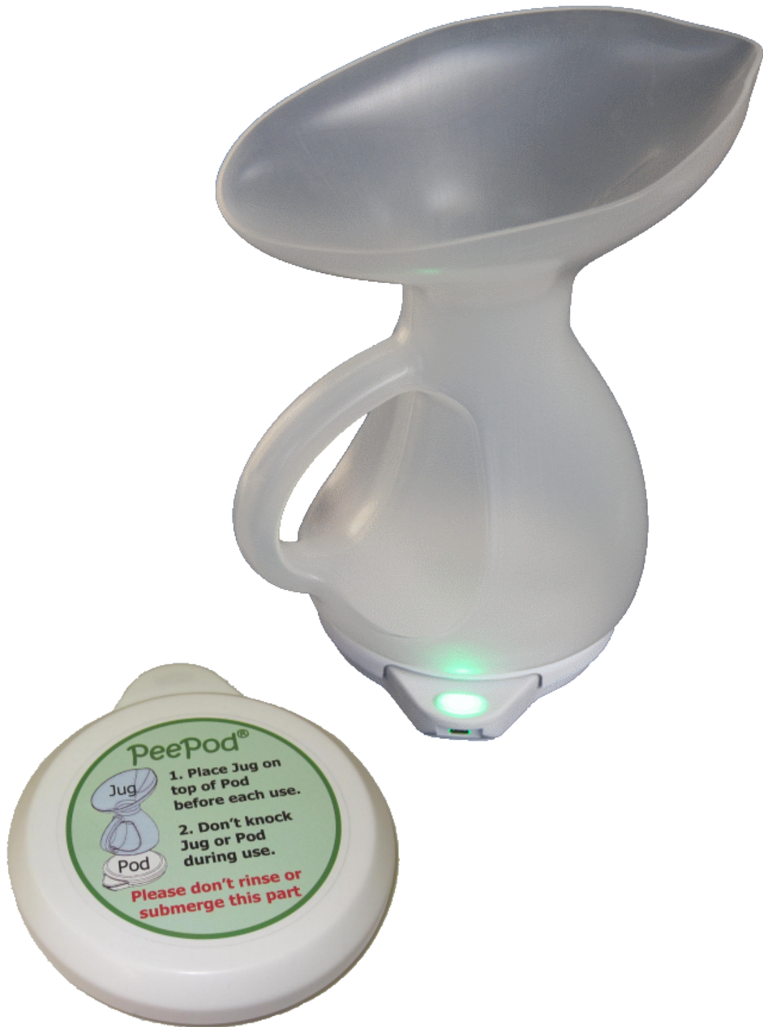
Figure 6.3 The PeePod with the collecting jug positioned on top of the pod, and the pod alone showing user instruction label. A green LED indicates the state of the device to the user according to Figure 6.2.
