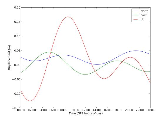
Figure 2.4: Computed solid earth tide on 5th August 2011 for Perth, Australia.
