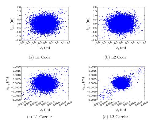
Figure 6.32: Lag plot for the AR(p) whitened residuals of GPS SVN05 at GUAM, where p is determined automatically using AIC.
