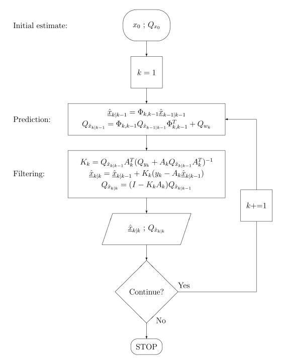
Figure 3.2: Flowchart showing the Kalman filter process
