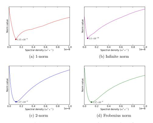
Figure 5.31: Norm of the cross-correlation matrix for lag 10 for different spectral densities. In each case the minimum norm is shown along with the equivalent process noise value.
