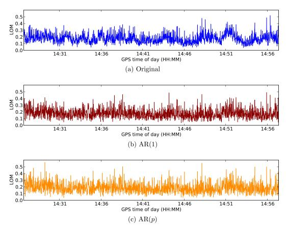
Figure 7.7: Example time series of local overall model test statistic values calculated using post-fit residuals for FALK, where minimum  $F_{\alpha_{m-k}} = 1.171$
