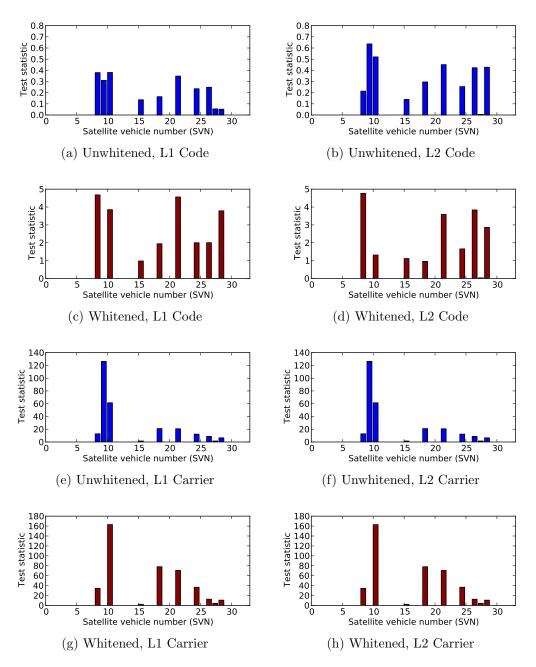
Figure 7.14: Local slippage test statistic values computed using post-fit residuals at 09:10:56 for ALBM dataset. In each case the absolute values are taken, i.e. negative values are now positive.
