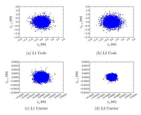
Figure 6.30: Lag plot for the AR(p) whitened residuals of GPS SVN05 at ABPO, where p is determined automatically using AIC.
