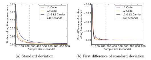
Figure 5.9: Standard deviation of the lag 0 autocovariance for satellite G09 of the ALBM dataset with increasing sample size.
