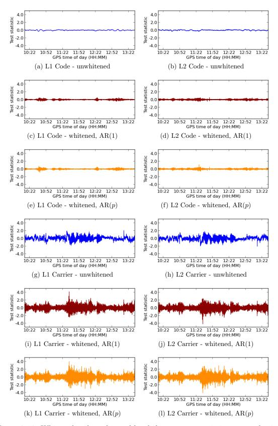
Figure 7.13: Whitened and unwhitened local slippage test statistic computed using post-fit residuals for GPS SVN17 at ALBM.
