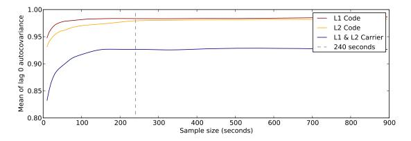
Figure 5.8: Mean of the lag 0 autocovariance for satellite G09 of the ALBM dataset with increasing sample size.
