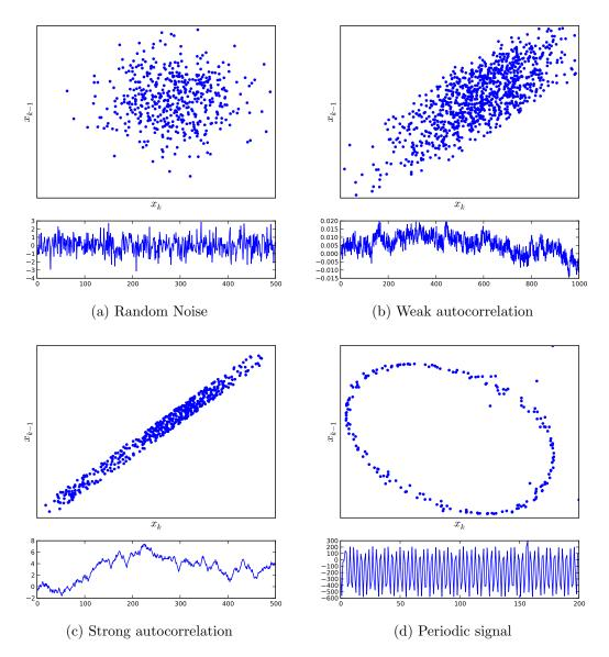
Figure 5.10: Examples of lag plots for different noise types with the corresponding time series shown below.
