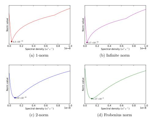
Figure 5.29: Norm of the cross-correlation matrix for lag 1 for different spectral densities. In each case the minimum norm is shown along with the equivalent process noise value.
