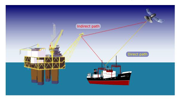
Figure 2.3: An illustration of the direct and indirect paths of a GNSS signal at the antenna. The diagram is not to scale.
