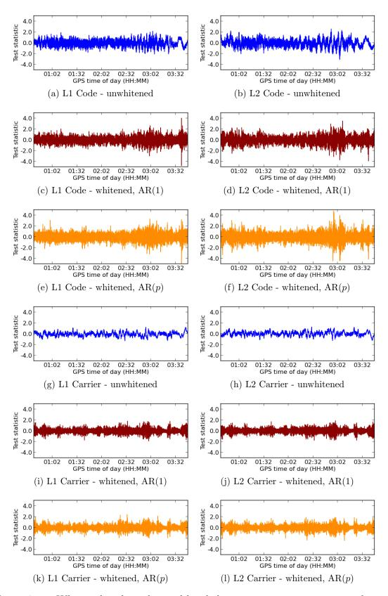
Figure 7.11: Whitened and unwhitened local slippage test statistic computed using post-fit residuals for GPS SVN05 at FALK.
