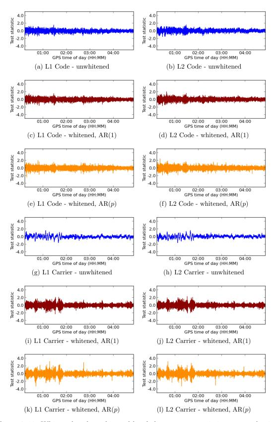
Figure 7.10: Whitened and unwhitened local slippage test statistic computed using post-fit residuals for GPS SVN05 at ABPO.
