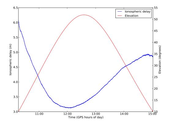
Figure 2.1: Estimated ionospheric path delay between satellite G05 and a receiver located in Perth, Australia on 5th August 2011 generated using the E-HP/PPP software.
