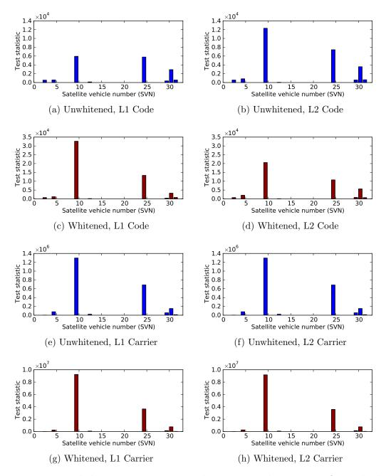
Figure 7.15: Local slippage test statistic values computed using post-fit residuals at 23:48:03 for FALK dataset. In each case the absolute values are taken, i.e. negative values are now positive.
