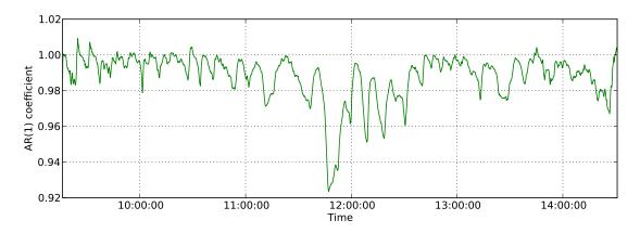
Figure 6.2: Variation of the AR(1) coefficient estimated using the forwards least squares method over a satellite pass (G9 L1 Code).
