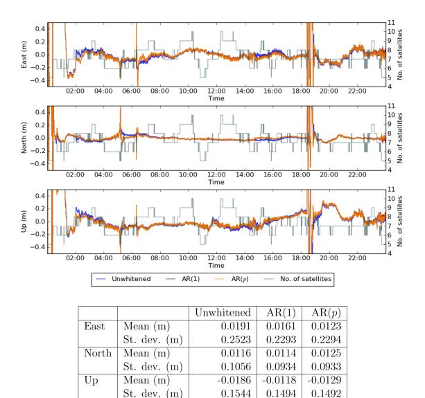
Figure 7.21: Local ENU positions for GUAM using the unwhitened local slippage test statistic, AR(1) whitened local slippage test statistic and AR(p) local slippage test statistic with the level of significance set at 99%. In all cases the post-fit residuals were used to calculate the test statistics. The mean and standard deviation for each plot are shown in the table below.
