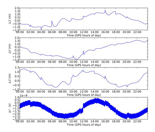
Figure 2.5: Difference between broadcast and IGS Final orbits and clocks for GPS SVN01 on 1st January 2012
