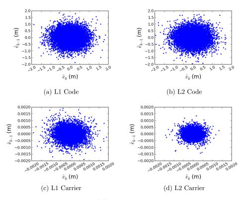
Figure 6.31: Lag plot for the AR(p) whitehed residuals of GPS SVN05 at FALK, where p is determined automatically using AIC.
