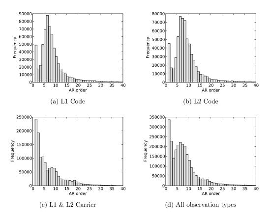
Figure 6.23: Histogram showing the frequency at which each AR order has been chosen using AIC for FALK dataset.
