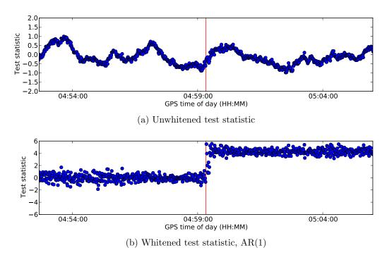
Figure 7.18: Effect on the local slippage test statistic of a 'jump' in time series of post-fit residuals statistic caused by a change in the geometry of the least squares solution.
