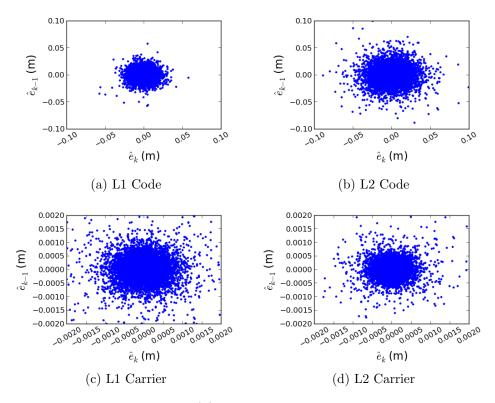
Figure 6.33: Lag plot for the AR(p) whitened residuals of GPS SVN17 at ALBM, where p is determined automatically using AIC.
