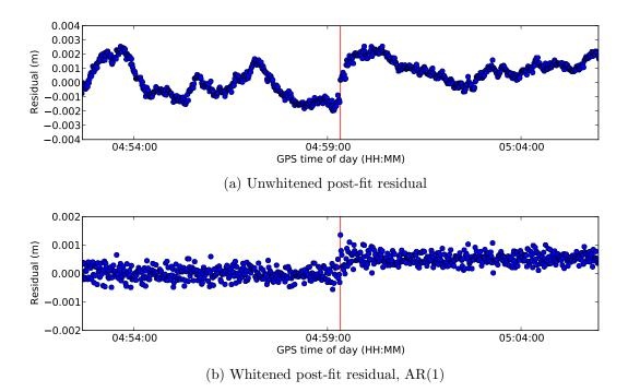
Figure 7.17: 'Jump' in time series of post-fit residuals statistic caused by a change in the geometry of the least squares solution.
