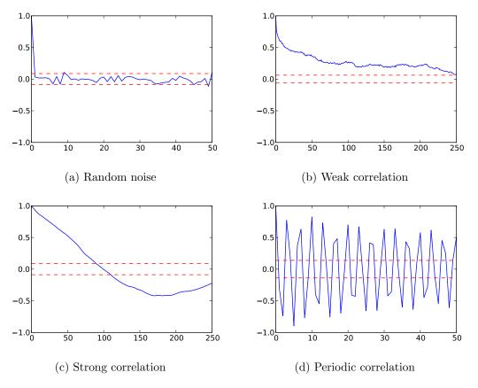
Figure 5.19: Examples of autocorrelation plots for different noise types.
