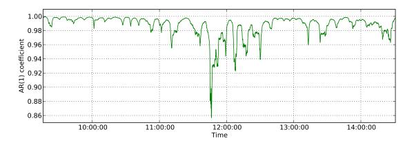
Figure 6.3: Variation of the AR(1) coefficient estimated using Burg's method over a satellite pass (G9 L1 Code).
