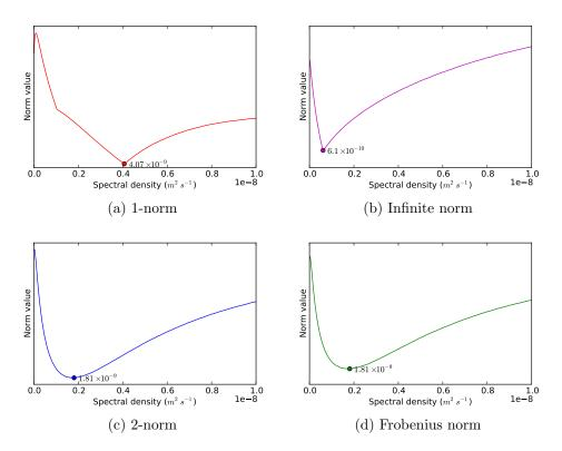
Figure 5.33: Norm of the cross-correlation matrix for lag 30 for different spectral densities. In each case the minimum norm is shown along with the equivalent process noise value.
