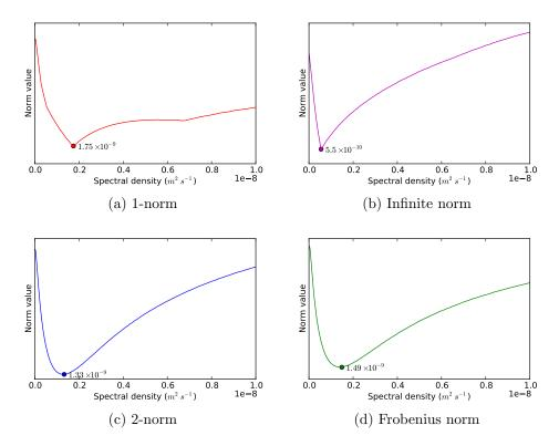
Figure 5.32: Norm of the cross-correlation matrix for lag 15 for different spectral densities. In each case the minimum norm is shown along with the equivalent process noise value.
