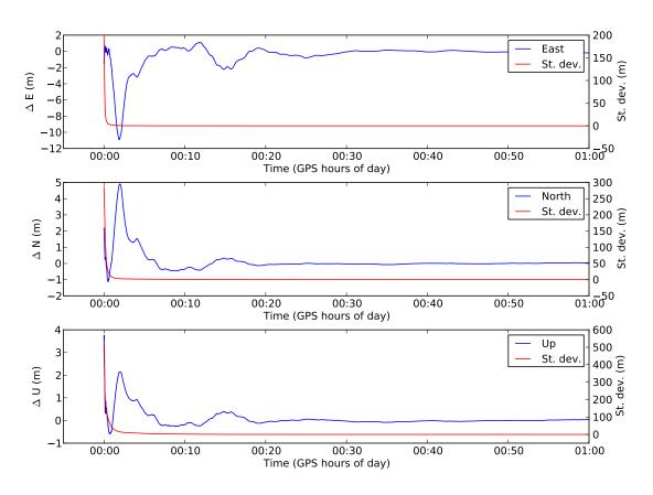
Figure 2.6: Difference between coordinates calculated using PPP in 'kinematic mode' and the known coordinates during the convergence period for ABPO (located on the island of Madagascar in the Indian Ocean) on 25th December 2009.
