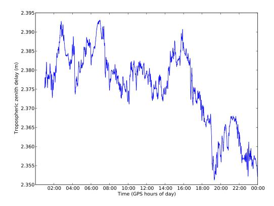
Figure 2.2: Estimated tropospheric zenith delay at a receiver located in Perth, Australia on 5th August 2011 generated using the E-HP/PPP software.
