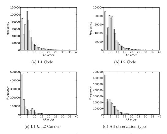
Figure 6.24: Histogram showing the frequency at which each AR order has been chosen using AIC for GUAM dataset.
