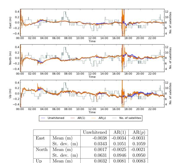
Figure 7.20: Local ENU positions for FALK using the unwhitened local slippage test statistic, AR(1) whitened local slippage test statistic and AR(p) local slippage test statistic with the level of significance set at 99%. In all cases the post-fit residuals were used to calculate the test statistics. The mean and standard deviation for each plot are shown in the table below.
