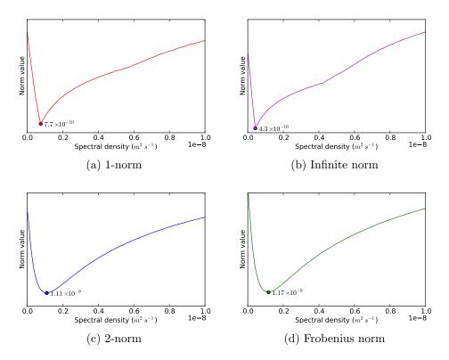
Figure 5.30: Norm of the cross-correlation matrix for lag 5 for different spectral densities. In each case the minimum norm is shown along with the equivalent process noise value.
