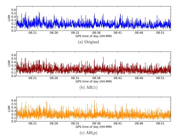
Figure 7.8: Example time series of local overall model test statistic values calculated using post-fit residuals for GUAM, where minimum  $F_{\alpha_{m-k}} = 1.277$
