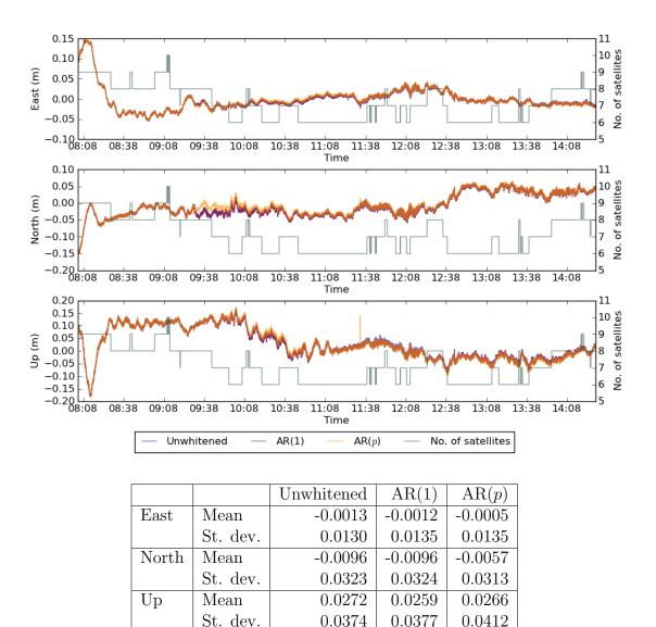
Figure 7.22: Difference in local ENU positions relative to the double-difference 'truth' solution for ALBM using the unwhitened local slippage test statistic, AR(1) whitened local slippage test statistic and AR(p) local slippage test statistic with the level of significance set at 99%. In all cases the post-fit residuals were used to calculate the test statistics. The mean and standard deviation for each plot are shown in the table below.
