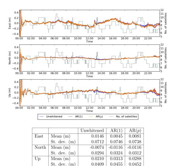
Figure 7.19: Local ENU positions for ABPO using the unwhitened local slippage test statistic, AR(1) whitened local slippage test statistic and AR(p) local slippage test statistic with the level of significance set at 99%. In all cases the post-fit residuals were used to calculate the test statistics. The mean and standard deviation for each plot are shown in the table below.
