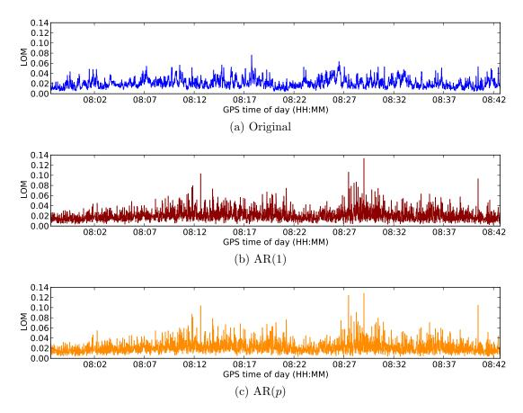
Figure 7.9: Example time series of local overall model test statistic values calculated using post-fit residuals for ALBM, where minimum  $F_{\alpha_{m-k}} = 1.326$
