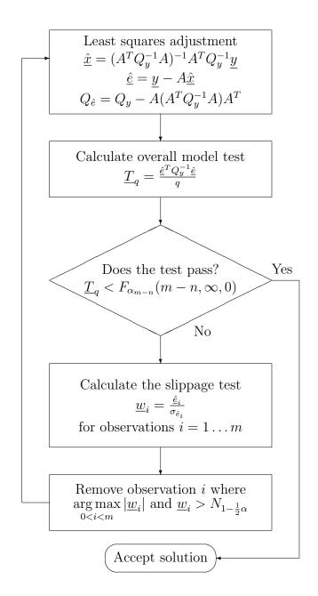
Figure 4.4: Quality control procedure for batch processing.
