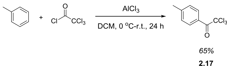
Scheme 2.7 The synthesis of 2,2,2-trichloro-1-(4-tolyl)ethan-1-one ( 2.17 )
