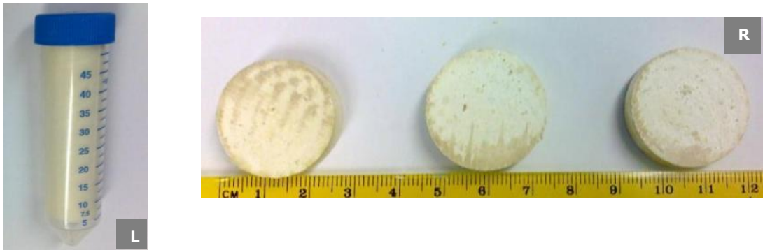
Fig. 3-3: EPHP S10 series produced after polymerisation in cylindrical cone mould (L) and dried EPHP Disks, diameter = 2.6 cm and thickness = 5-7 mm (R).
