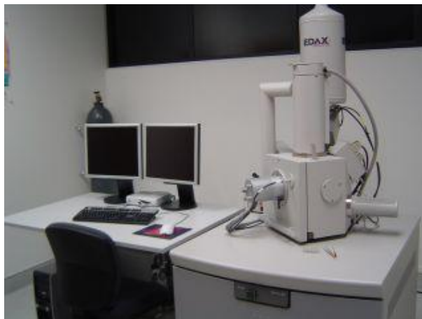
Fig. 3-9: typical SEM instrument facilities. The SEM is recognisable on the right, while the imaging and editing monitors are visible on the left.
