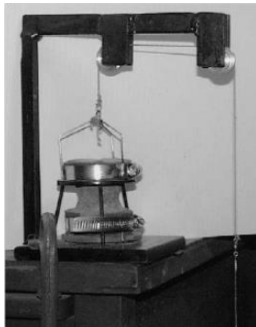
Figure 2.43 Tensile strength measurement method (a) sample preparation in soil lathe and (b) clamp and pulley apparatus (after Ibarra et al. 2005).
