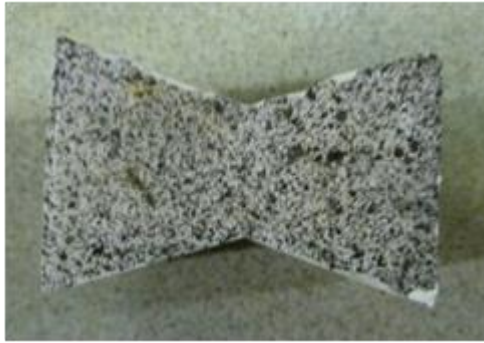
Figure 4.17 Sample with speckle pattern.
