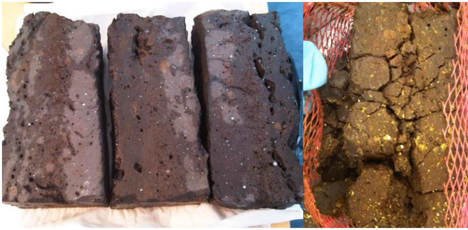
Figure C.5 – Slag blocks prior to suspension in leachate wells
