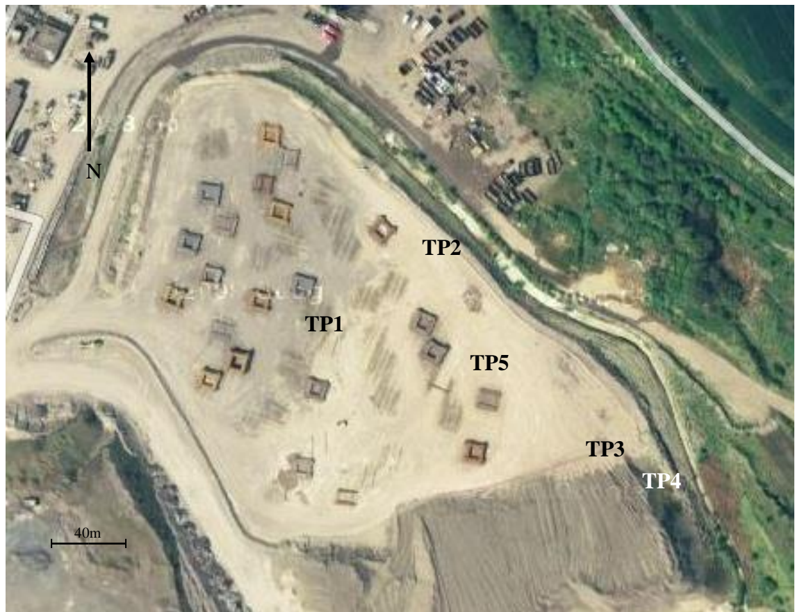
Figure 4.3 – Location of trial pits in Cell 1 of Yarborough Landfill, Scunthorpe (Google Maps 2010) The square features are stacks of girders, stored periodically in this area of the site
