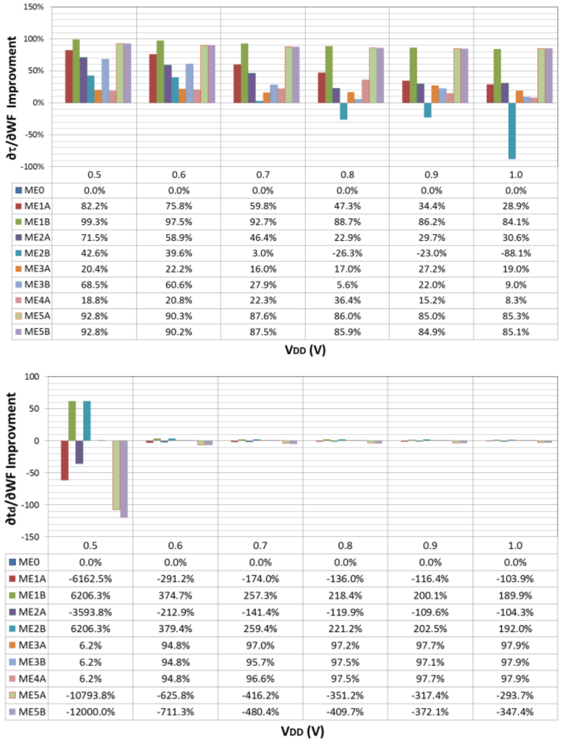
Figure 4.25 Improvement of sensitivity of \tau and t_d to load width against V_{DD}
