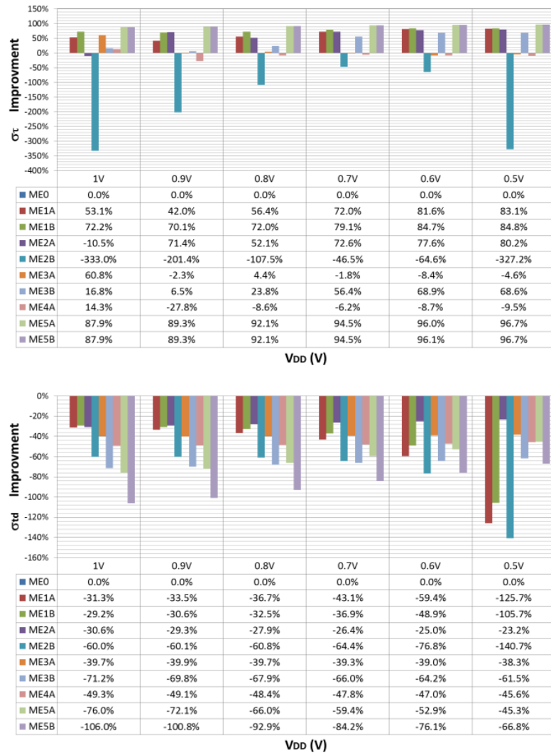
Figure 4.32 Improvement of standard deviation of \tau and t_d to that of ME0 against V_{DD}
