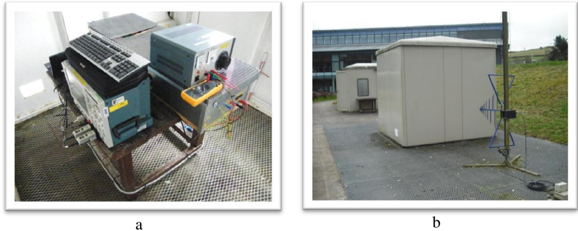
Figure 5-12: a) Pulse test setup for radiated emissions, b) OATS.
