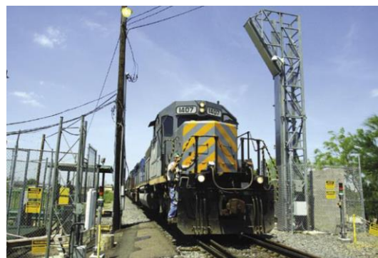
Figure 3-3 X-ray scan of a container loaded in a train
