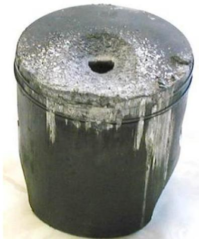
Figure 5.3: Piston Damage caused by late ignition
