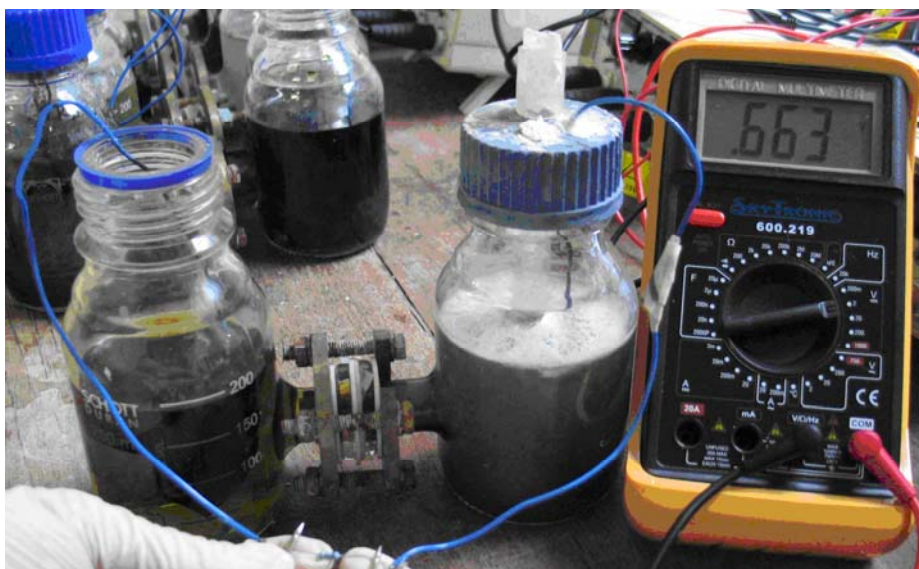
Figure 9.1 Two-chamber Microbial Fuel Cell design with membrane chamber, organic substrate is oxidized in the anodic compartment and electrons were transferred via an external resistor to the cathode. The voltage output was measured continuously by a high impedance multimeter.
