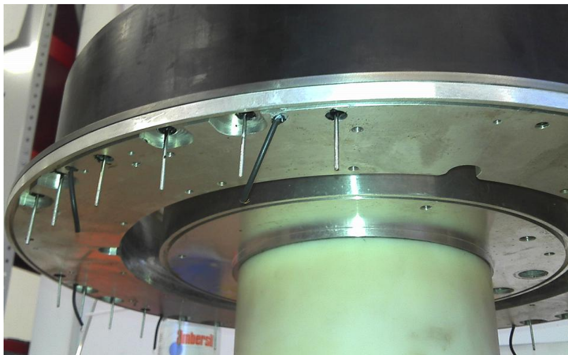
Figure D 6. Seal stator, showing connection pins.
