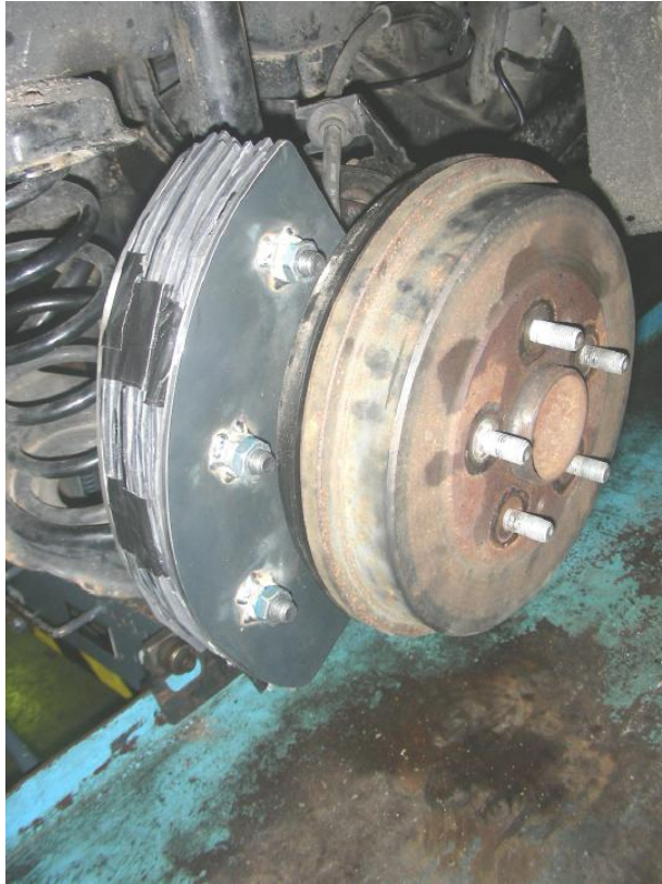
Figure 2.14. Un-sprung mass experimentation by Lotus [74].
