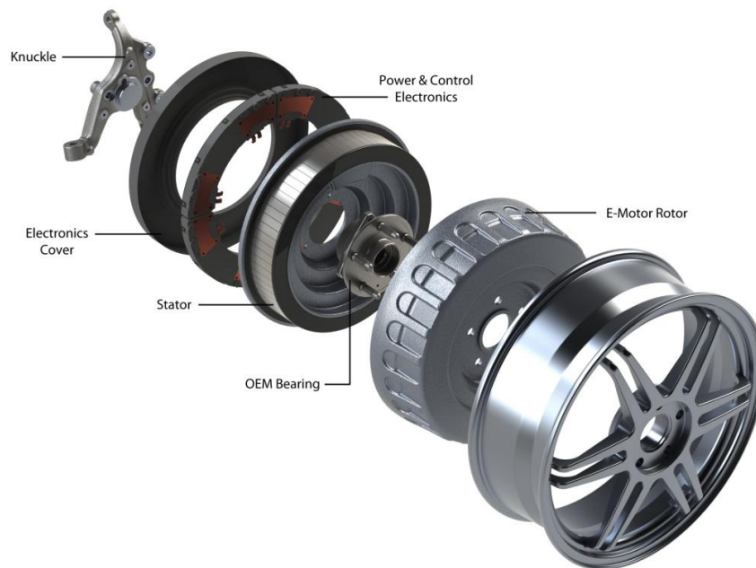
Figure 2.4. Protean Electric in-wheel motor assembly.
