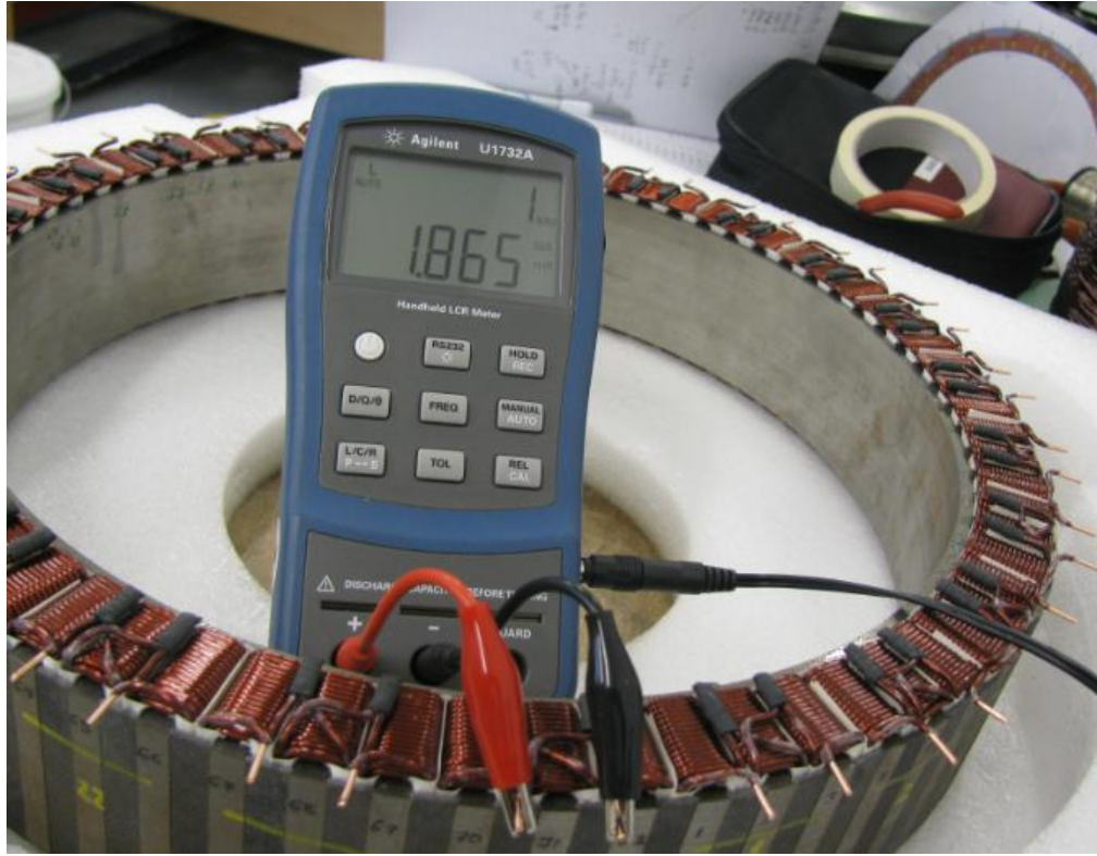
Figure D 4. Coil and phase inductance and resistance measurement.
