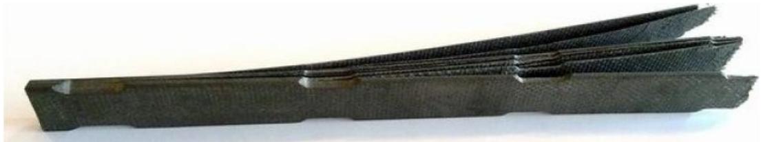
Figure 4.16. Delaminating of a laminated magnetic wedge [105].
