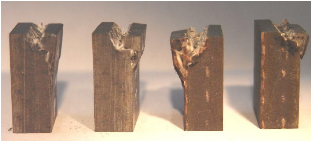
Figure 4.19. Test SPIndu wedge after mechanical failure [105].
