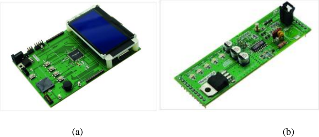
Figure 4.5: The ATA2270b-EK1 RFID reader kit from ATMEL used to program the memory content of the tags. The main board (a) and the RFID reader daughter board (b) are shown above.
