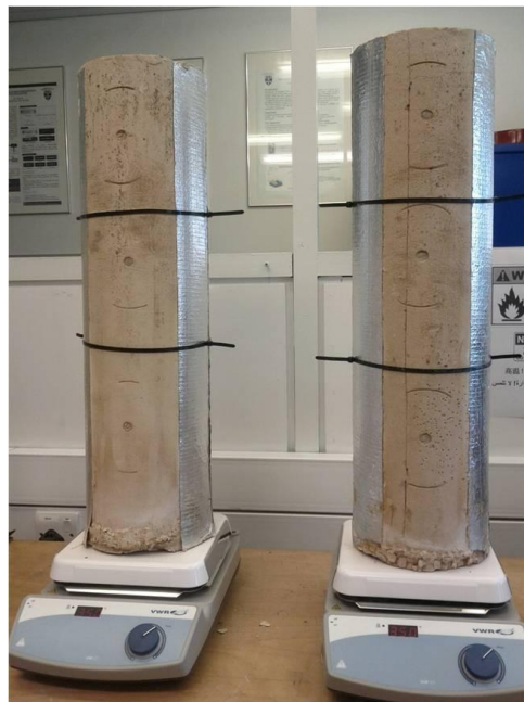
Figure 6.6: picture of experimental setup showing strip of aluminium foil removed.
