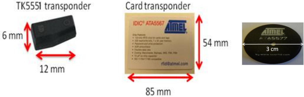
Figure 3.13: Three commercially available tags used in study and their dimensions.
