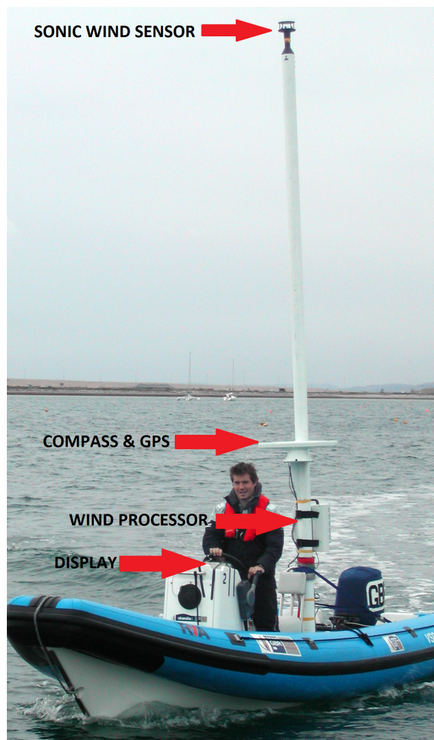
Figure 34 – RYA weather boat with instrumentation and wind processor.
