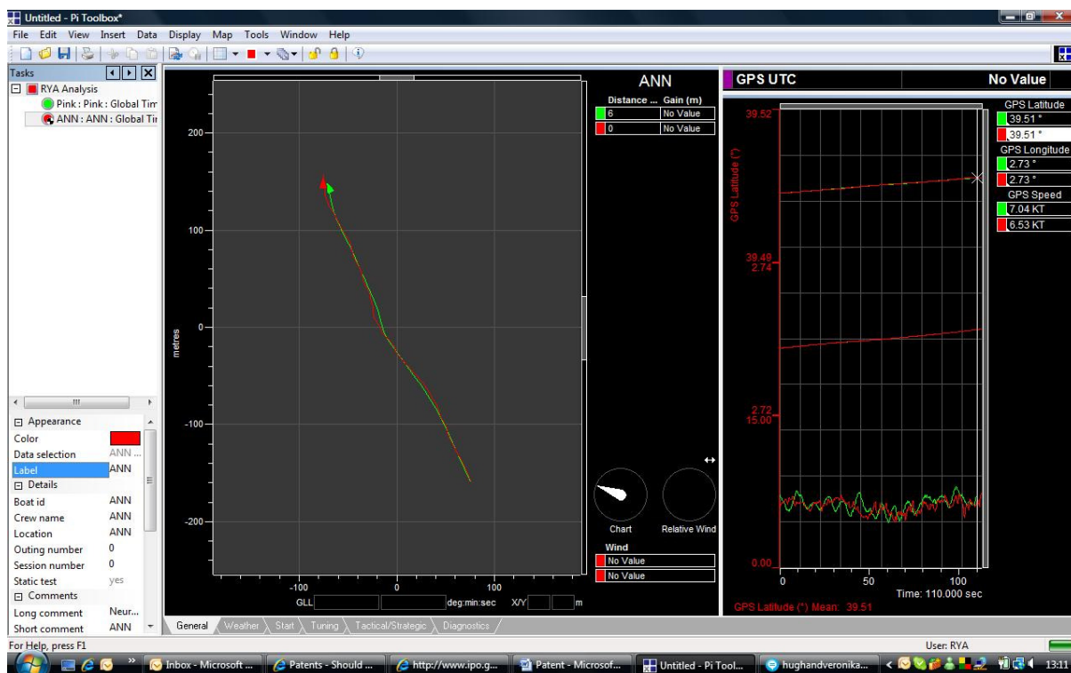
Figure 60 - The comparative analysis of performance through producing an artificial latitude and longitude ANN trace
