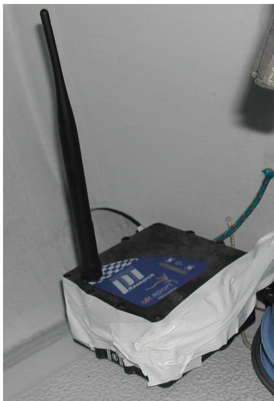
Figure 29 – Pi Research data logger secured onboard a Yngling boat.
