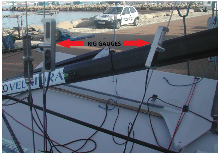
Figure 35 – Custom strain gauges fitted on a 49er
