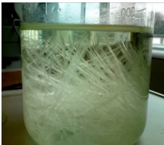
Figure 3-1 : Re-crystallization of the prepared ethaline melt at 15 °C, these crystals disappeared when the ethaline melt was heated to a temperature >20 °C
