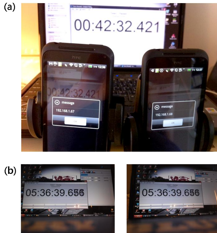
Figure 4-4: The system synchronisation experiment, showing (a) the handset and monitor configuration, with examples of captured images from the two handsets at the same epoch (b).
