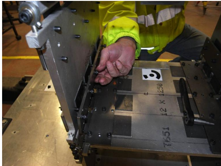
Figure 5-7: Unscrewing some mounting bolts of the three-story stainless steel frame.
