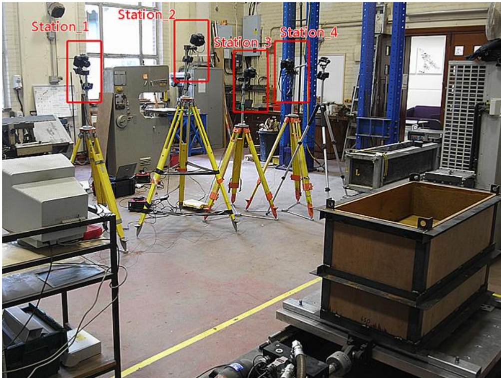
Figure 6-5: Configuration of imaging stations for shaking table test.
