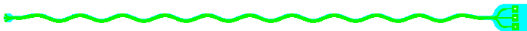
Figure 2.1. The sinusoidal probe first generation. The recording end was a parylene disc of 100 \mu\text{m} diameter, out of which the three metal electrode sites protrude. There were three electrode recording sites to isolate single-unit activity through triangulation recording. The electrode body was 20 \mu\text{m} deep and 35 \mu\text{m} wide, and 5.5mm long, consisting of 10 sinusoidal cycles of 100 \mu\text{m} amplitude and 500 \mu\text{m} period. Each electrode connected to a bondpad, which was approximately 400 \mu\text{m}^2 . Recording sites had an area of 96 \mu\text{m}^2 and the distance between the recording sites were 40 \mu\text{m} centre to centre. Distance between the electrode recording tracks are 5 \mu\text{m} edge to edge.
