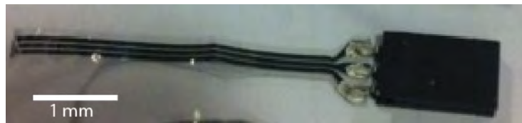
Figure 3.8. Connector bonded to the electrode bondpad region using silver paint.
