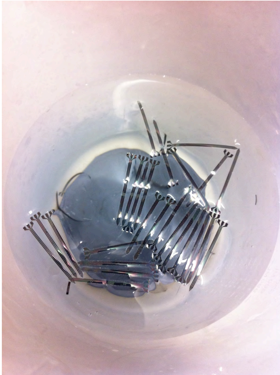
Figure 3.3. Premature device release with BHF use to remove titanium mask. Device interaction leads to probe damage.
