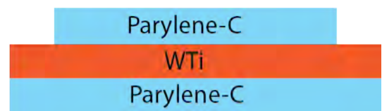
Figure 2.4. Summarised edge-on fabrication for the sinusoidal probe. A) Ebeam deposition of 1 \mu\text{m} aluminium as a sacrificial layer. B) Parylene-C deposition using a CVD process. C) WTi metal deposition and patterning using \text{SF}_6 . D) Second layer parylene-C with subsequent patterning with oxygen plasma (E). F) Device release using peeling or aluminium etch (80% \text{H}_3\text{PO}_4 + 5% \text{HNO}_3 + 5% \text{HAc} + 10 % \text{H}_2\text{O} ).
