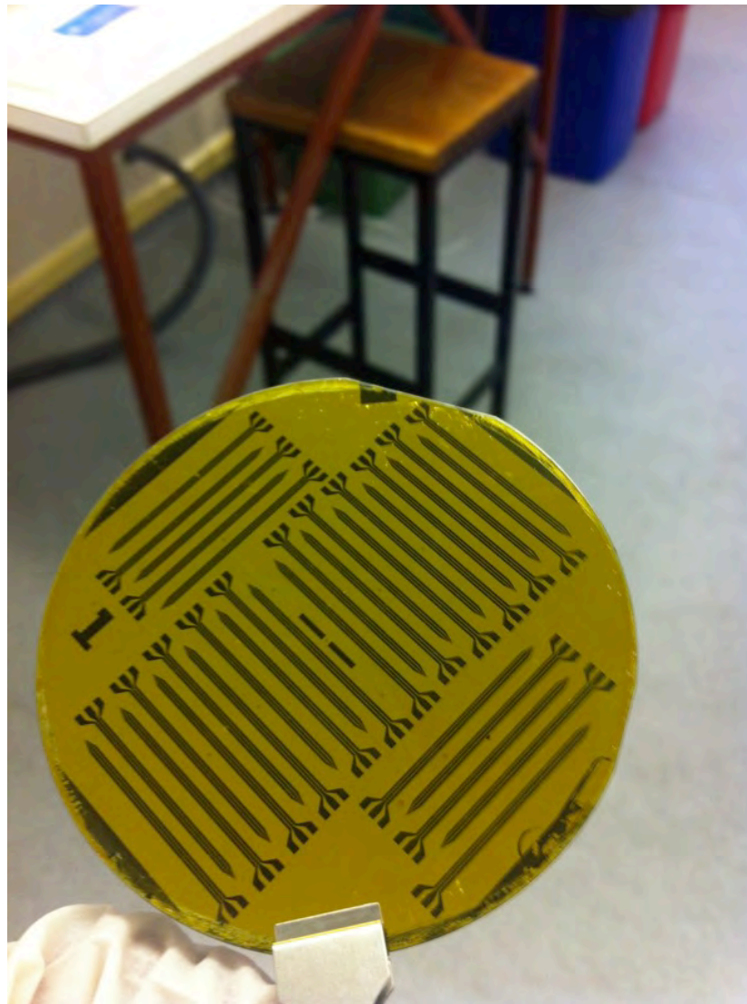
Figure 2.15. Polyimide based sinusoidal probes. Wafer diameter is 3 inches. Fabrication using polyimide was stopped due to the complexities in obtaining conformal and bubble free layers. This may have been related to the plastic pipette deposition used before the polyimide spin process.
