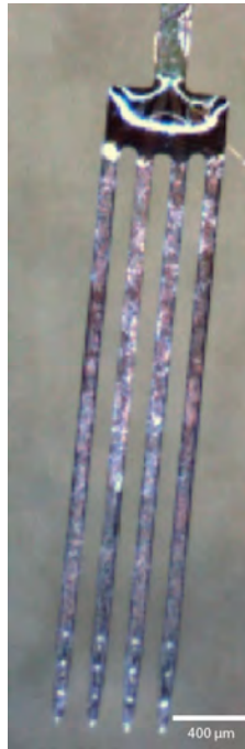
Figure 1.9. The Michigan probe electrode consists of a substrate material of silicon with silicon dioxide/nitride insulation with 16 iridium-recording sites linearly arranged on the end of four shanks to allow for recordings from different layers of specific brain regions. Shank length= 3 mm. Probe thickness= 15 \mu\text{m} . Site area= 1250 \mu\text{m}^2 (Ward et al., 2009). Recently, it is possible to obtain customised probes from the michigan probe spin-off company (NeuroNexus,USA), where multi-depth recording sites can be arranged in a circular format to allow for better isolation of neuronal activity ( www.neuronexus.com ). Further, customisable probes are now available with up to 128 recording sites.
