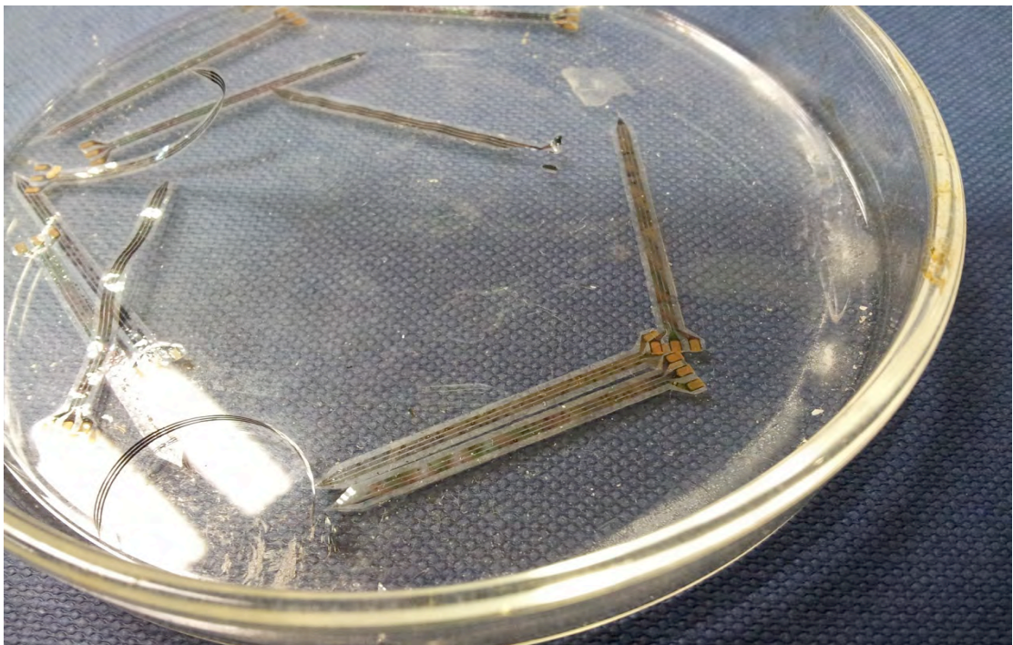
Figure 3.6. Bondpad decolourisation and etching of WTi due to more concentrated HF used to etch the titanium mask, post-parylene-C etching
