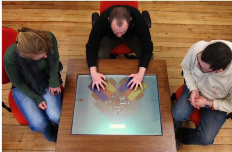
Figure 29: The custom-built FTIR table used for the evaluation (49x95x105cm) and the user study context.
