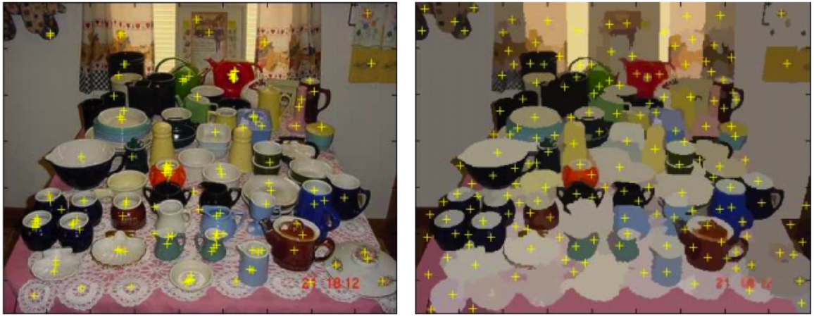
Figure 12: Dirik et al. [33] used image processing techniques such as corner detection to predict likely sequences of Passpoints graphical passwords. (left) an overlay of click points collected from a corpus of users; (right) overlay of click points predicted using their image processing methods.
