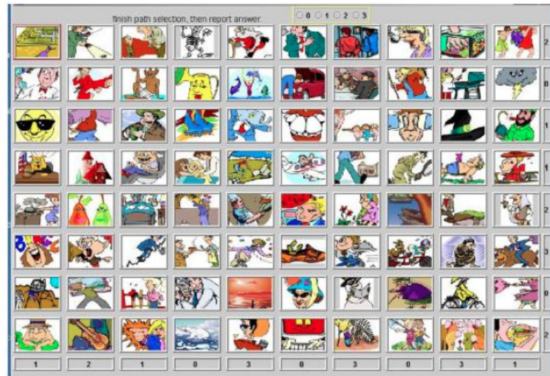
Figure 11: The cued-recall graphical password scheme proposed by Weinshall [139]. Users begin in the top left corner, and traverse the grid by moving down if they see a key image, or right otherwise. The user must then enter the number they arrive to at the edge of the grid.
