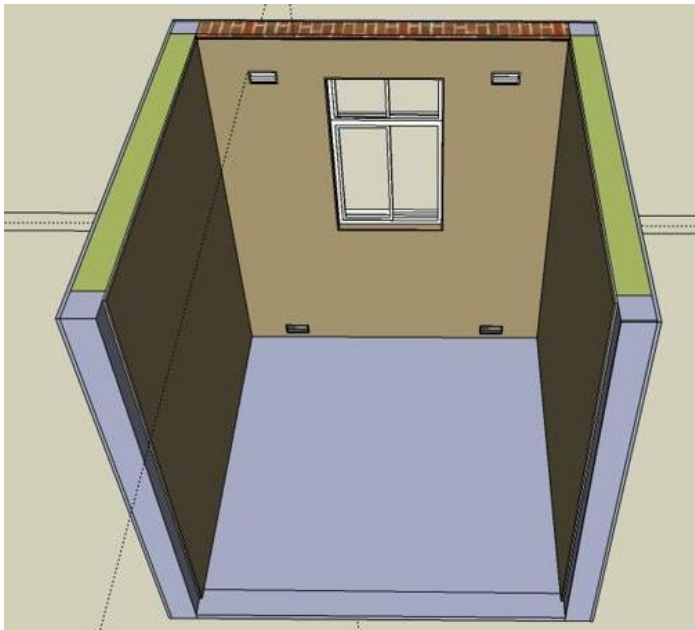
Figure 2-7 Walling system - wallboard finishing (Isa et al. , 2010)
