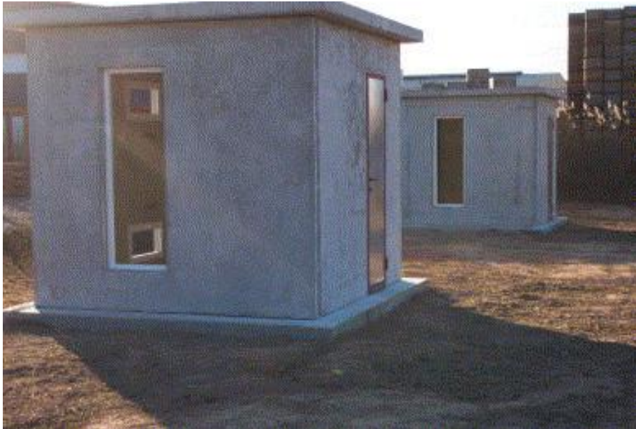
Figure 2-13 Cubicles testing Mopcon concrete
