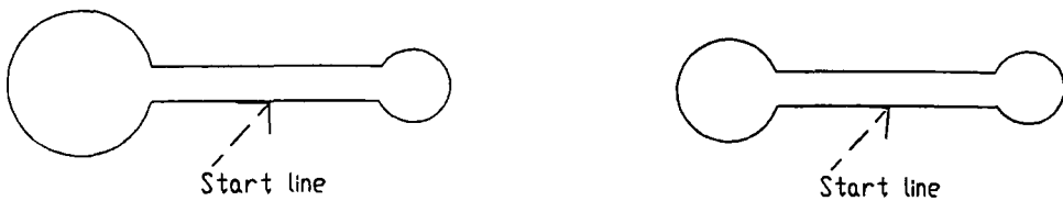
Fig 3.14 An example where use of chord length (the straight-line distance between start and end points) rather than segment length as prime discriminator between possible start lines makes choice of start line and start direction less sensitive to small changes in object shape.
