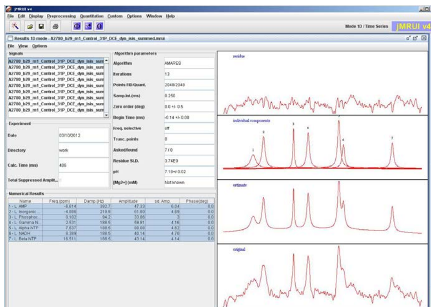
Figure 2.12: An example of the jMRUI user interface for one A2780 tumour AMARES final results. On the right hand side is, from bottom to top, the original spectrum, the estimated spectrum, the individual components of the spectrum and the residue of the estimation. On the left hand side are the numerical results including the amplitude and standard deviation of each peak.
