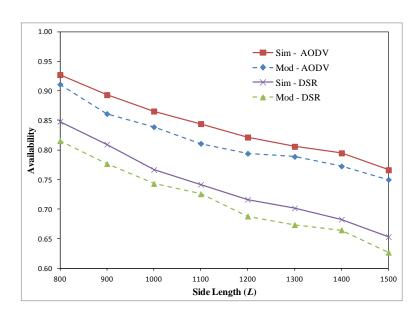
Figure 5.8: Path connection availability versus the side length of the network area, where R = 250 m, N = 100,  $\lambda = 10$  Kbps and routing protocol is AODV or DSR
