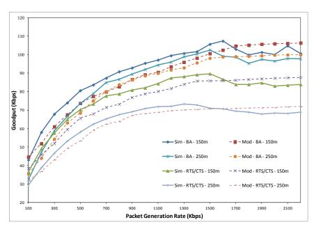
Figure 6.17: Goodput versus packet generation rate for the BA and RTS/CTS methods, in the case of packet size = 2 kB,  $R_{cs} = 250$  m, L = 800 m, and R = 150 or 250 m
