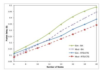
Figure 3.11: Packet delay versus number of nodes for both BA and RTS/CTS methods, in the case of  $\lambda = 2$  Mbps,  $N_h = 2$ , Packet Size = 2 KB,  $\lambda_h = 10$  Kbps
