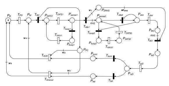
Figure 3.5: One node detailed model for the BA method
