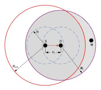
Figure 1.5: Single hop communication illustrating interfering and hidden nodes
