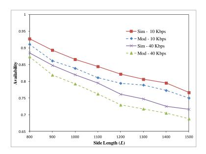
Figure 5.6: Path connection availability versus the side length of the network area, where R = 250 m, N = 100, and  $\lambda = 10$  or 40 kbps
