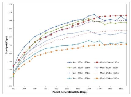
Figure 6.15: Goodput versus packet generation rate for the BA method, in the case of packet size = 2 kB,  $R_{cs}$  = 250 or 350 m, L = 800 m, and R = 150 or 250 m
