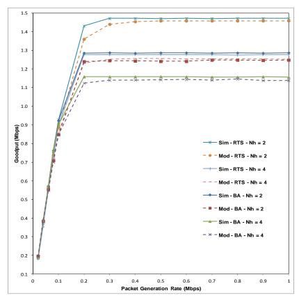
Figure 3.10: Goodput versus packet generation rate for the BA and RTS/CTS methods, in the case of N = 10,  $N_h = 2$  and 4, Packet Size = 2 KB,  $\lambda_h = 100$  Kbps
