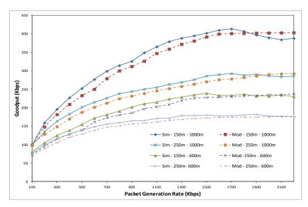
Figure 6.13: Goodput versus packet generation rate for the RTS/CTS method, in the case of packet size = 6kB,  $R_{cs}$  = 150m or 250, L = 600m or 1000m, and R = 150m
