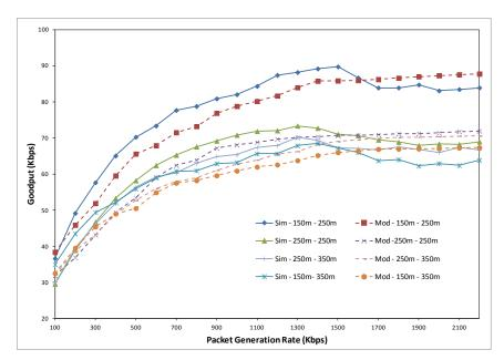
Figure 6.16: Goodput versus packet generation rate for the RTS/CTS method, in the case of packet size = 2 kB,  $R_{cs} = 250 \text{ or } 350 \text{ m}$ , L = 800 m, and R = 150 or 250 m
