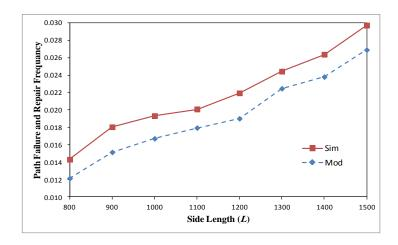
Figure 5.9: Path failure and repair frequency versus the side length of the network area, where R = 250 m, N = 100, and  $\lambda = 10$  Kbs.
