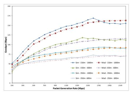
Figure 6.12: Goodput versus packet generation rate for the BA method, in the case of packet size = 2 kB,  $R_{cs}$  = 150 or 350 m, L = 600 or 1000 m, and R = 150 m
