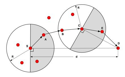
Figure 4.2: Packet forwarding in a multi-hop path
