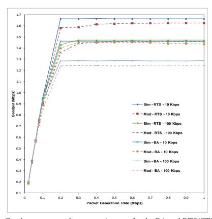
Figure 3.9: Goodput versus packet generation rate for the BA and RTS/CTS methods, in the case of N = 10,  $N_h = 2$ , Packet Size = 2 KB,  $\lambda_h = 10$  and 100 Kbps
