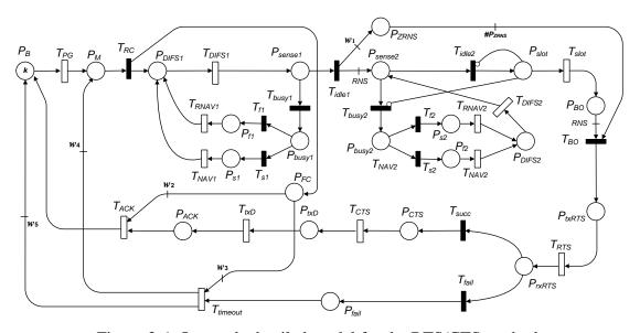
Figure 3.6: One node detailed model for the RTS/CTS method
