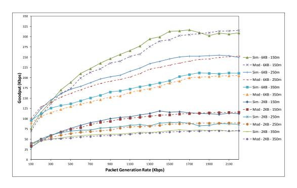
Figure 6.8: Goodput versus packet generation rate for the BA method, in the case of packet size = 2 or 6 kB,  $R_{cs}$  = 150, 250 or 350 m, L = 600 m, and R = 150 m
