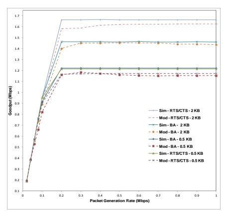
Figure 3.12: Goodput versus packet generation rate for the BA and RTS/CTS methods, in the case of N = 10,  $N_h = 2$ , Packet Size = 2 and 0.5 KB,  $\lambda_h = 10$  Kbps
