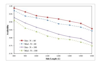
Figure 5.5: Path connection availability versus the side length of the network area, where R = 250 m, N = 60 or 100, and  $\lambda = 10$  kbps
