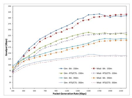
Figure 6.11: Goodput versus packet generation rate for the BA and RTS/CTS methods, in the case of packet size = 6 kB,  $R_{cs}$  = 150 or 350 m, L = 600 m, and R = 150 m
