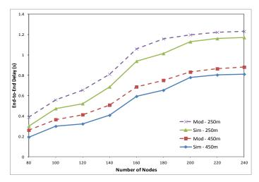
Figure 6.18: End-to-end delay versus number of nodes for the BA method, in the case of packet size = 2 kB,  $R_{cs}$  = 250 or 450 m, L = 1200 m, and R = 250 m
