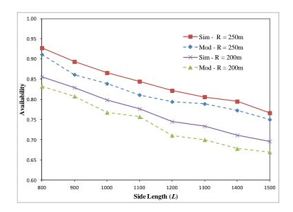
Figure 5.7: Path connection availability versus the side length of the network area, where R = 250 or 200 m, N = 100, and  $\lambda = 10$  kbps.
