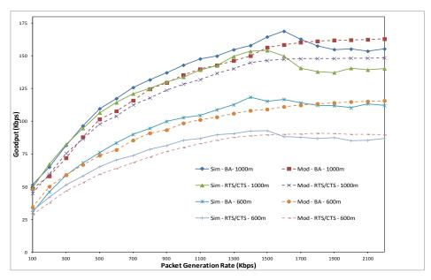
Figure 6.14: Goodput versus packet generation rate for the BA and RTS/CTS methods, in the case of packet size = 2 kB,  $R_{cs}$  = 150 m, L = 600 or 1000 m, and R = 150 m
