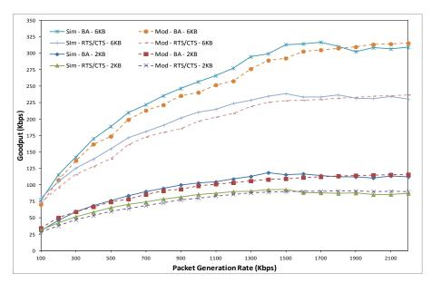
Figure 6.10: Goodput versus packet generation rate for the BA and RTS/CTS methods, in the case of packet size = 2 or 6 kB,  $R_{cs}$  = 150 m, L = 600 m, and R = 150 m
