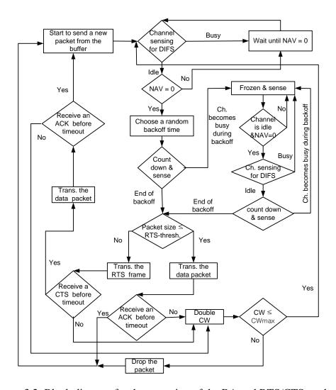
Figure 3.2: Block diagram for the operation of the BA and RTS/CTS methods
