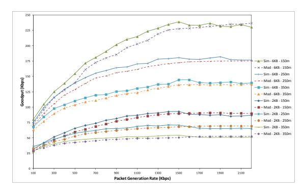
Figure 6.9: Goodput versus packet generation rate for the RTS/CTS method, in the case of packet size = 2 kB or 6 kB,  $R_{cs}$  = 150, 250 or 350 m, L = 600 m, and R = 150 m
