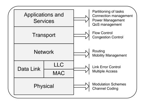
Figure 1.4: Protocol stack of wireless networks and corresponding main functions
