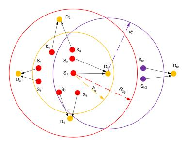
Figure 3.4: The Network architecture for a single hop ad hoc network with hidden nodes
