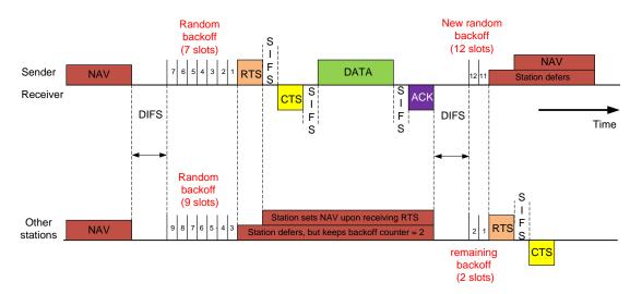
Figure 3.3: Timing diagram for the operation of the RTS/CTS method
