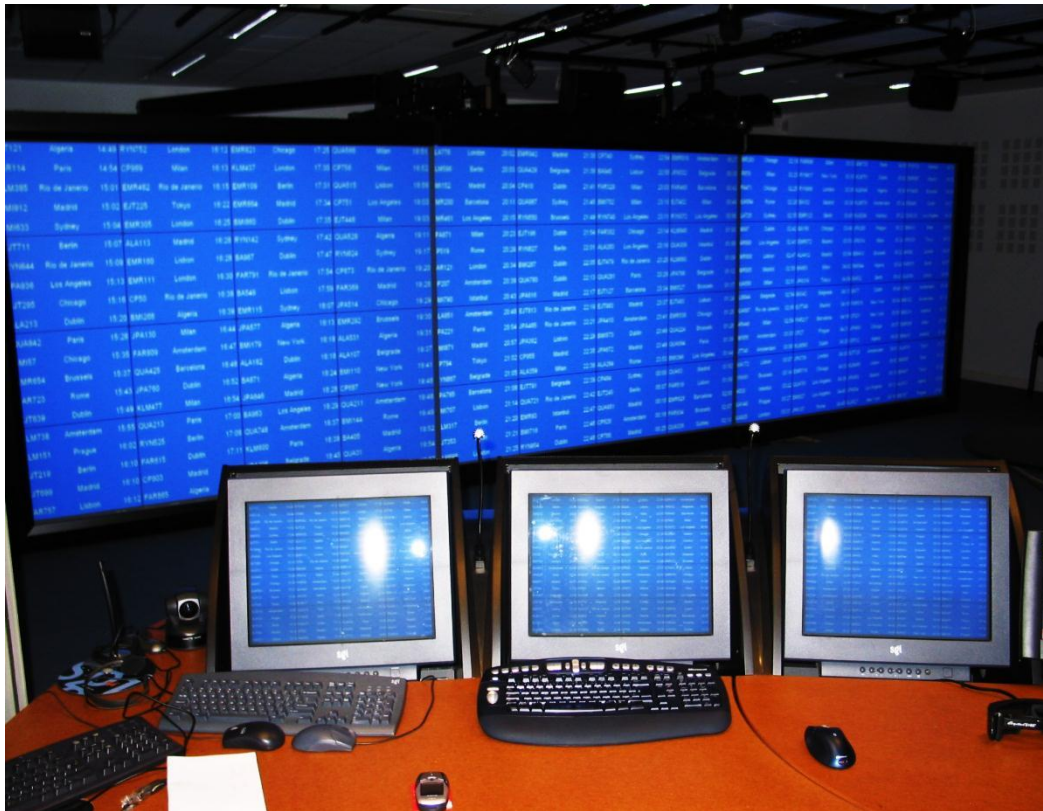
Figure 8.7 Display setup, using a 3-screen CAVE in a “wall” arrangement.
