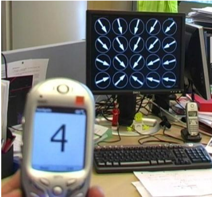
Figure 4.14 An informal pilot study of CROSSFLOW using a desktop PC monitor as a public display and a SPV E200 smartphone as a personal display.
