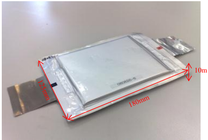
Figure 2-2 - Pouch cell packaging of JS micro Li-ion capacitor
