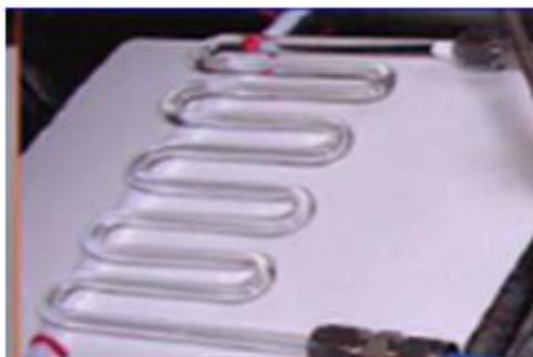
Figure 2.9: Glass narrow channel reactor made of made of borosilicate with internal diameter of 1.5 mm (Jachuck and Nekkanti, 2008)
