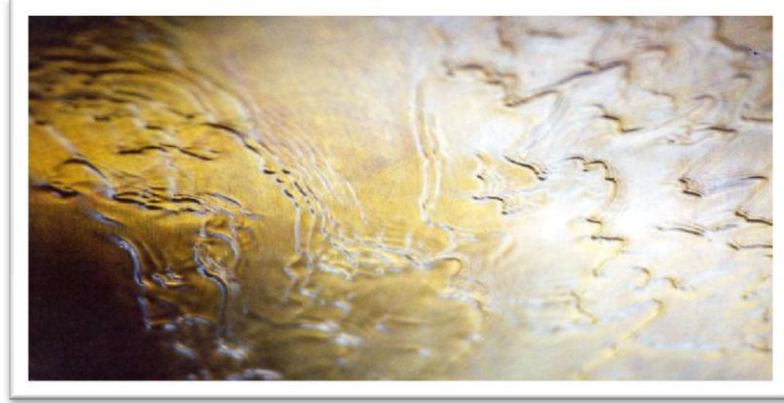
Figure 2.4: Thin film flows on smooth disc (adopted from (Vicevic, 2004))
