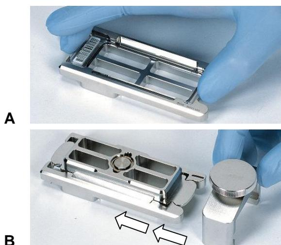
**Figure 2.4** – CGH oligo array, chamber and clamp assembly
