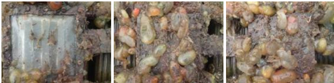
Figure 44. Panels after 6 month static water immersion trial in Hartlepool Marina. From left to right: Silicone membrane and CO 2 panels, PVC panels, and silicone membrane panels. All panels are 10 x 10 cm square.
