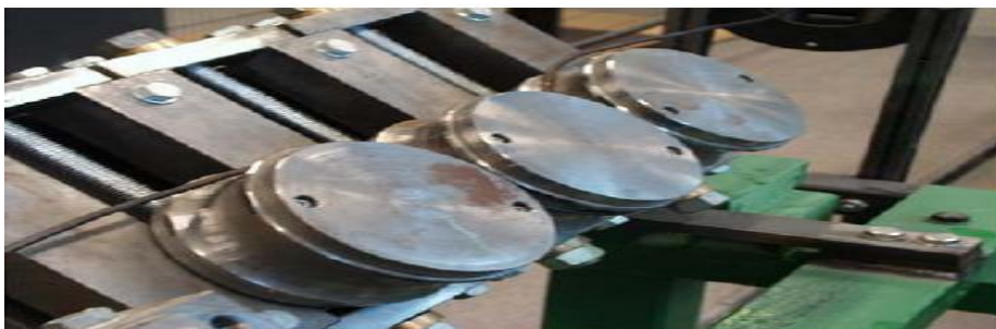
Figure 4.13: Reverse bending equipment with three steel rollers (Gillström and Jarl, 2006).
