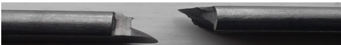
(e) Fractured specimen with 2mmx2mm channel cut from laboratory tensile testing
