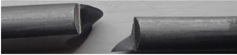
Figure 8.6: Fractured specimen from laboratory tensile testing of specimen with 1mm deep V-shaped cut.
