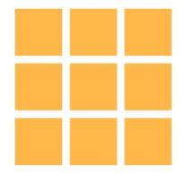
Figure 6.12: Square mask design for AlN MIM capacitors
