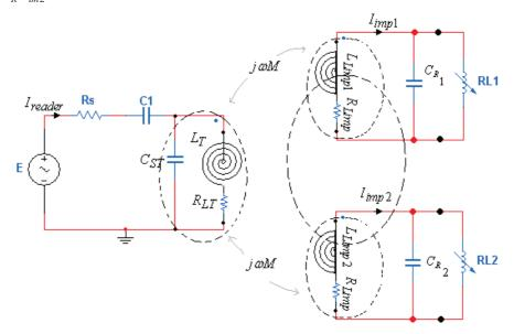
Figure (3.23) Lumped equivalent circuit with dual for inductive coupling module
