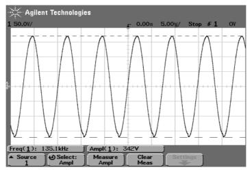
Figure (3.42) the output voltage of Class-E power amplifier
