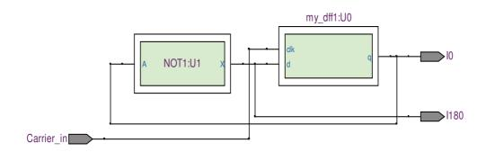
Figure (B1.6) the carrier simulation for generates (0,180)
