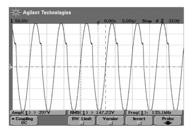
Figure (3.43) the output voltage of Class-F power amplifier at reader coil (Tx RF signal)
