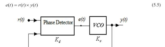
Figure (5.22) the feedback control method using PLL
