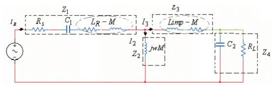
Figure (3.7) the equivalent circuit can be simplified as shown
