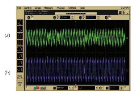
Figure (5.32) the TX and RX for QPSK signal generated by VHDL Code (a) RX-QPSK signal, (b) TX QPSK signal
