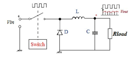
Figure (3.66) the principle of switch regulator circuit
