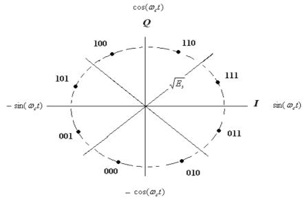
Figure (2.19) the constellation diagram for 8-PSK
