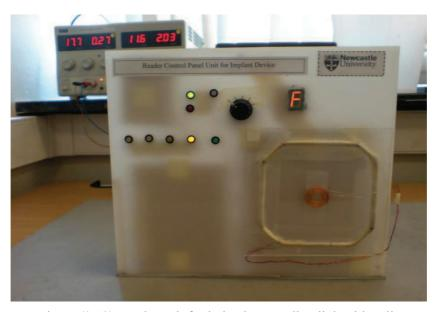
Figure (3.12) Reader unit for inductive coupling link with coils
