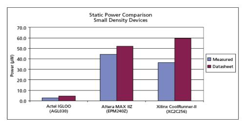
Figure (4.2) comparison of static power for FPGA and CPLD [198]
