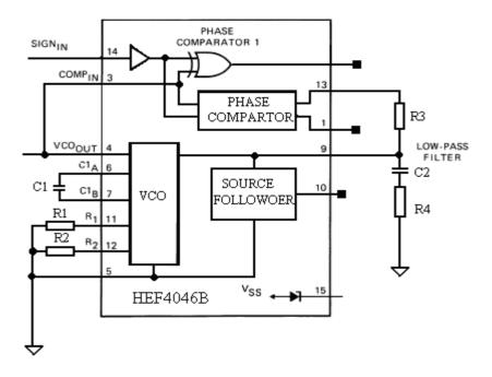
Figure (5.24) Detailed PLL HEF4046B control system
