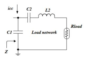
Figure (3.33) the load network circuit of Class-E PA
