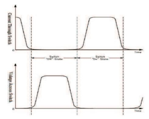
Figure (3.32) waveforms of the voltage and current switch conditions [145]
