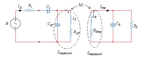
Figure (3.3) the modified circuit where ( $C_R = C_{simp} + C_2$ )
