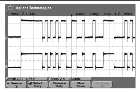
Figure (5.5) Tx PN data (a), (b) Demodulated data output
