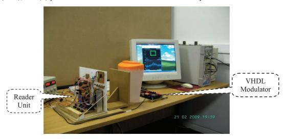
Figure (4.45) The Lab measurement for QPSK VHDL modulator over Inductive coupling link With Agilent, demodulator (E8408A)
