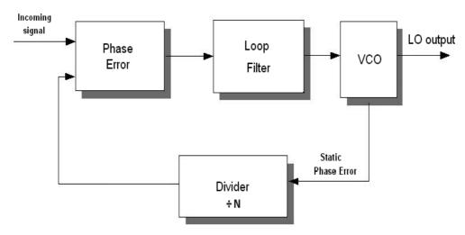
Figure (2.24) the principle architecture for PLL diagram [220]
