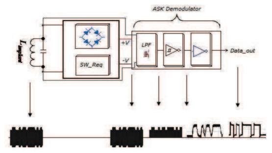
Fig (5.16) the ASK Demodulator used at the implant device
