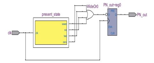
Figure (5.12) the PN sequence generated by VHDL code (A)
