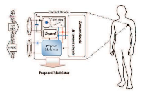
Figure (5.14) the target proposed modulator at implant device
