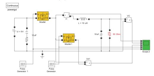
Figure (3.70) Simulation of the DC-DC converter block diagram
