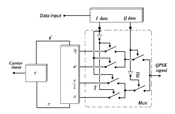
Figure (4.18) the concept (B) for generating Direct QPSK digital modulator
