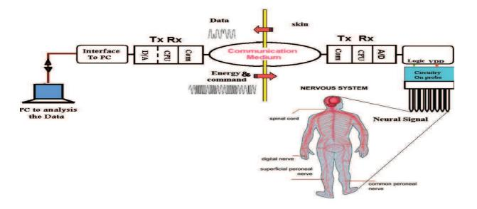
Figure (1.2) the bio-communications system architecture
