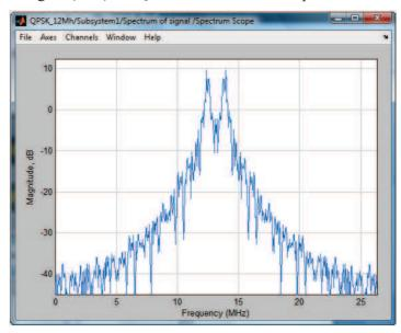
Figure (4.22) the spectrum of QPSK transmission and receipt of signal at Data rate 2Mbps, carrier 12.5MHz
