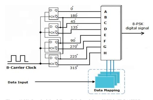
Figure (4.33) the principle of direct digital modulator 8PSK in FPGA/CPLD
