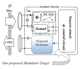
Figure (2.39) the proposed modulator target design inside the implant device
