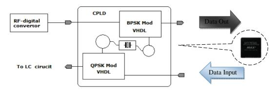
Figure (C1.2) the proposed full digital modulators at the implant device
