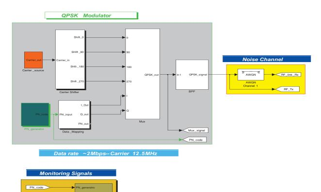
Figure (4.20) the simulation environment in MATLAB/Simulink for the proposed QSPK digital modulator
