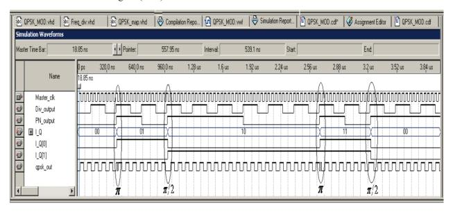
Figure (4.25) the simulation waveforms of VHDL QPSK modulator
