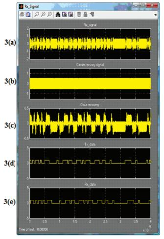
Figure (4.12) the proposed digital BPSK Mod/ Demodulator in MATLAB/Simulink
