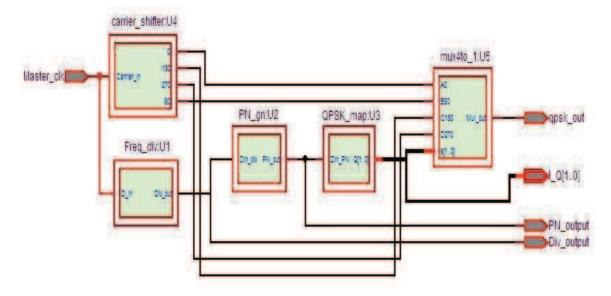
Figure (4.24) the behavioral VHDL modulator simulation
