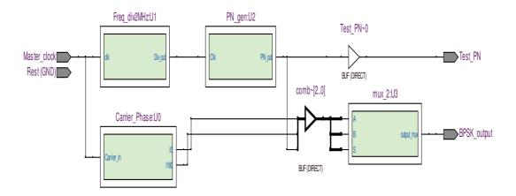
Figure (B1.5) the block diagram of the behavioral BPSK modulator
