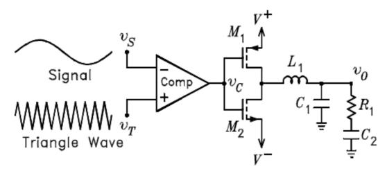
Figure (3.30) illustrating the principle of Class D power amplifier
