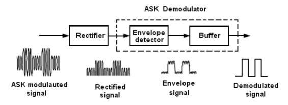
Figure (2.8) the block diagram of ASK demodulator [57]
