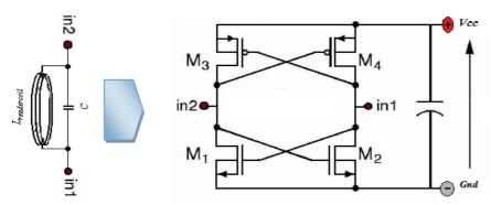
Figure (3.60) the RF-DC CMOS Bridge rectifier circuit
