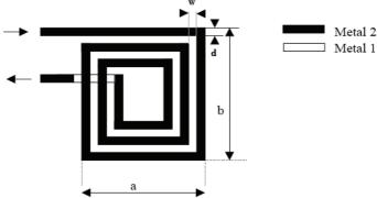
Figure (C1.8) the geometry of a typical rectangular spiral coil
