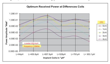
Figure (3.18) the best receiving power over different reader coils
