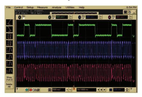
Figure (4.60) the output of the VHDL QPSK modulator filtered the QPSK TX signal by LPF
