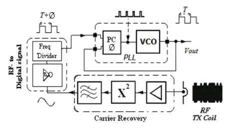
Figure (5.21) the first control method using PLL (HEF4046)
