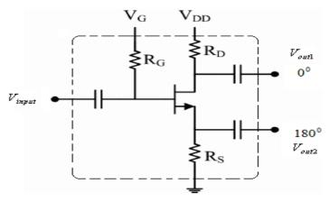
Figure (2.32) the single FET phase shifter circuit
