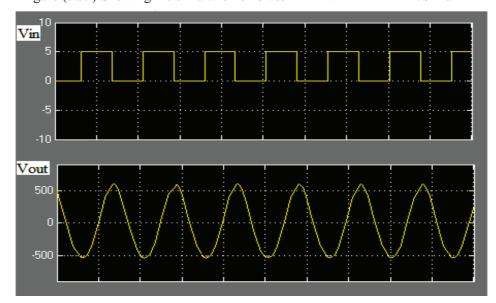
Figure (3.40) showing the simulation result waveform of Class F –PA at Frequency 135 kHz
