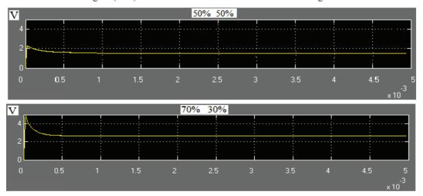
Figure (3.71) Simulation waveform of the DC-DC converter according to duty cycle
