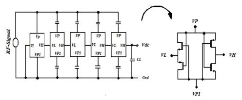
Figure (3.58) the bridge voltage multiplier cells circuit [151]
