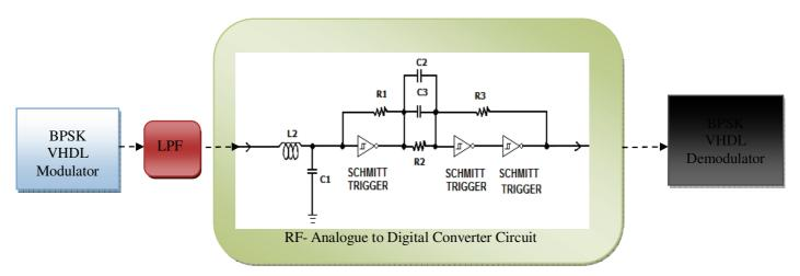
Figure (C1.3) illustrated the second proposed RF-digital circuit converter
