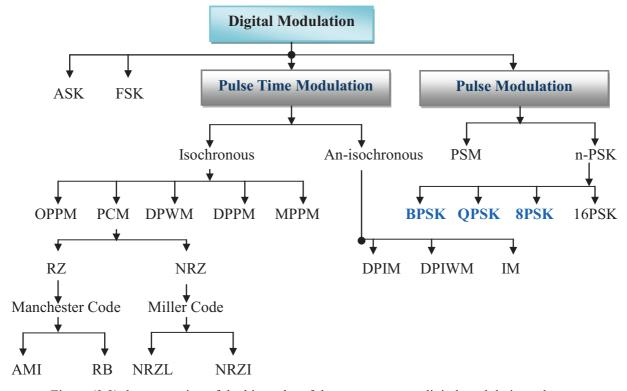
Figure (2.2) demonstration of the hierarchy of the most common digital modulation schemes
