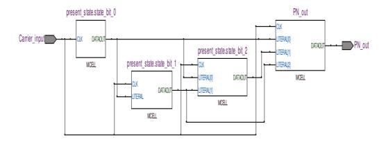
Figure (B1.19) the block diagram of the Behavioral the PN- code generator
