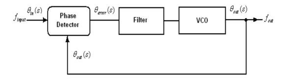
Figure (5.23) the PLL feedback system
