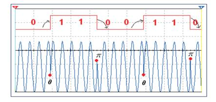
Figure (2.10) the BPSK waveform with respect to binary state
