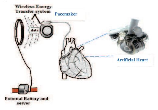
Figure (1.6) the wireless communication for artificial pacemaker device
