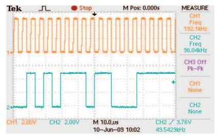
Figure (C1.1) the PN sequence waveform output (CH2)
