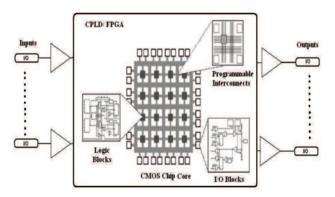
Figure (4.4) power component of typical CPLD/FPGA devices [198]
