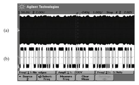
Figure (5.30) (a) the TX-RF ASK transmitted by Class E-PA and (b) controlled PN-signal
