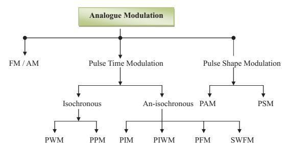
Figure (2.1) demonstration of the hierarchy of analogue modulations
