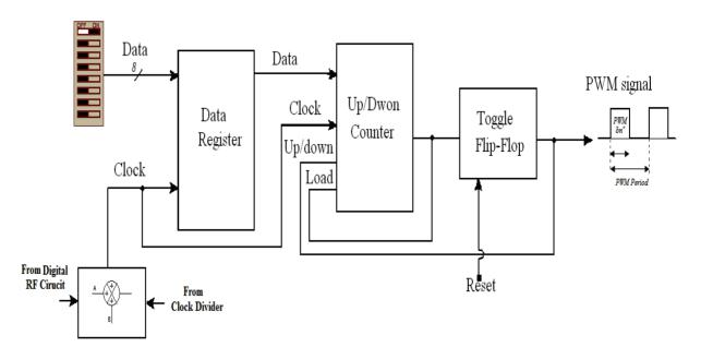
Figure (5.28) the second control method using PWM code by VHDL
