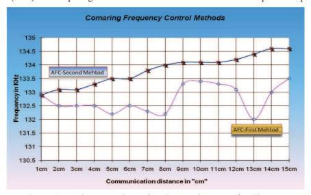
Figure (3.47) the comparison of AFC control systems for Class PA
