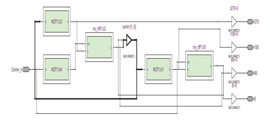
Figure (4.27) Behavioral VHDL Simulation for carrier phase shifter
