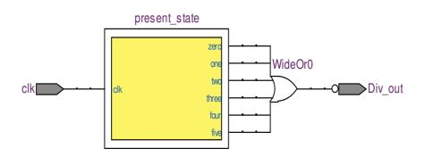
Figure (B1.8) the simulation behavioral of frequency divider
