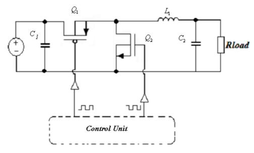
Figure (3.64) the circuit of **dc-dc** charging pump [181]
