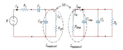
Figure (3.2) the basic lumped equivalent inductive coupling circuit
