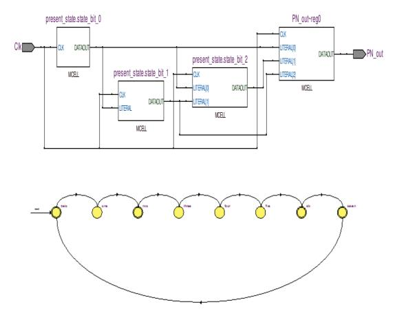
Figure (B1.9) the simulation behavioral of the PN sequence code and the states
