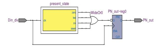
Figure (B1.16) the simulation behavioral of the PN -code sequence generator
