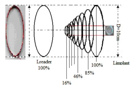
Figure (3.15) the comparison of coupling coefficient between the implant and reader coils
