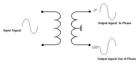
Figure (2.28) the diagram of a simple balun using a transformer tap centre
