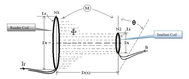
Figure (3.13) the geometry for inductive coupling and orientation between two coils
