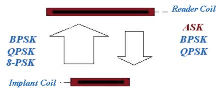
Figure (3.77) Proposed digital schemes over inductive link system
