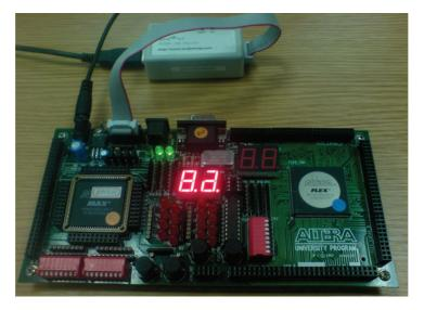
Figure (B1.0) the Altera development board FPGA/CPLD
