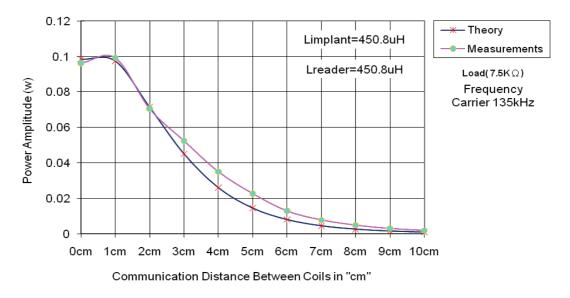
Figure (3.10) the optimum received power for the choice of coil at reader and implant
