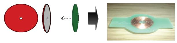
Figure (A1.7) The spiral coil design for implant in our work, 30mm diameter for the Rx- wireless received power
