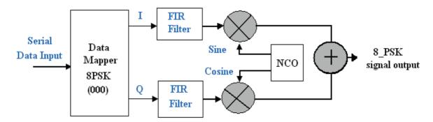
Figure (4.31) the diagram for 8psk modulator
