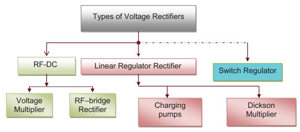
Figure (3.55) illustrates the different types of power rectifying topologies applied for biomedical device
