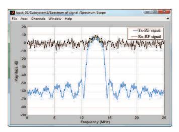
Figure (4.11) The Spectrum of BPSK transmits Receives signals at carrier 12.5MHz
