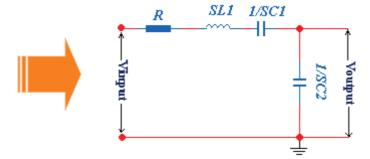
Figure (4.52) the second-order for LPF filter circuit
