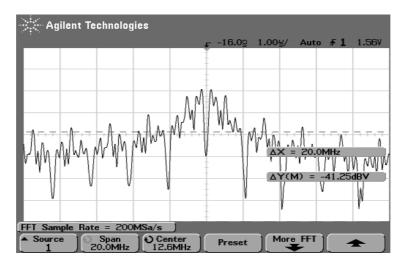
Figure (4.39) The Spectrum of BPSK transmitted signal at carrier 12.5MHz
