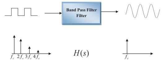
Figure (4.55) The BPF principle for attenuation of the harmonics
