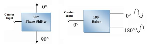
Figure (2.27) the balun phase shifters block diagrams
