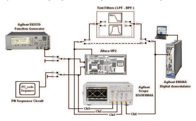
Figure (4.58) LAB measurment for filters (LPF,BPF) for TX-QPSK digital signal
