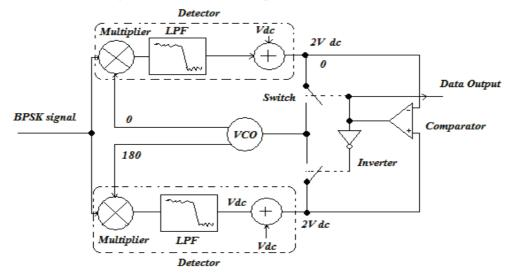
Figure (2.13) the Anti-parallel synchronization loop demodulator for BPSK
