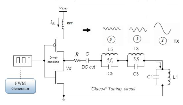
Figure (3.34) the principle components of Class F amplifier circuit
