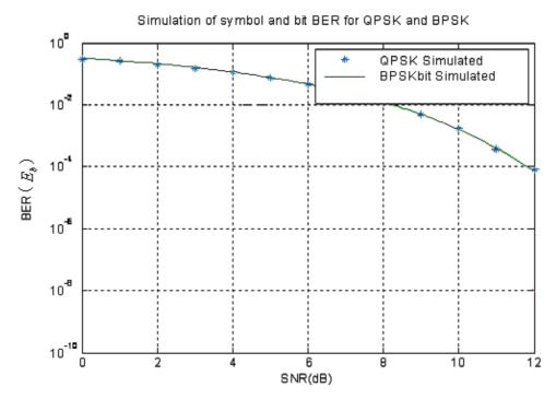
Figure (2.21) Simulation for the BER comparing between BPSK and QPSK
