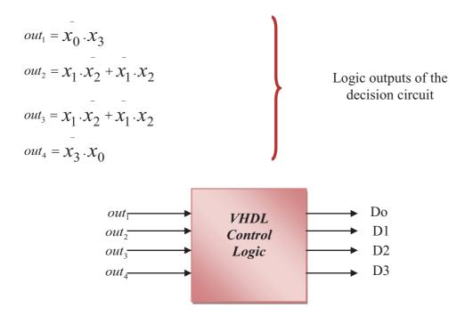
Figure (5.9) the Inputs/Outputs implemented with CPLD
