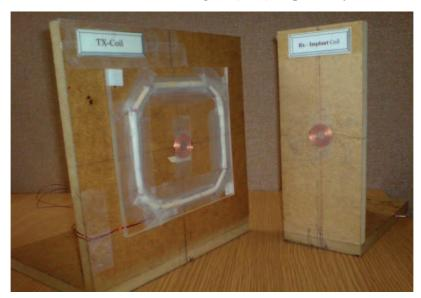
Figure (3.11) Fabricated transmitter and receiver coils
