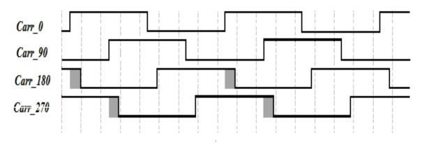
Figure (4.28) the waveforms delay in carrier phase shifters
