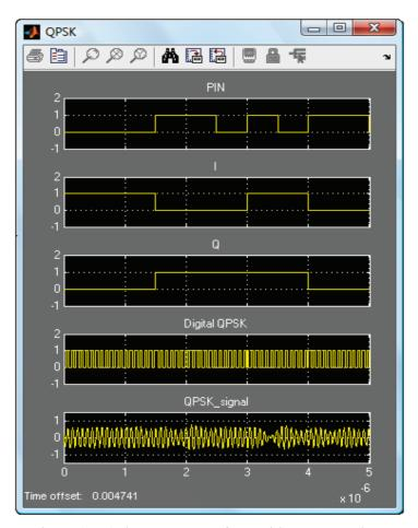
Figure (4.21) the QPSK waveform with respect to data state
