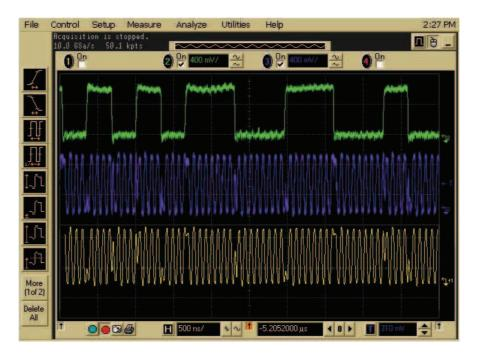
Figure (4.59) the output of VHDL BPSK modulator (Digital signal) and filtered signal at 12.5 MHz
