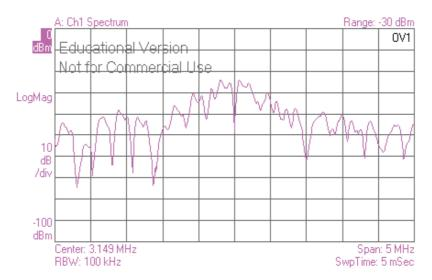
Figure (4.47) The TX Spectrum of the 8PSK transmitted Signal at carrier 12.50MHz and data 2MBps
