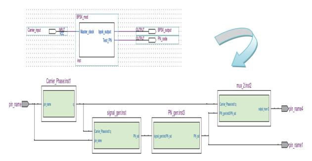
Figure (4.14) the proposed VHDL BPSK modulator
