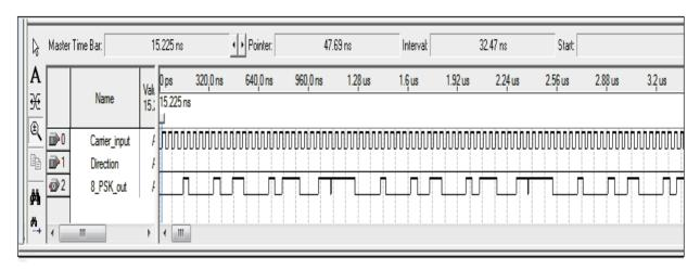
Figure (4.38) waveform simulation for 8PSK VHDL modulator
