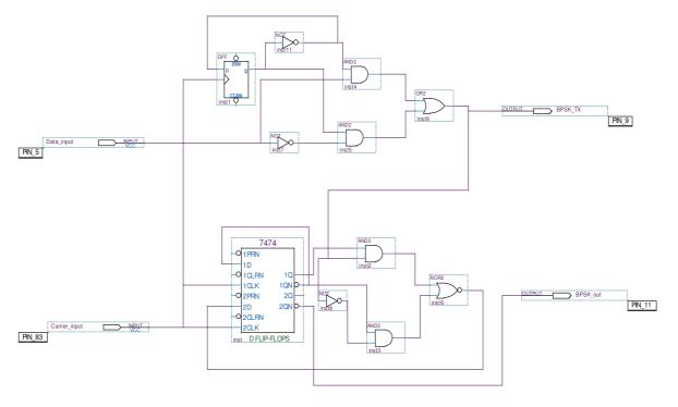
Figure (B1.4) the block diagram of the structural BPSK modulator Module (B)
