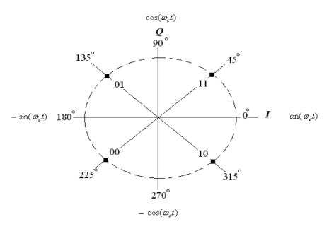
Figure (2.15) Constellation diagram of QPSK signal
