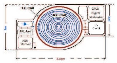
Figure (5.15) the general layout diagram for the implant device
