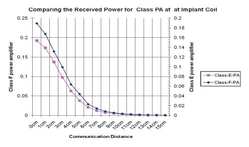
Figure (3.46) the comparing of received Power between Class E and F power amplifiers
