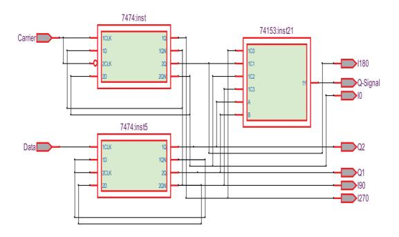
Figure (4.23) Structural VHDL-code simulation for the QPSK modulator
