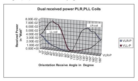
Figure (3.25) the RF inductive coupling Lab test for dual coils
