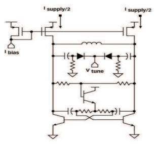
Figure (2.25) the LC-VCO principle of circuit diagram
