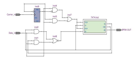
Figure (B1.3) the VHDL of the structural BPSK modulator module (A)
