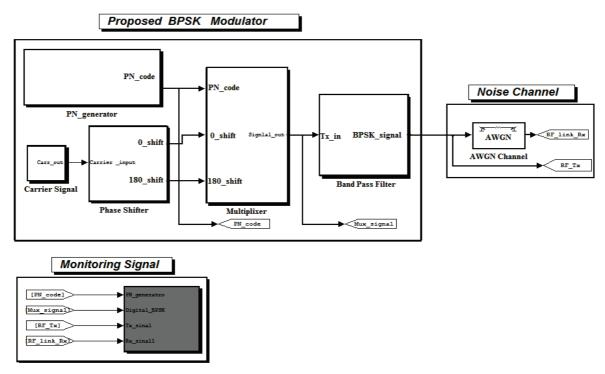
Figure (4.10) the simulation environment with MATLAB/Simulink for proposed BPSK modulator
