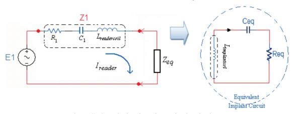
Figure (3.5) Equivalent impedance circuit at load part
