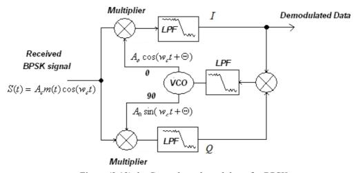
Figure (2.12) the Costas loop demodulator for BPSK
