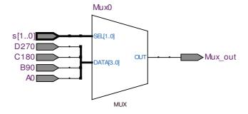
Figure (B1.14) the simulation behavioral of multiplexer (4 to 1)
