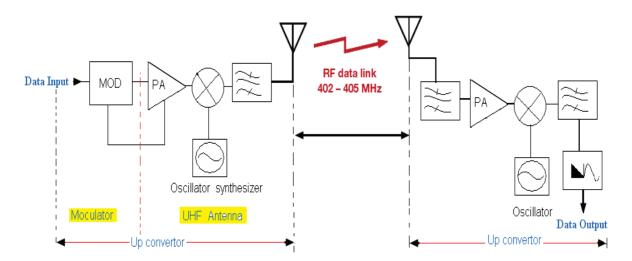
Figure (C1.6) the transceiver solution with UHF solution
