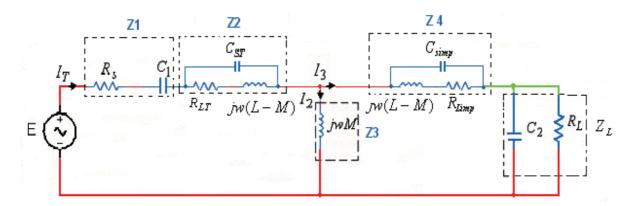
Figure (3.78) the equivalent coupling circuit
