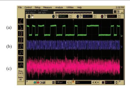
Figure (5.31) TX and RX for BPSK signal generated by VHDL code: (a) PN-sequence Code, (b) Tx- BPSK signal,(c) RX-BPSK signal
