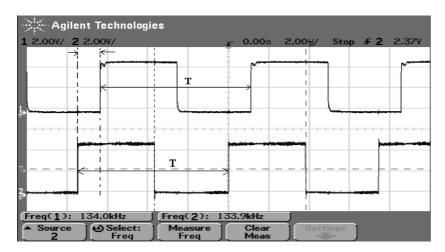
Figure (5.27) Phase error between original and converted digital signal
