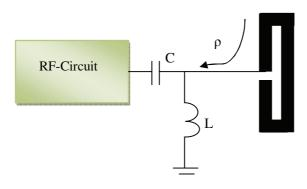
Figure (C1.13) Addition of Shunt capacitor for matching Antenna
