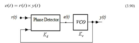
Figure (3.36) showing the analysis feedback signal for PLL -VCO
