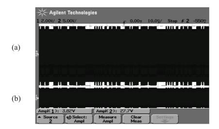
Figure (5.18) Waveforms of ASK RF Tx signal (a), (b) Rx-received signal at implant device at distance (5cm)
