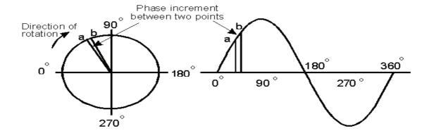
Figure (2.23) the Phase changing diagram
