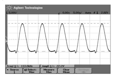
Figure (3.41) the switch (Transistor) voltage of the power amplifier
