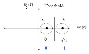
Figure (2.4) Constellation diagram of ASK signal
