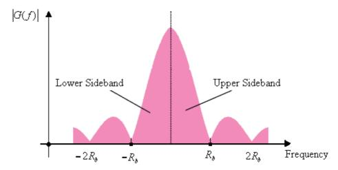
Figure (2.5) Spectrum of the ASK signal
