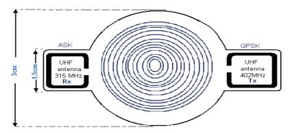
Figure (C1.11) the second proposed geometry of UHF antenna with power spiral coil
