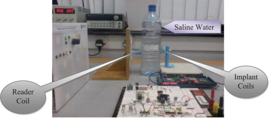
Figure (3.80) bench test measurements for the proposed VHDL Modulator over inductive coupling link
