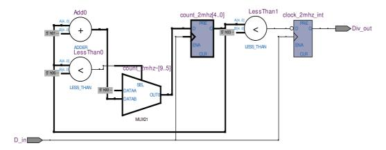
Figure (B1.15) the simulation behavioral for the frequency divider
