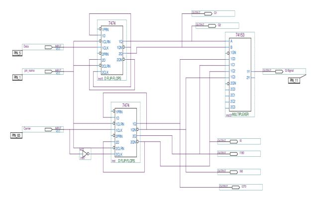
Figure (B1.11) the block diagram of the structural QPSK modulator
