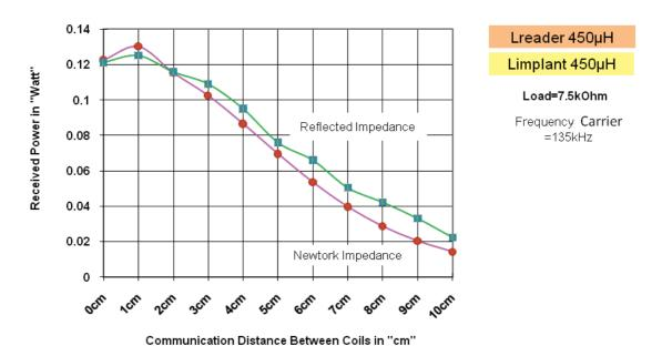
Figure (3.8) the MATLAB/ Simulation and measurement comparison for Optimum received Power with different methods
