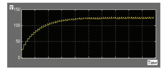
Figure (3.69) Simulation Result for voltage doubler output waveform
