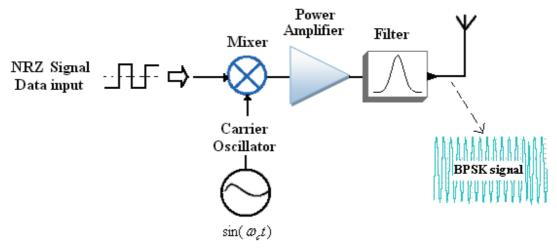
Figure (2.9) the block diagram of the BPSK modulator
