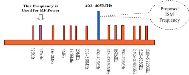
Figure (1.11) ISM frequency bands used for medical applications
