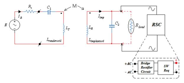
Figure (3.67) the switch regulator connected with the inductive coupling circuit
