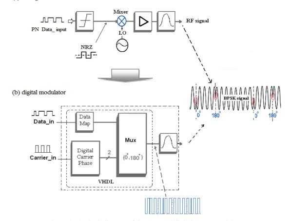
Figure (4.8) Block diagram of the proposed digital BPSK Modulator Compared to Analogue
