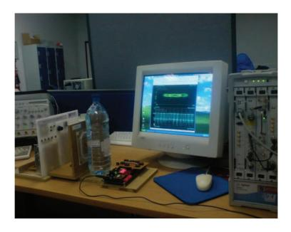
Figure (4.41) the preliminary lab measurements with (E8408AVXI) For the proposed BPSK VHDL modulator at over inductive link
