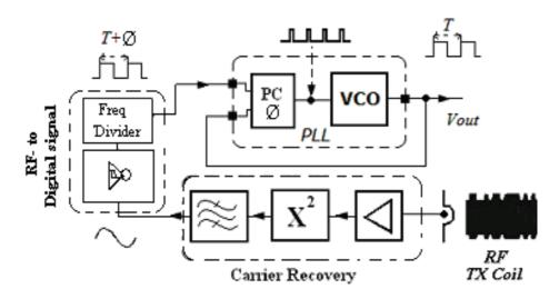
Figure (3.35) the proposed Feedback Control block diagram for Class-F- PA
