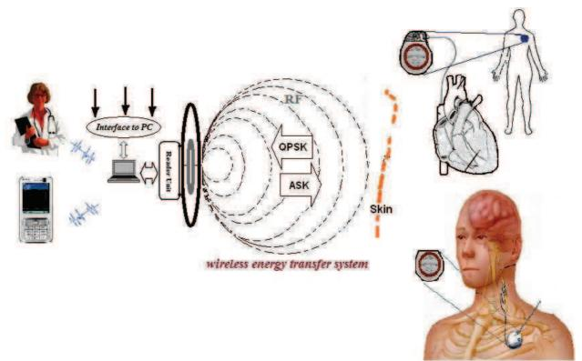
Figure (4.1) Proposed bioelectronics implant wireless interface system for pacemaker
