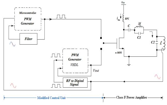
Figure (3.37) modified the block diagram of the Class-F- power amplifier
