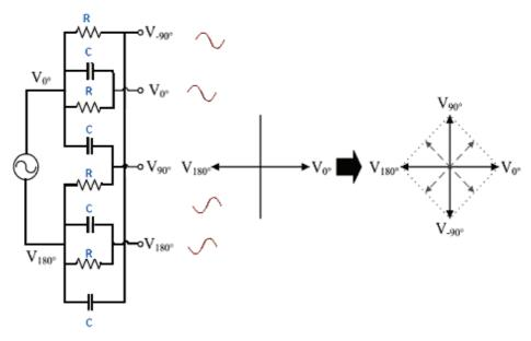
Figure (2.29) shows the RC-Polyphase network diagram
