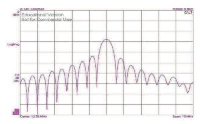
Figure (4.43) The TX Spectrum of the QPSK transmitted Signal at carrier 12.58MHz
