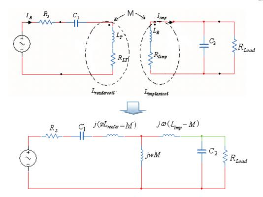
Figure (3.6) the inductive circuit converted to the equivalent circuit diagram
