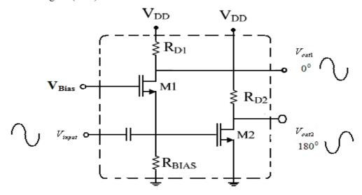
Figure (2.34) the CG-CS Active Balun FET phase shifter circuit
