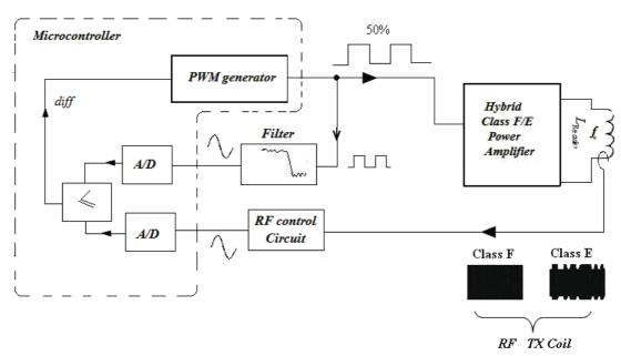
Figure (C1.17) Third method for frequency controller using microcontroller
