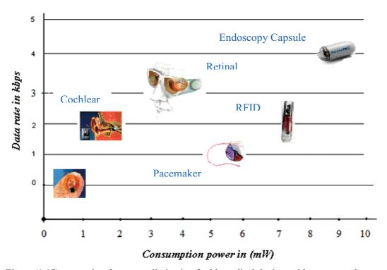
Figure (1.17) comparing the power dissipation for biomedical devices with respect to data rate
