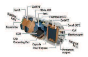
Figure (1.7) the Architecture of Endoscopy Capsule [203]
