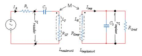
Figure (3.1) the basic lumped equivalent inductive coupling circuit
