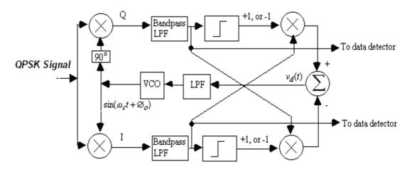
Figure (2.20) the block diagram of the QPSK demodulator
