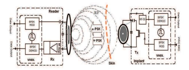
Figure (C1.15) the proposed completed block diagram of RF-digital convertor
