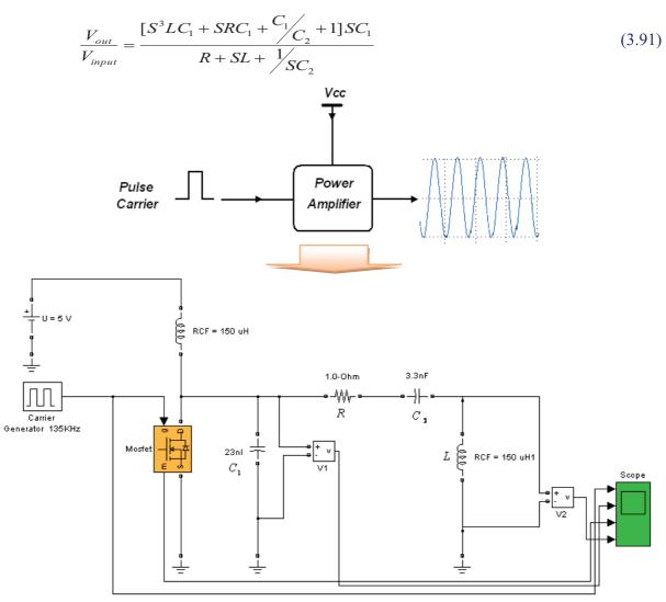
Figure (3.38) the simulation of Class-E- PA with MATLAB/Simulink
