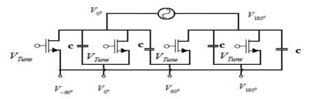
Figure (2.30) the RC-polyphase network diagram
