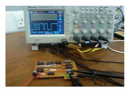
Figure (C1.0) shown the PN sequence generator circuit
