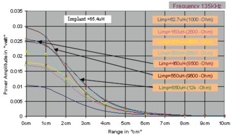
Figure (A1.5) Received Rx wireless power for the fixed implant Coil and changed the reader coil
