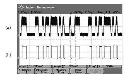
Figure (5.19) (a) LPF output demodulated signal (b) PN output data
