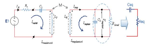
Figure (3.4) the lumped equivalent circuit for reflected impedance
