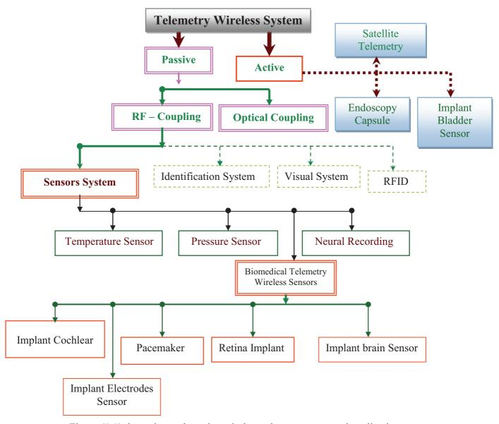
Figure (1.1) the active and passive wireless telemetry types and applications
