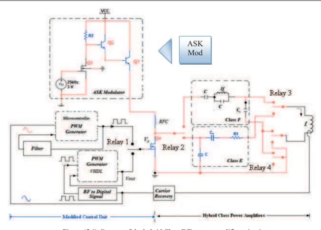
Figure (5.6) diagram of the hybrid Class E/F power amplifiers circuit
