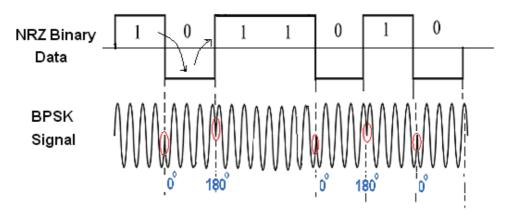
Figure (4.7) the BPSK waveform with respect to (NRZ) data state
