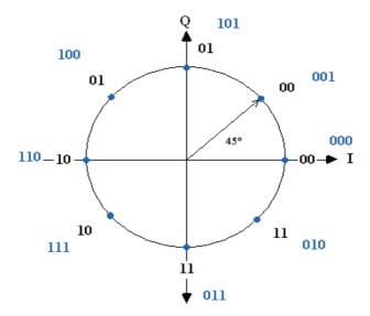
Figure (4.32) the constellation diagram of 8PSK modulator
