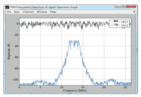
Figure (4.35) the spectrum of 8PSK transmission and receipt of signals at Data rate 2Mbps, carrier 12.5MHz
