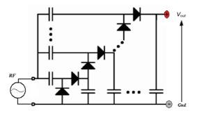
Figure (3.56) the voltage doubler circuit [153]
