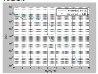
Figure (4.13) The BER simulation diagram of Demodulator signal from the proposed BPSK Modulator
