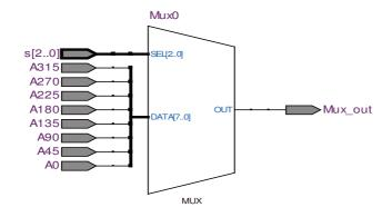
Figure (B1.21) the simulation behavioral of the multiplexer for (8 to 1)
