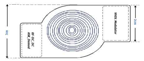
Figure (C1.12) the third proposed geometry of UHF antenna with power spiral coil
