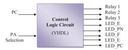
Figure (5.7) the Inputs/Outputs implemented with CPLD (EPM7128SL84-15)
