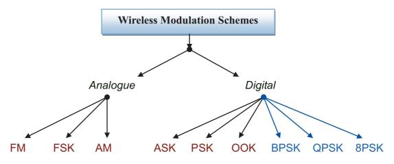
Figure (4.0) the most modulation schemes applied for biomedical devices
