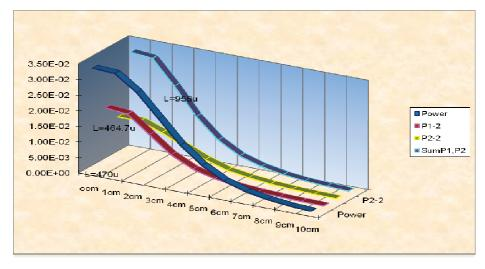
Figure (A1.9) the received power with two identical coils comparing to single coil
