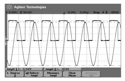
Figure (5.25) RF carrier signal (sine wave) and converted carrier digital signal
