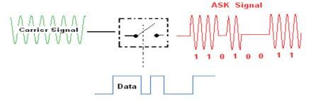
Figure (2.3) Principle of ASK modulation
