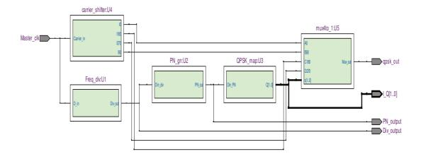
Figure (B1.12) the simulation behavioral for QPSK modulator
