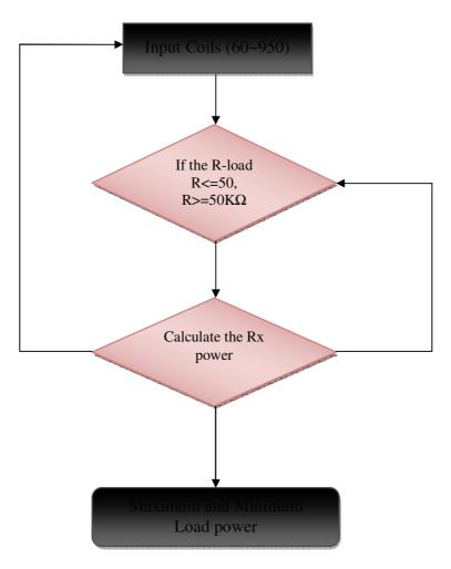
Figure (A1.1) flow chart to calculate the load power Compared to different Coils
