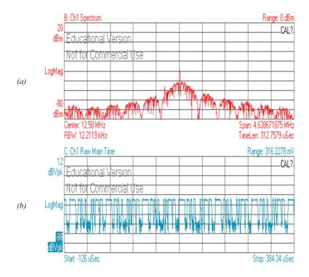
Figure (4.46) (a). The spectrum of Rx signal (b), demodulated data (3Mbps) Received from the proposed VHDL modulator at over inductive link
