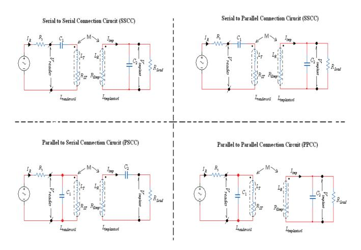
Figure (3.0) the four possible resonance circuits in inductive coupling
