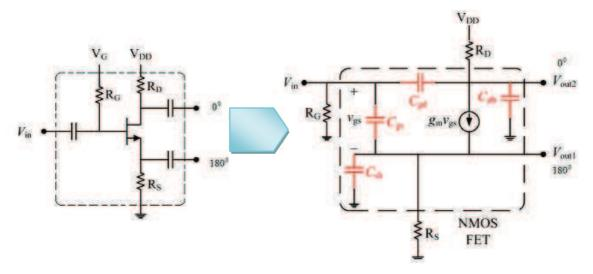
Figure (2.33) Single FET parasitic capacitance at high frequency
