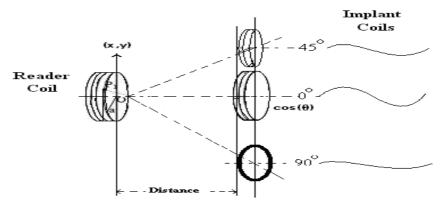
Figure (3.21) the misalignment analysis between two coils
