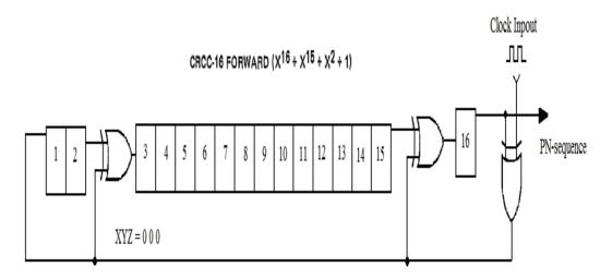
Figure (5.11) the technique for generates PN-sequence data [166]
