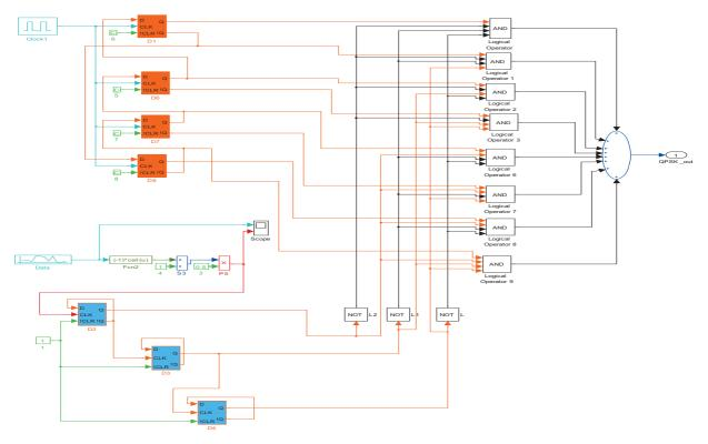
Figure (4.34) the simulation environment in MATLAB/Simulink For proposed 8PSK modulator
