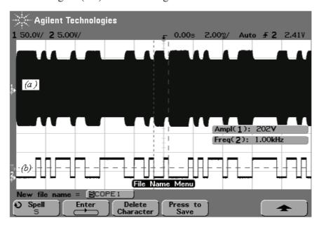
Figure (5.4) illustration of the ASK modulator (a), TX-PN code signal (b)
