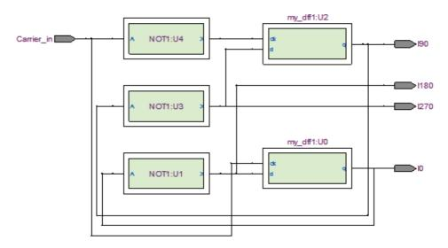
Figure (4.26) Structural VHDL Simulation for carrier phase shifter
