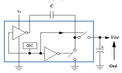
Figure (3.63) demonstrate the circuit of charging pump [136]
