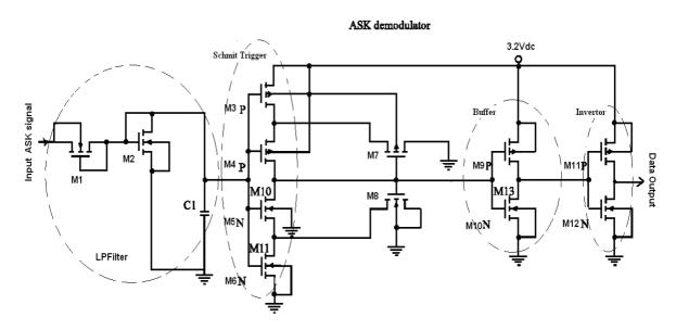
Figure (5.17) the ASK Demodulator circuit using MOSFET
