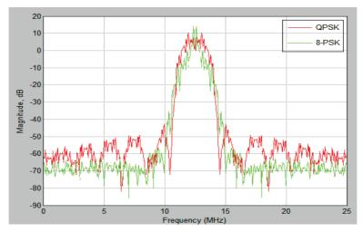
Figure (3.79) the simulation spectrum of n-PSK transmitted signals at carrier 12.5MHz
