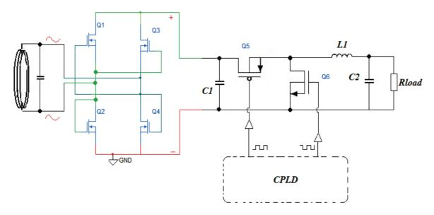
Figure (3.65) demonstrate the RF-Dc to Dc switch converter
