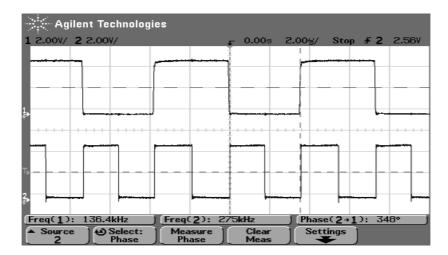
Figure (5.26) comparing the converted digital pulse and the reference pulse
