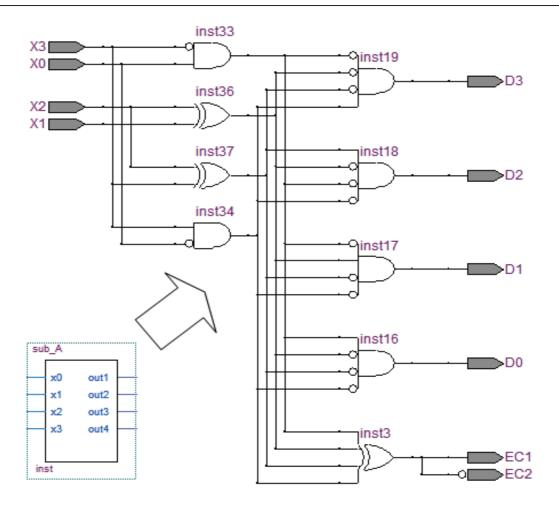
Figure (5.10) the code Inputs/Output with VHDL for the logic control circuit
