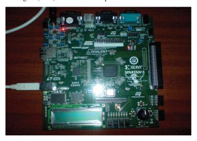
Figure (B1.1) the Xilinx development board FPGA /CPLD
