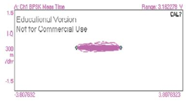
Figure (4.40) the constellation diagram of BPSK at demodulator using Agilent digital demodulator (E8408A)
