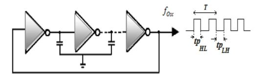
Figure (2.26) the *ring* oscillator principle
