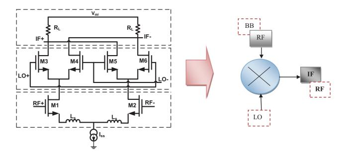
Figure (2.35) the Gilbert mixer working in RF circuit
