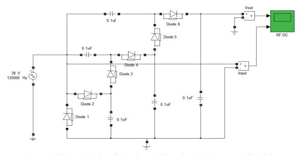
Figure (3.68) the simulation of the voltage doublers circuit with MATLAB/Simulink
