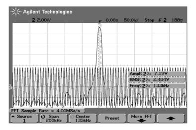
Figure (3.44) the spectrum of carrier frequency at 135 kHz
