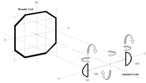
Figure (3.22) Optional solution for splitting the implant coils in to two parts
