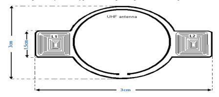
Figure (C1.10) our first proposed geometry design for UHF and power spiral coils
