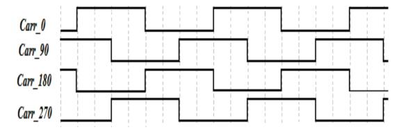
Figure (4.30) the simulation waveforms for modified carrier phase shifter
