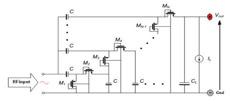
Figure (3.57) voltage multiplier based on NMOSFET [178]
