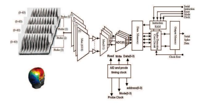
Figure (1.13) the architecture of Utah microelectrodes array [151]
