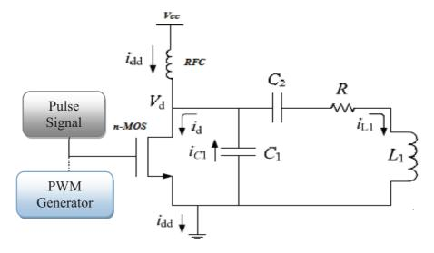
Figure (3.31) the principle circuit of the Class E amplifier
