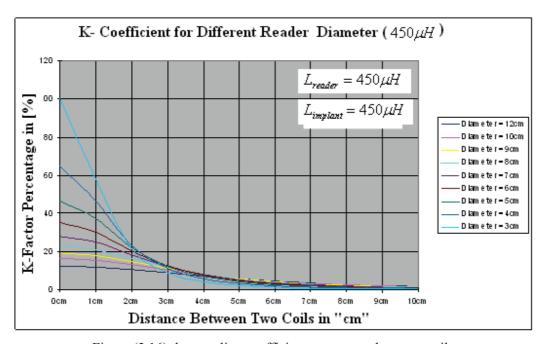
Figure (3.16) the coupling coefficient percentage between coils
