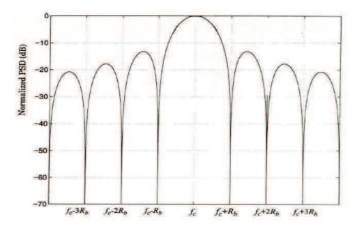
Figure (2.11) Spectrum for the BPSK Signal
