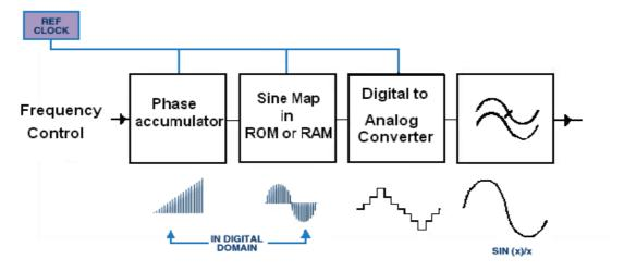
Figure (2.22) the architecture of DDS Block diagram
