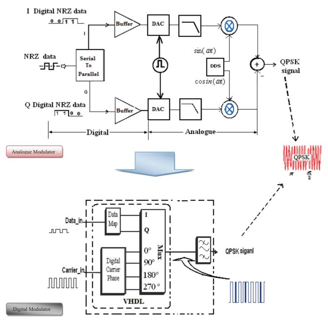
Figure (4.16) Block diagram of the proposed digital VHDL QPSK Modulator
