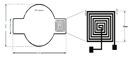
Figure (C1.9) geometry of the typical rectangular spiral coil for implant device [205]
