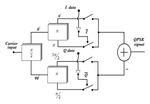
Figure (4.17) the concept (A) for generating direct QPSK digital modulator
