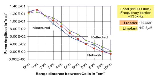
Figure (3.9) shows a comparison of theoretical methods and measured received power at Load (8500 $\Omega$ )
