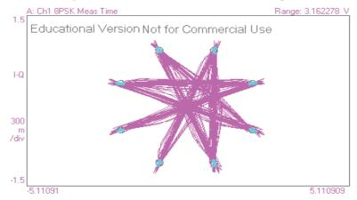
Figure (4.48) Constellation diagram of 8PSK demodulator Received from the proposed VHDL 8PSK modulator
