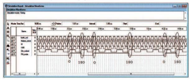
Figure (4.15) the waveforms simulation of the BPSK Proposed Modulator
