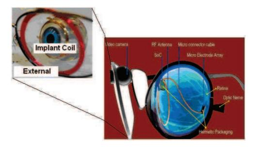
Figure (1.4) Principle architecture of the retinal implant device [198]
