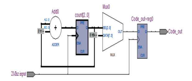
Figure (5.13) the PN sequence generated by VHDL code (B)
