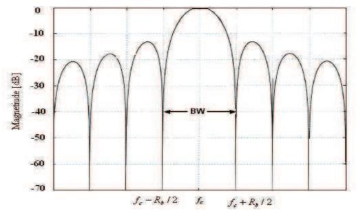
Figure (2.18) the Spectrum density for QPSK Signal
