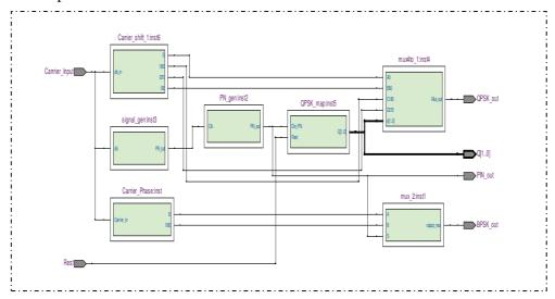
Figure (C1.4) the BPSK/ QPSK modulator/demodulator generated by VHDL
