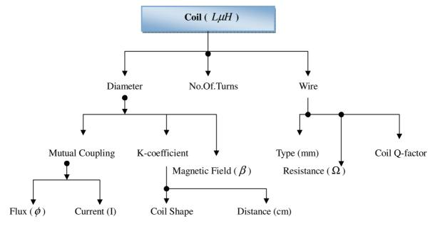
Figure (A1.6) Most common factor parameters for coil design
