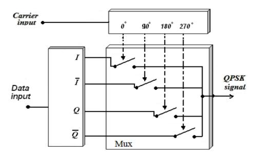
Figure (4.19) the concept (C) for generating the Direct QPSK digital modulator
