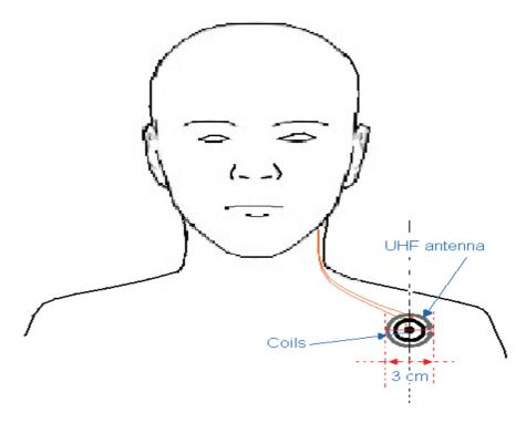
Figure (3.26) demonstrates the combined solution for implant coil location
