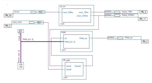
Figure (5.29) the simulation result generating VHDL code for PWM signal
