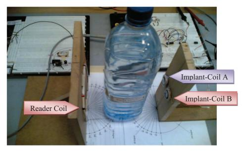
Figure (3.24) the RF inductive coupling lab measurements for dual coils
