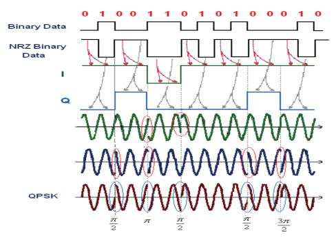
Figure (2.16) illustrates the QPSK waveform with respect to binary and NRZ states
