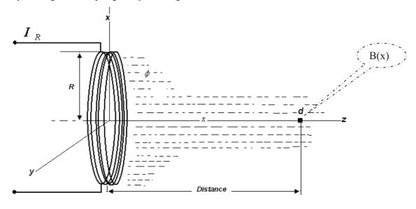
Figure (3.14) the loop coil geometry compared to magnetic flux
