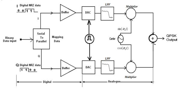
Figure (2.17) the block diagram of conventional QPSK modulator
