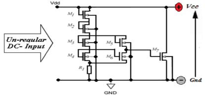
Figure (3.62) the circuit of voltage regulator [4]
