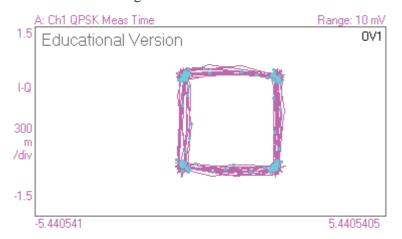
Figure (4.44) Constellation diagram of QPSK demodulator, received from the proposed VHDL QPSK modulator
