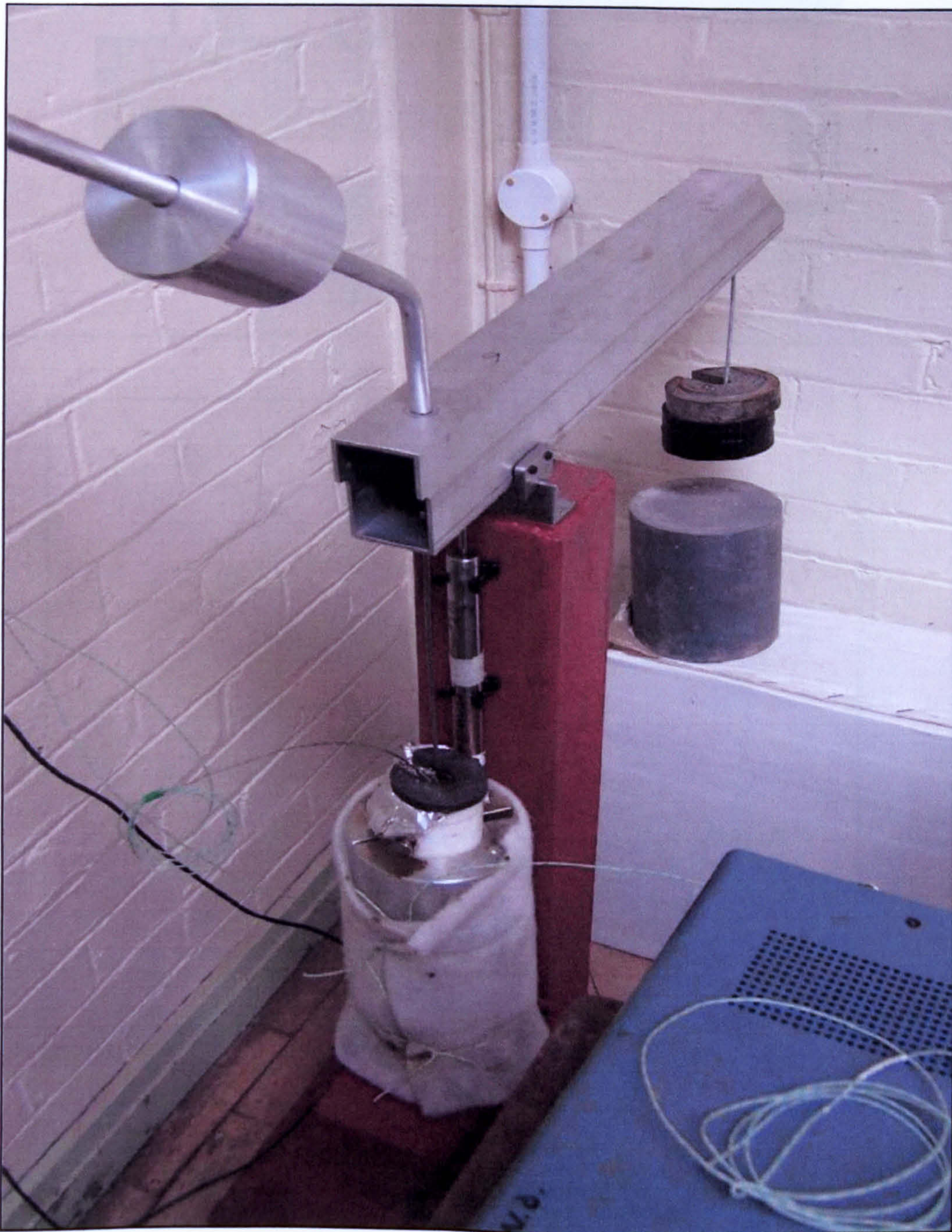
Figure 3.1 Photograph of: (B) the Vertical rigs for environmental testing
