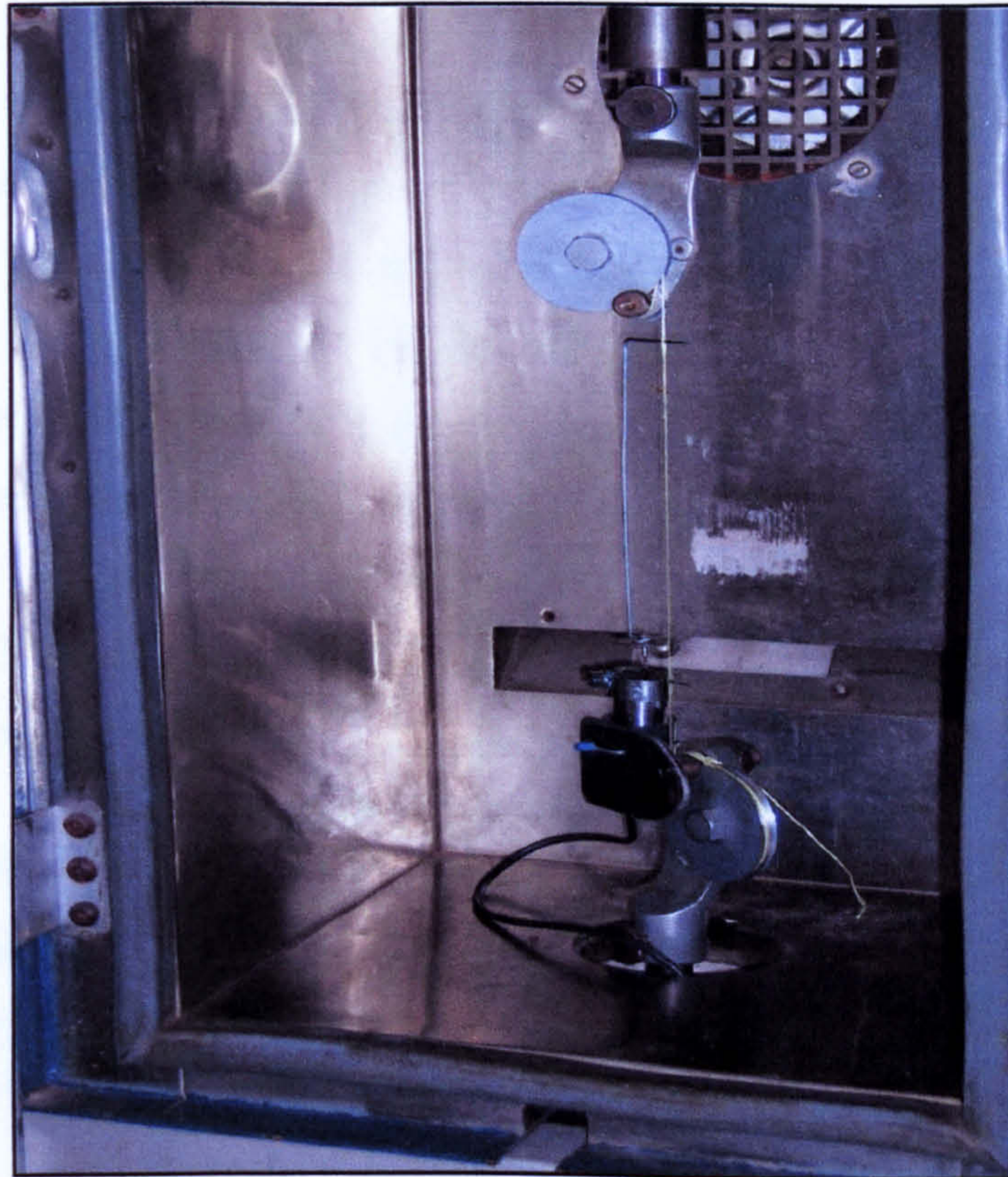
Figure 3.5 Close-up of the temperature controlled oven used for high temperature tests on the hydraulic Instron mechanical testing machine
