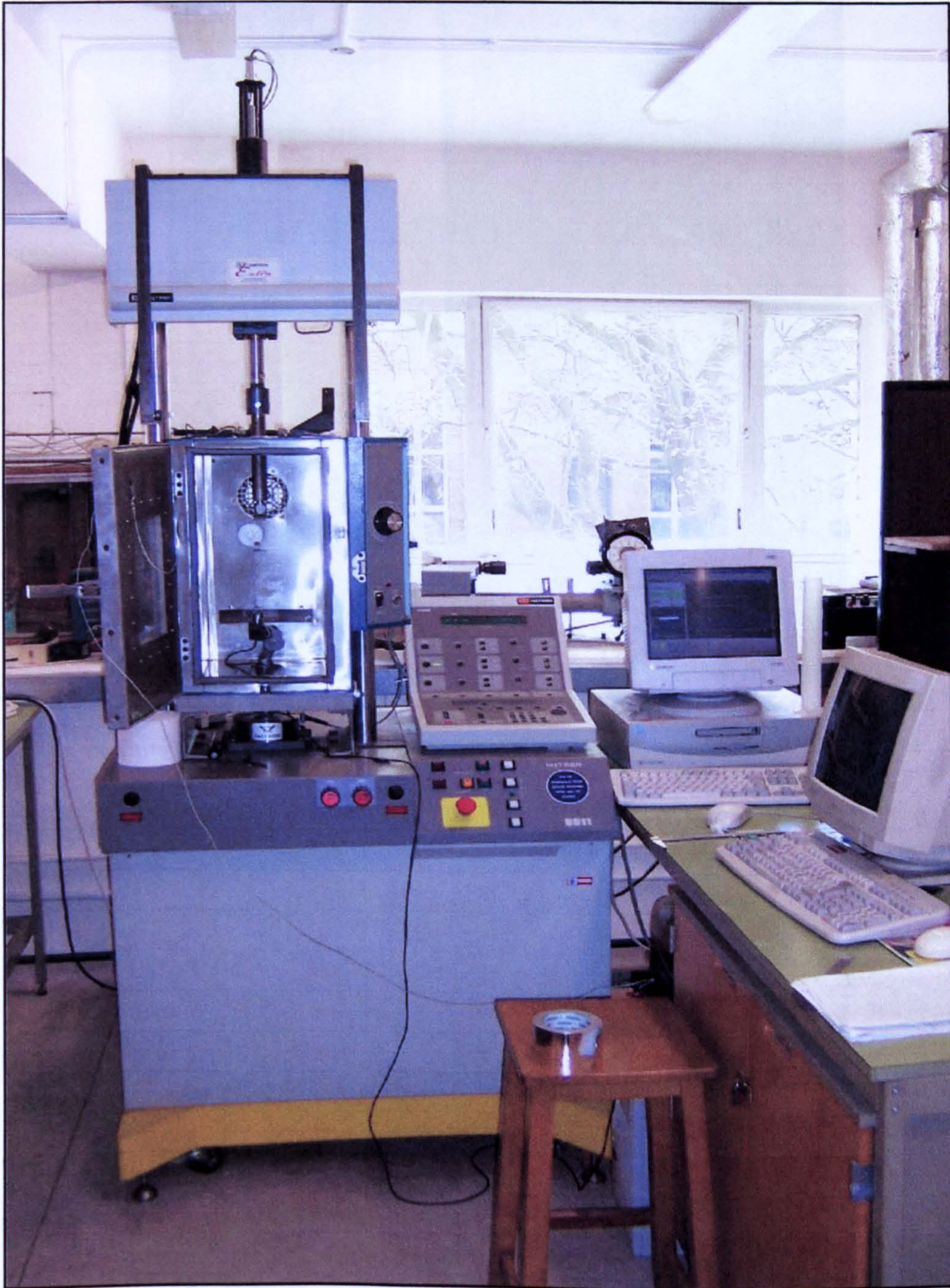
Figure 3.4 Computer controlled hydraulic Instron mechanical testing machine used to break the samples in tests of very long duration
