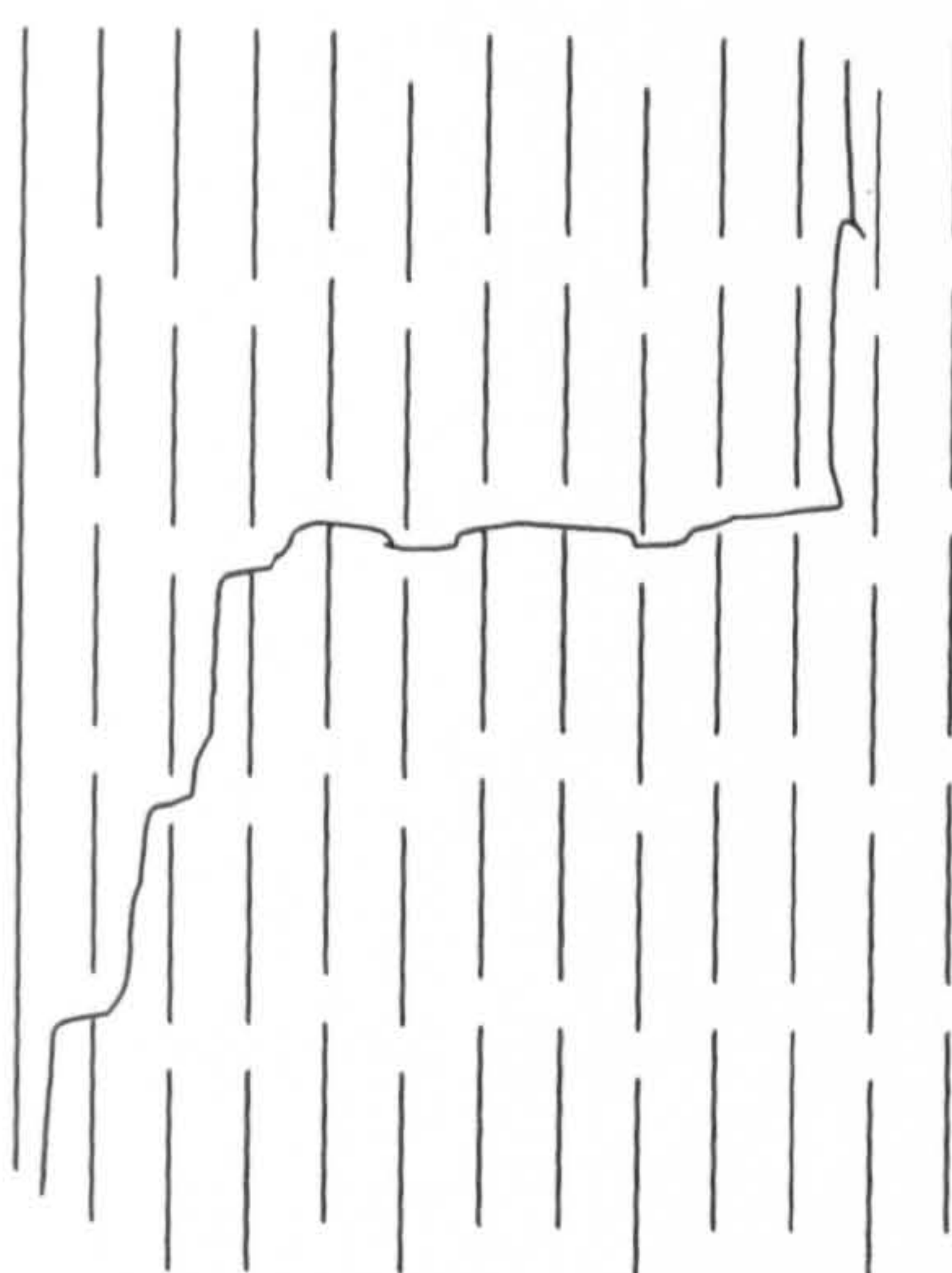
Figure 7.5 Schematic of the crack propagation path
