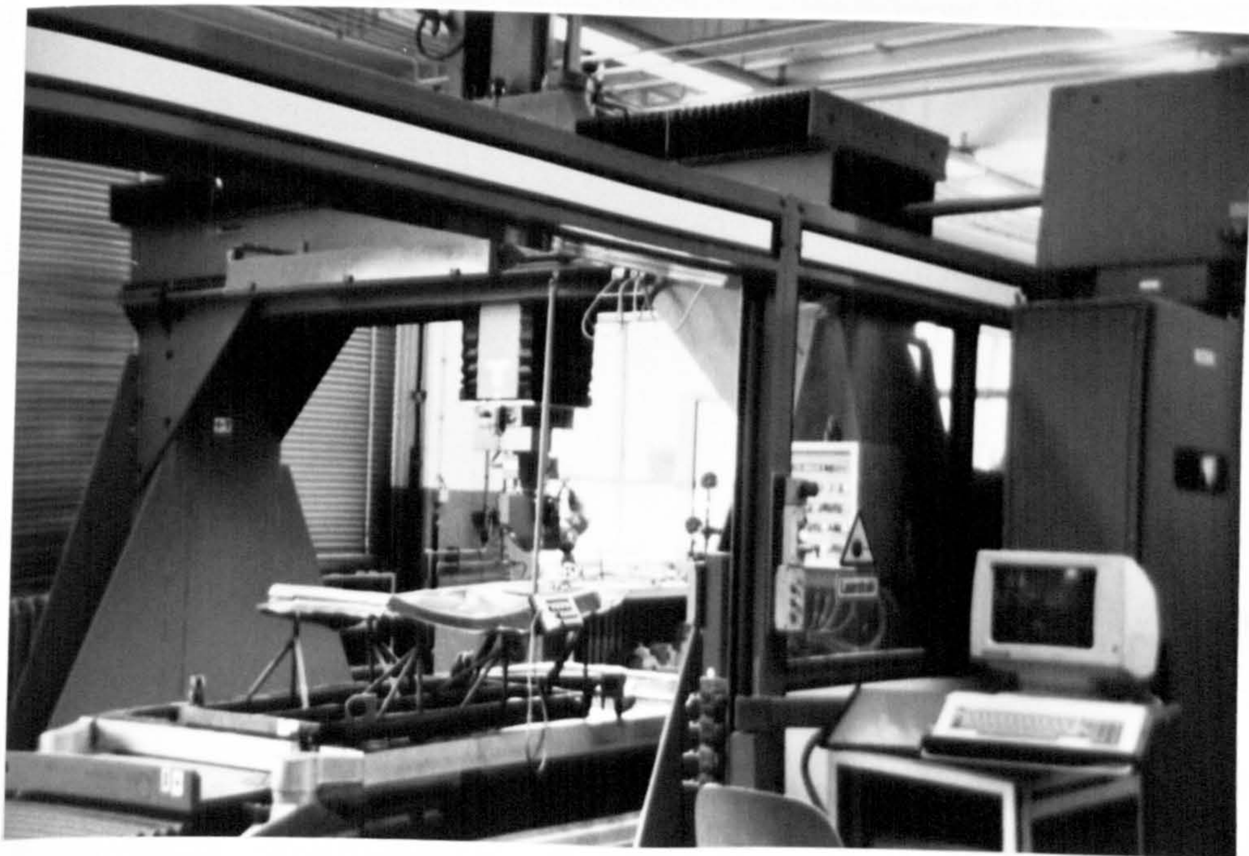
Figure 7.07b- Gantry mounted five axis production system
