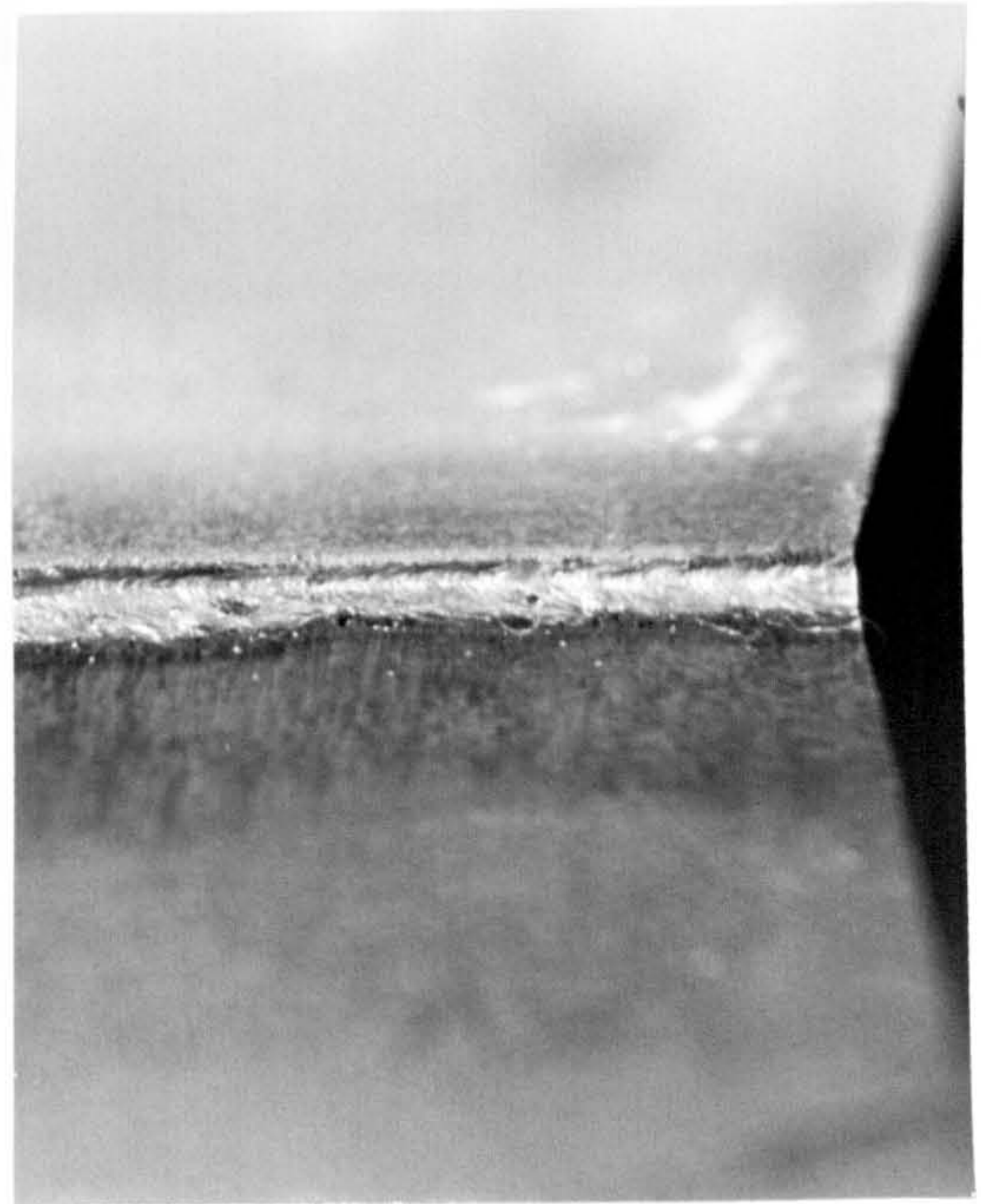
Figure B4.05a - Surface profiles of the incident bead (l) and emergent bead (r) beads in 12mm plate (power = 9kW)
