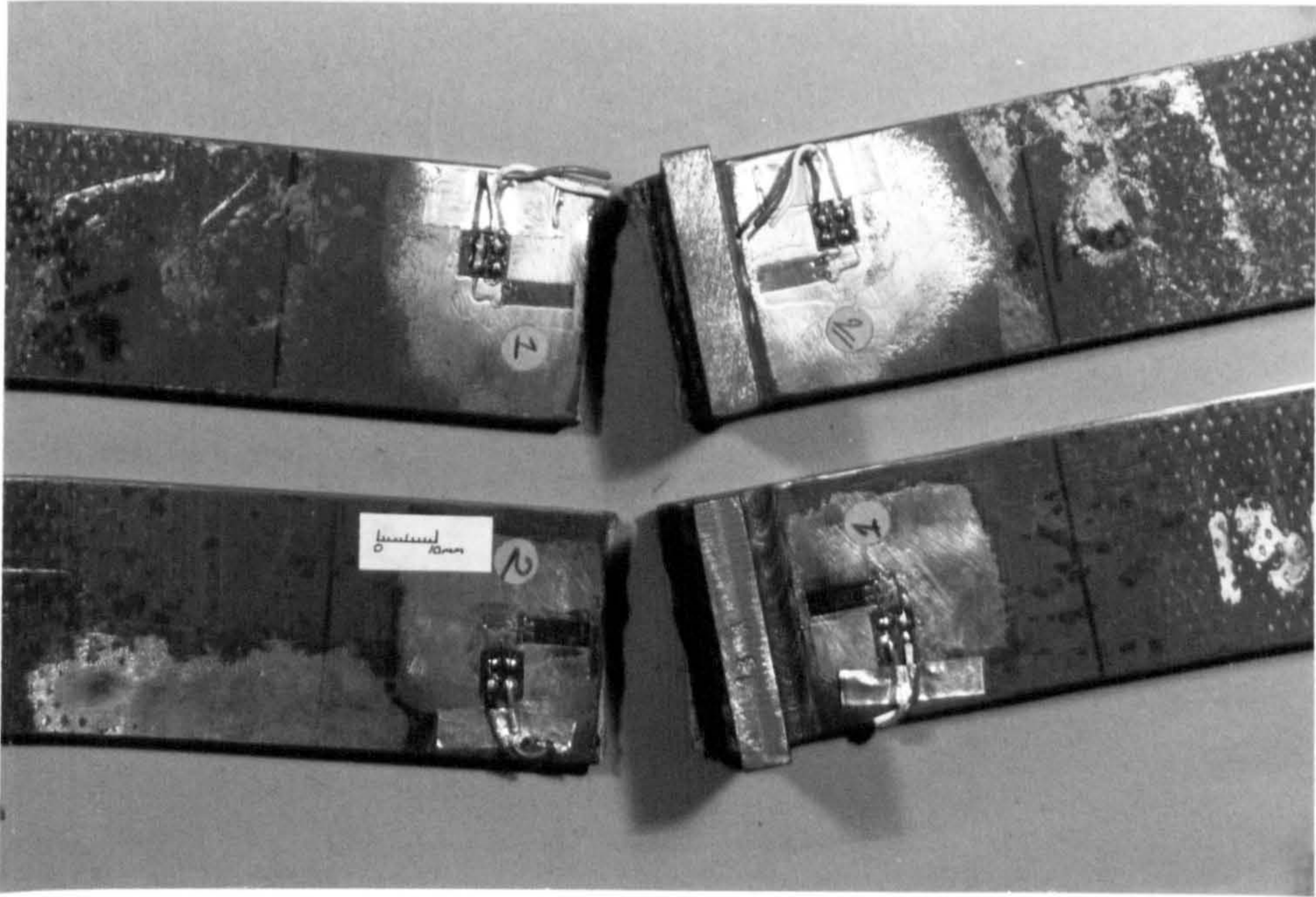
Figure 5.18a - Fatigue failure in the weld toe for non-loaded stiffeners, laser skid and MMA twin fillet welds
