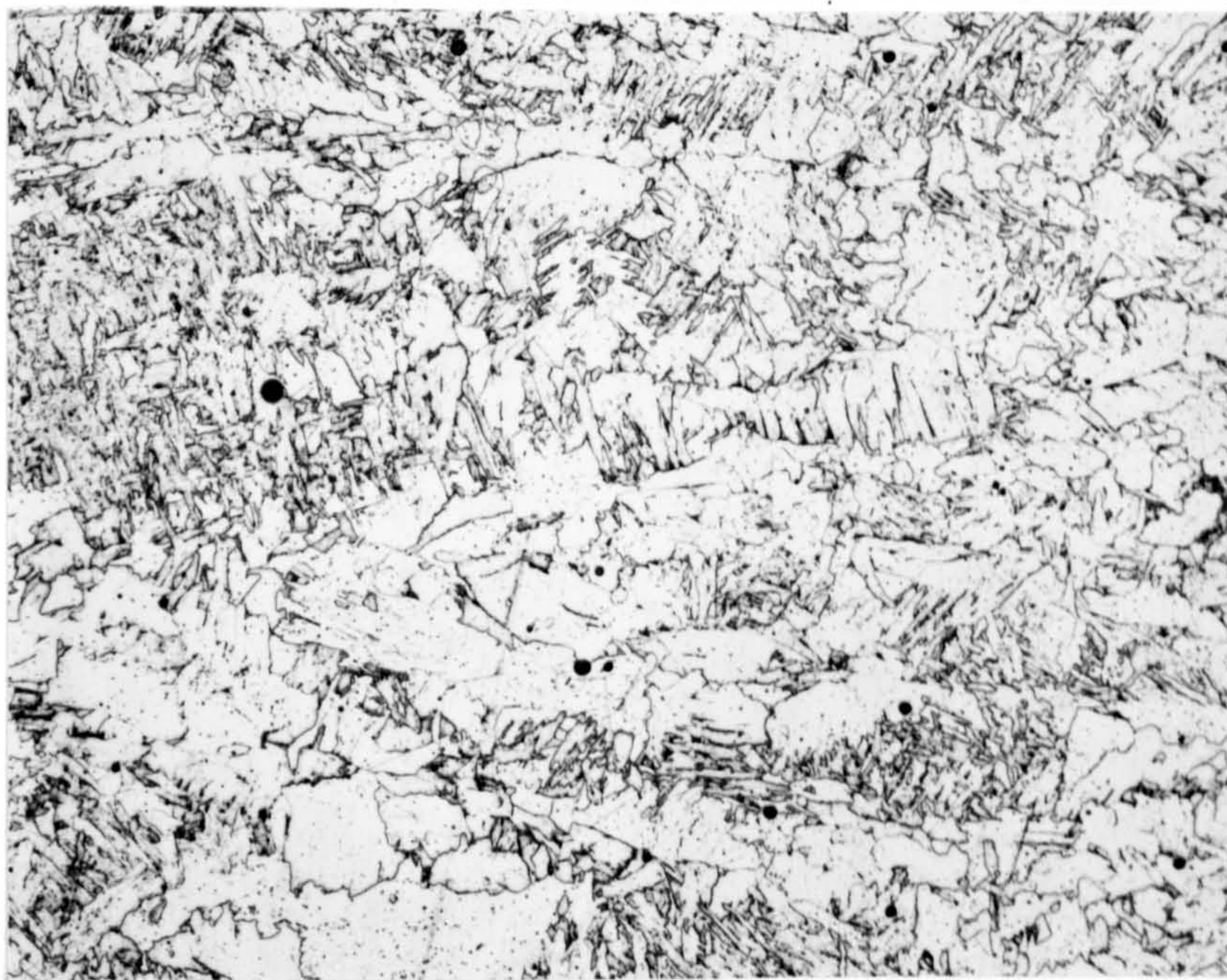
Figure 6.20b - 8mm MMA weld fillet - large areas of GF (x200).
