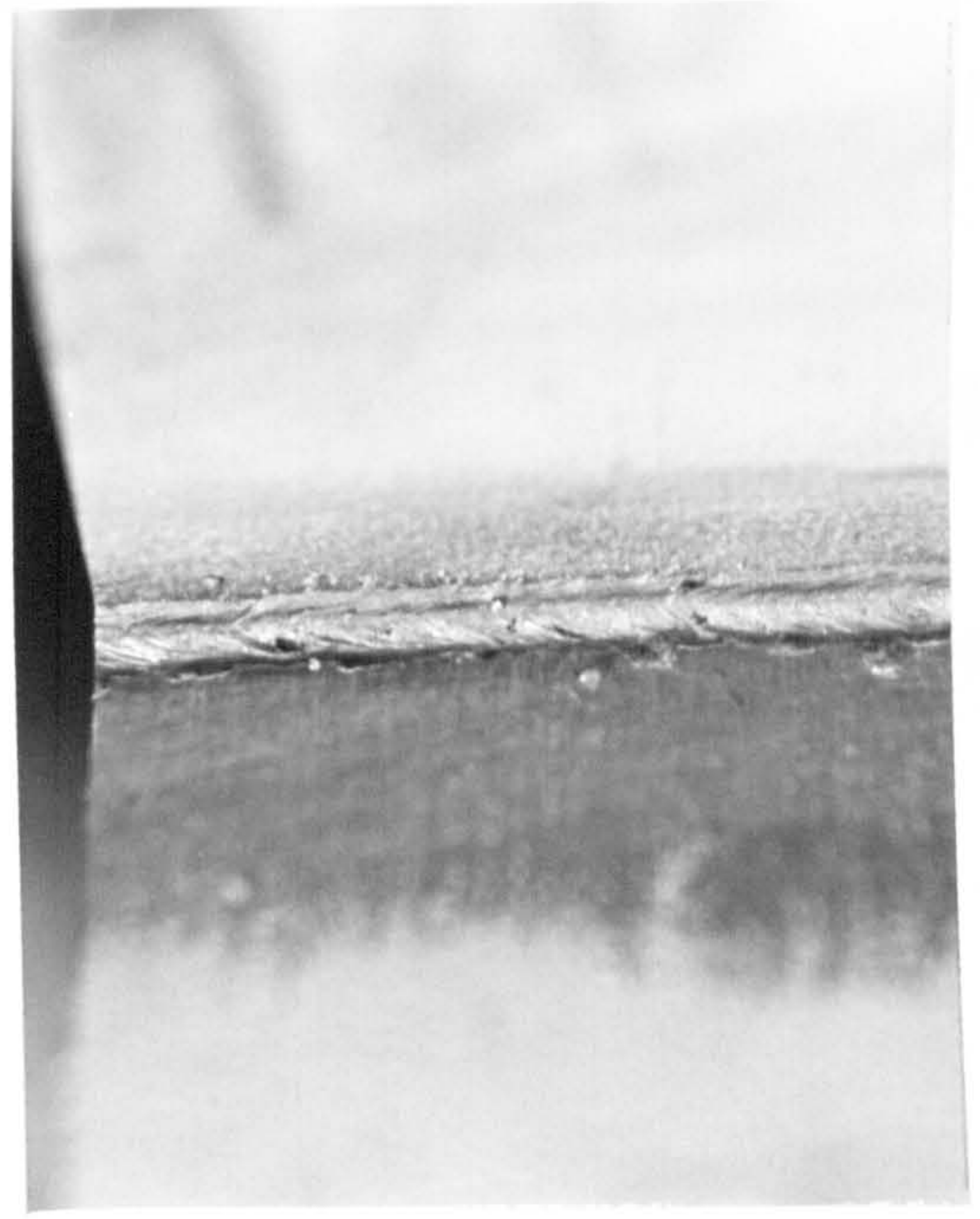
Figure B4.03a - Surface profiles of the incident bead (l) and emergent bead (r) beads in 8mm plate (power = 9kW)
