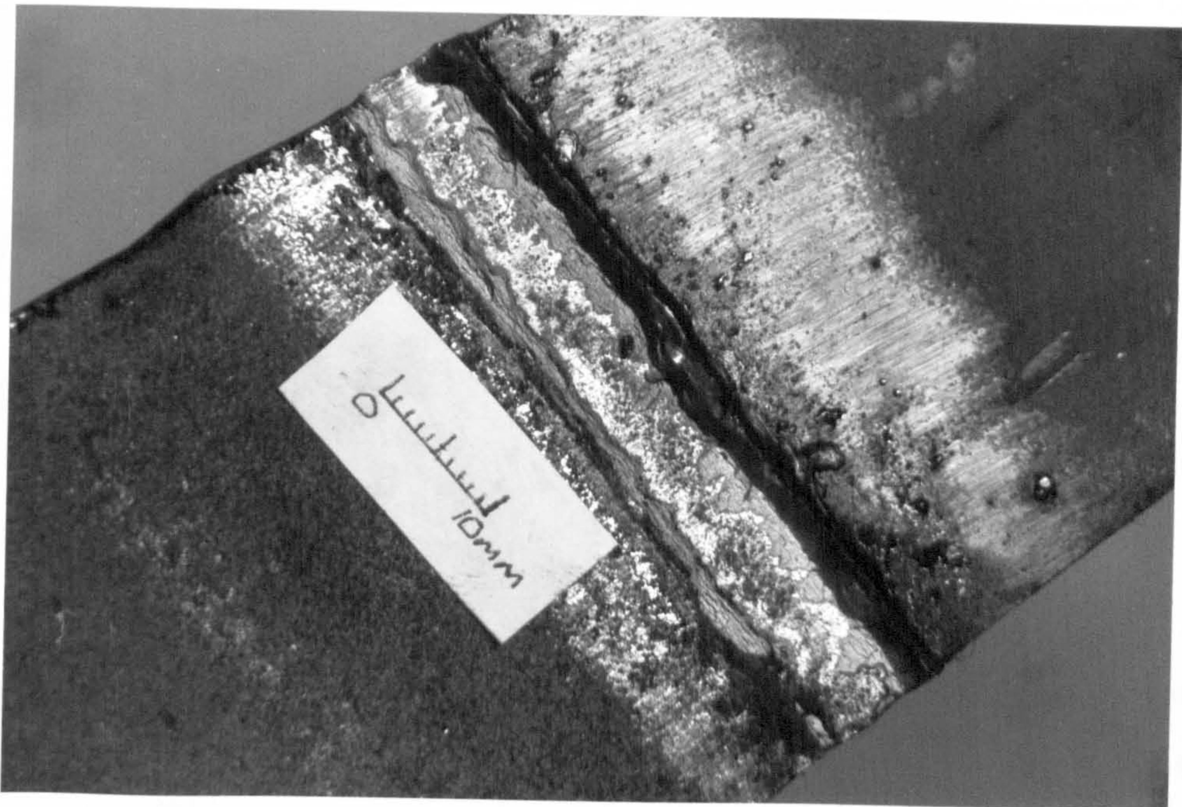
Figure 5.04 - Defect (lack of fusion) identified in the skid weld during tensile testing
