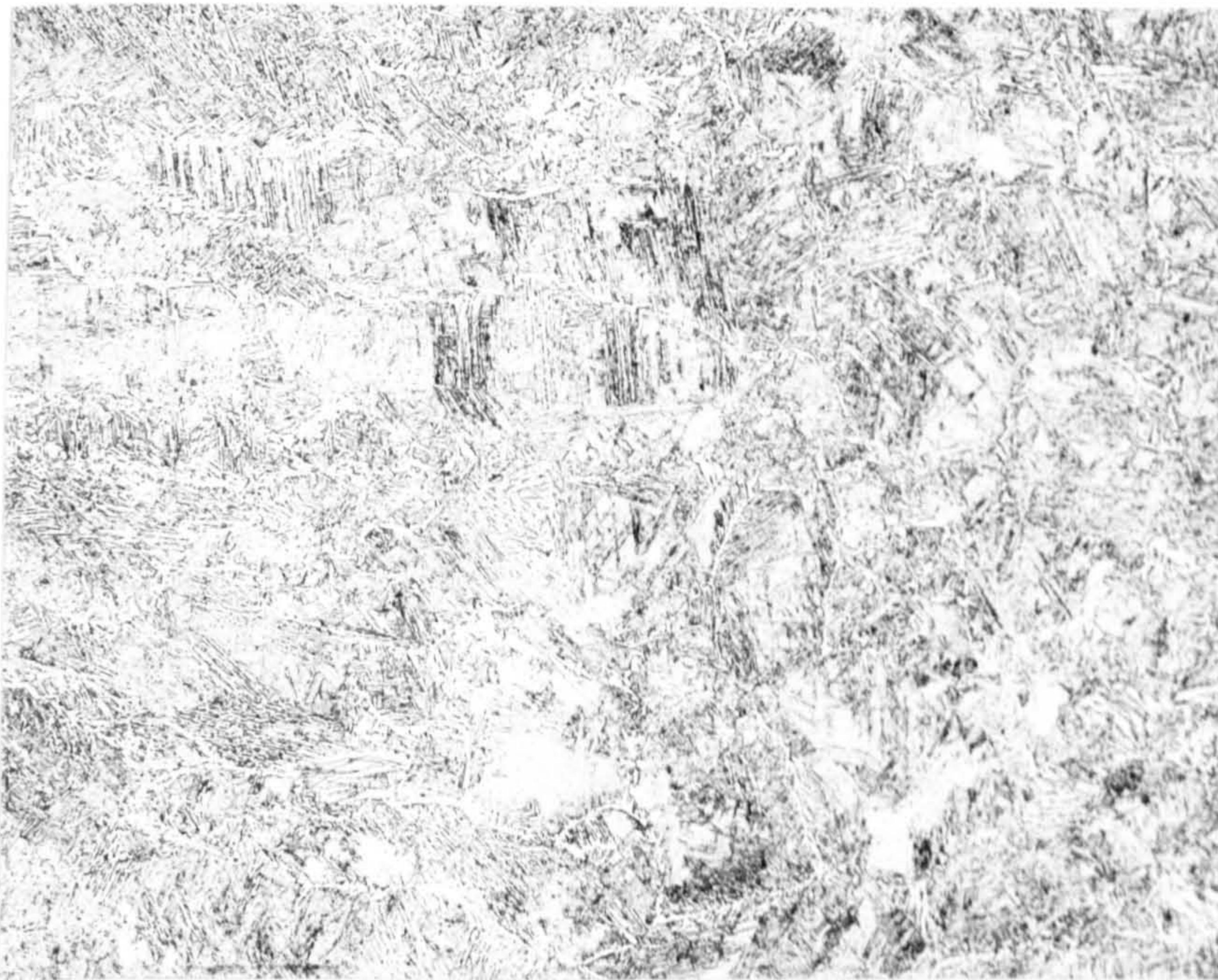
Figure D6.04b - Skid weld in 12mm plate; fusion line (x200)
