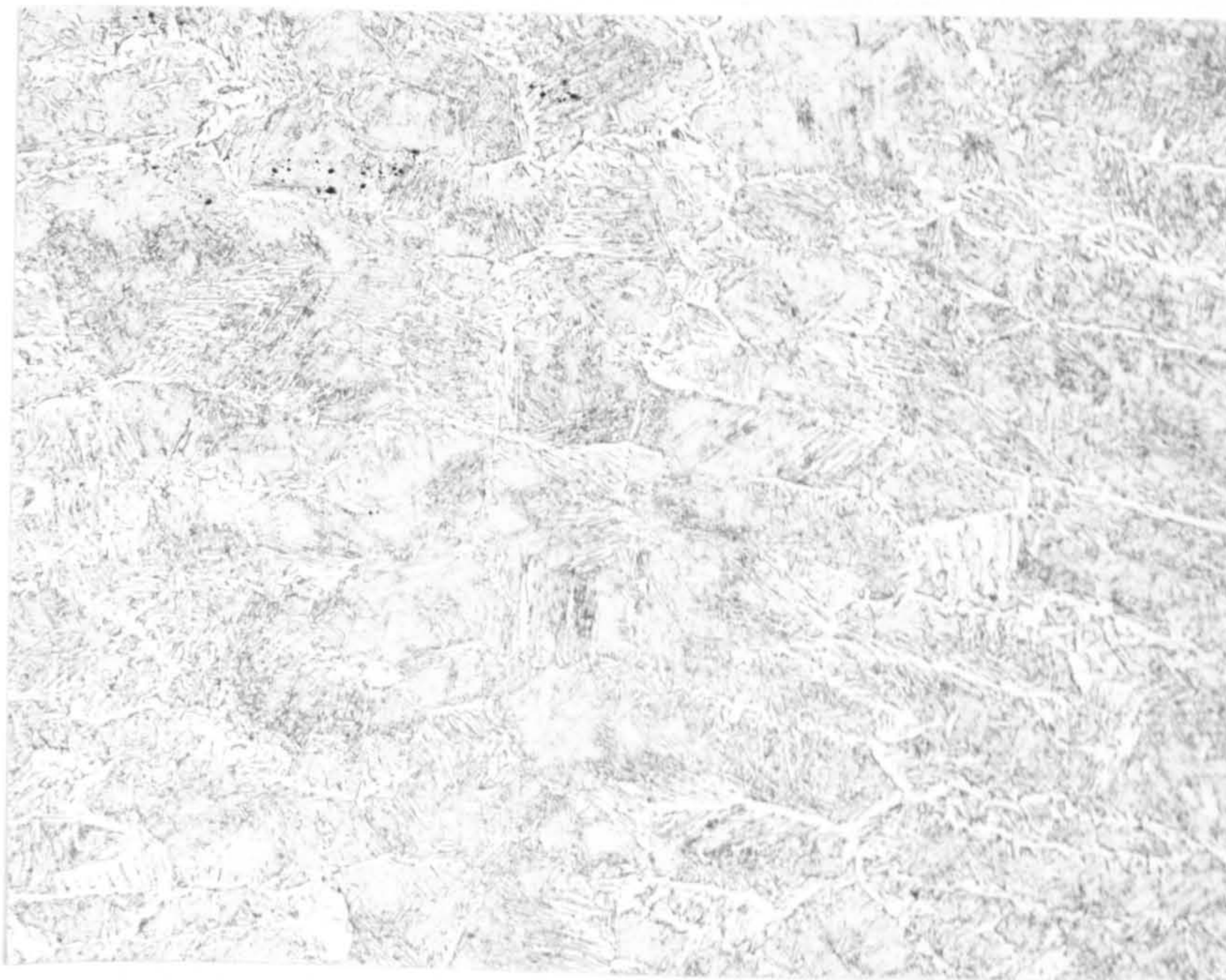
Figure D6.03b - Weld material within 10mm skid weld centreline; columnar grains meeting centreline equiaxed zone (x200)
