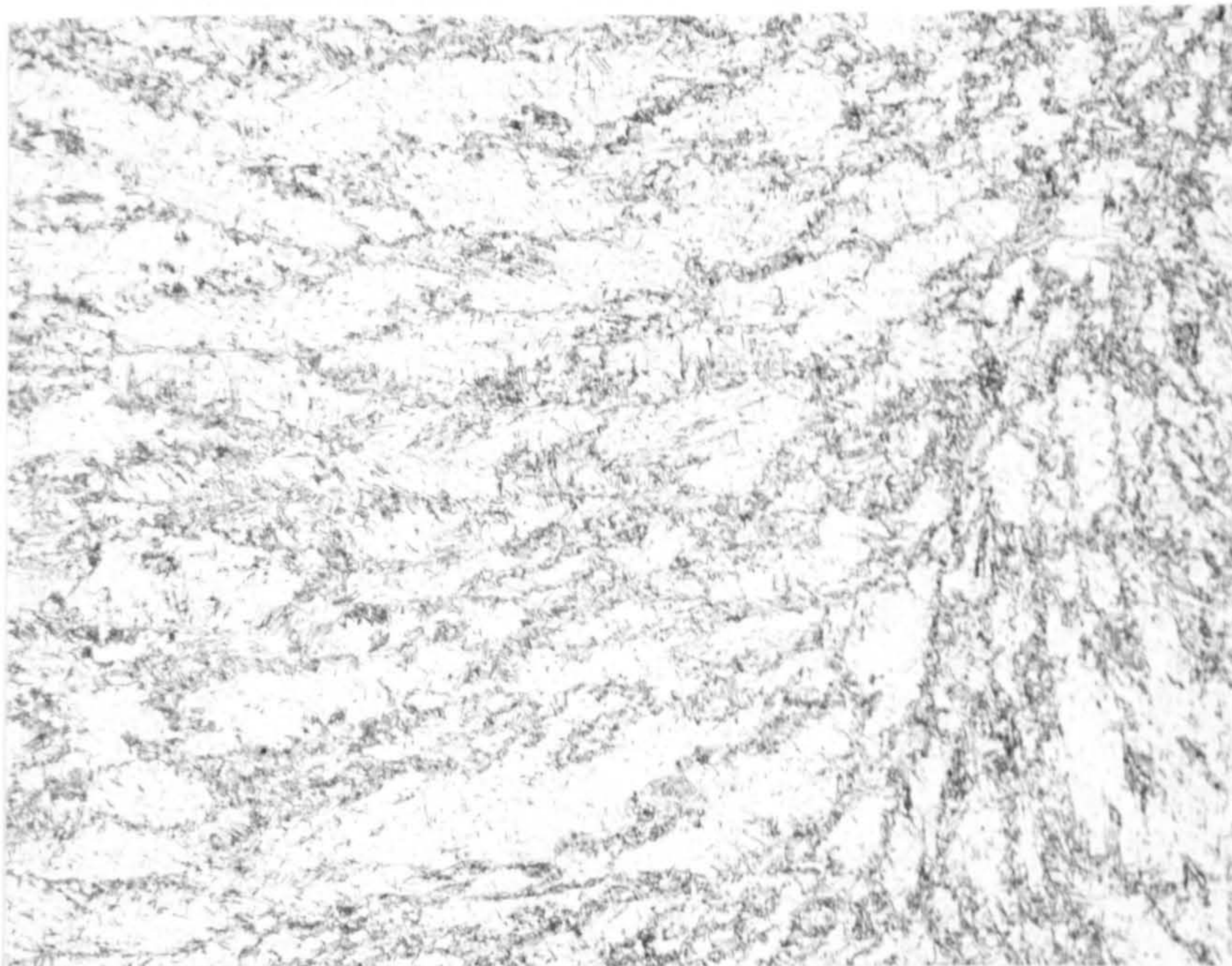
Figure D6.01b - Weld material within a 3mm skid weld ; coarse grains of transformed martensite (x200)
