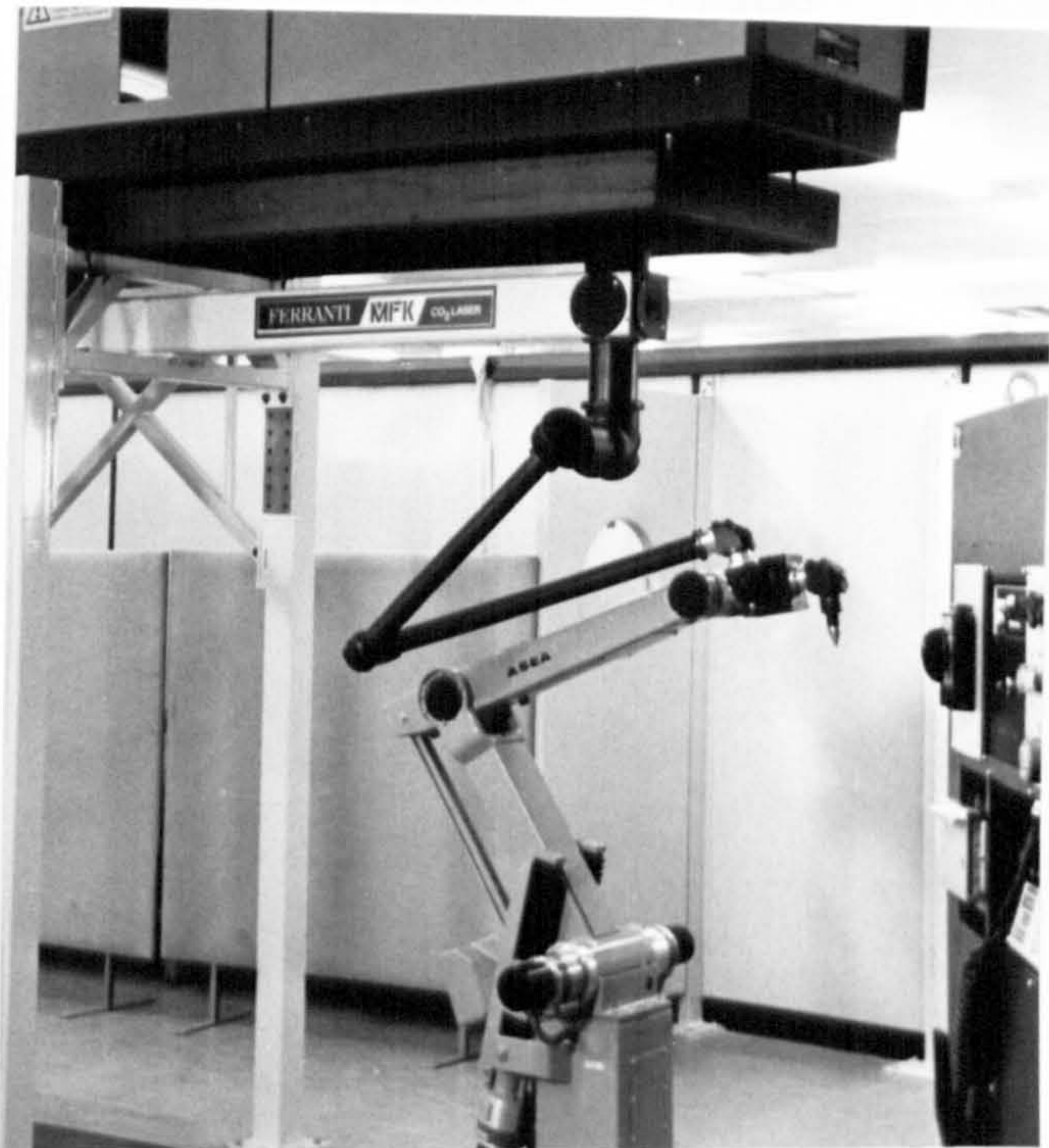
Figure 7.06a - Flexible beam guide linking the laser to the robots end
