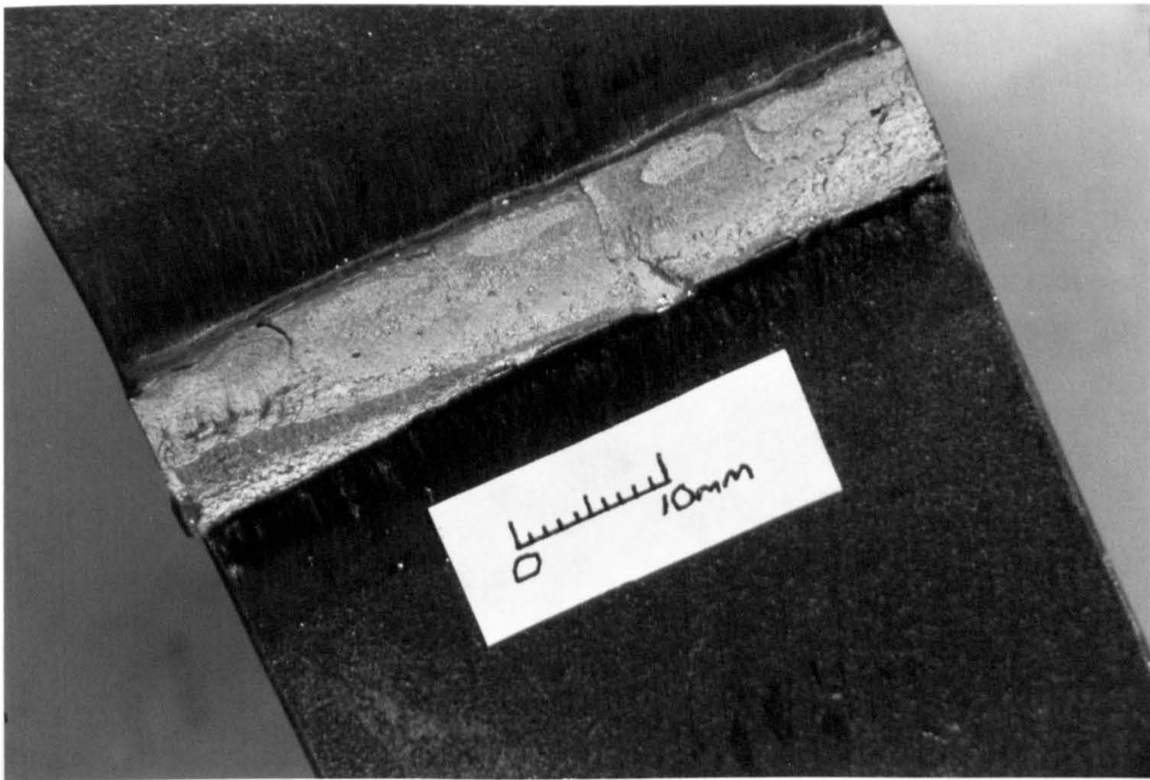
Figure 5.21 - Fatigue crack surface showing areas of weld defects
