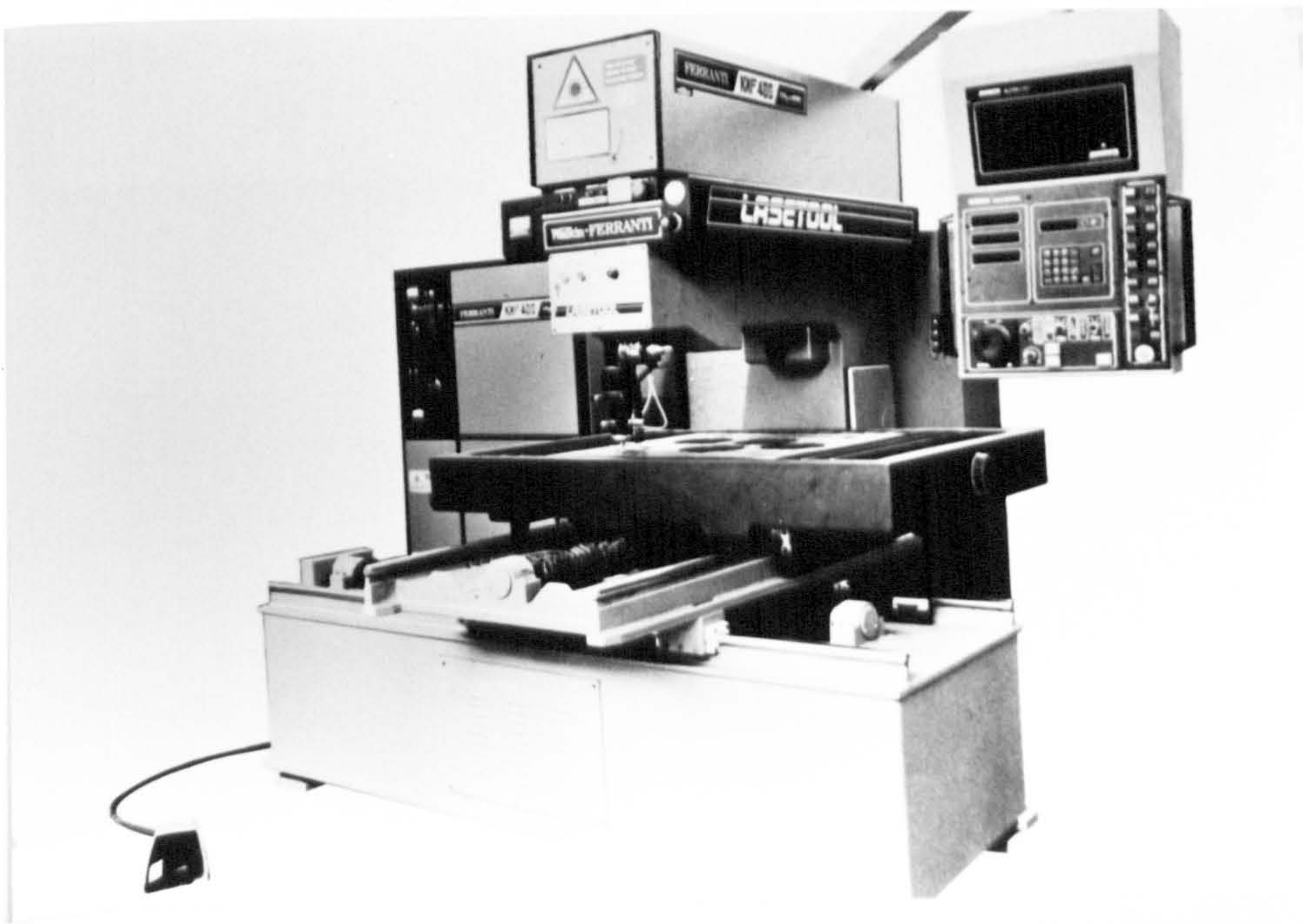
Figure 7.10 - Laser integrated into an existing machine tool design
