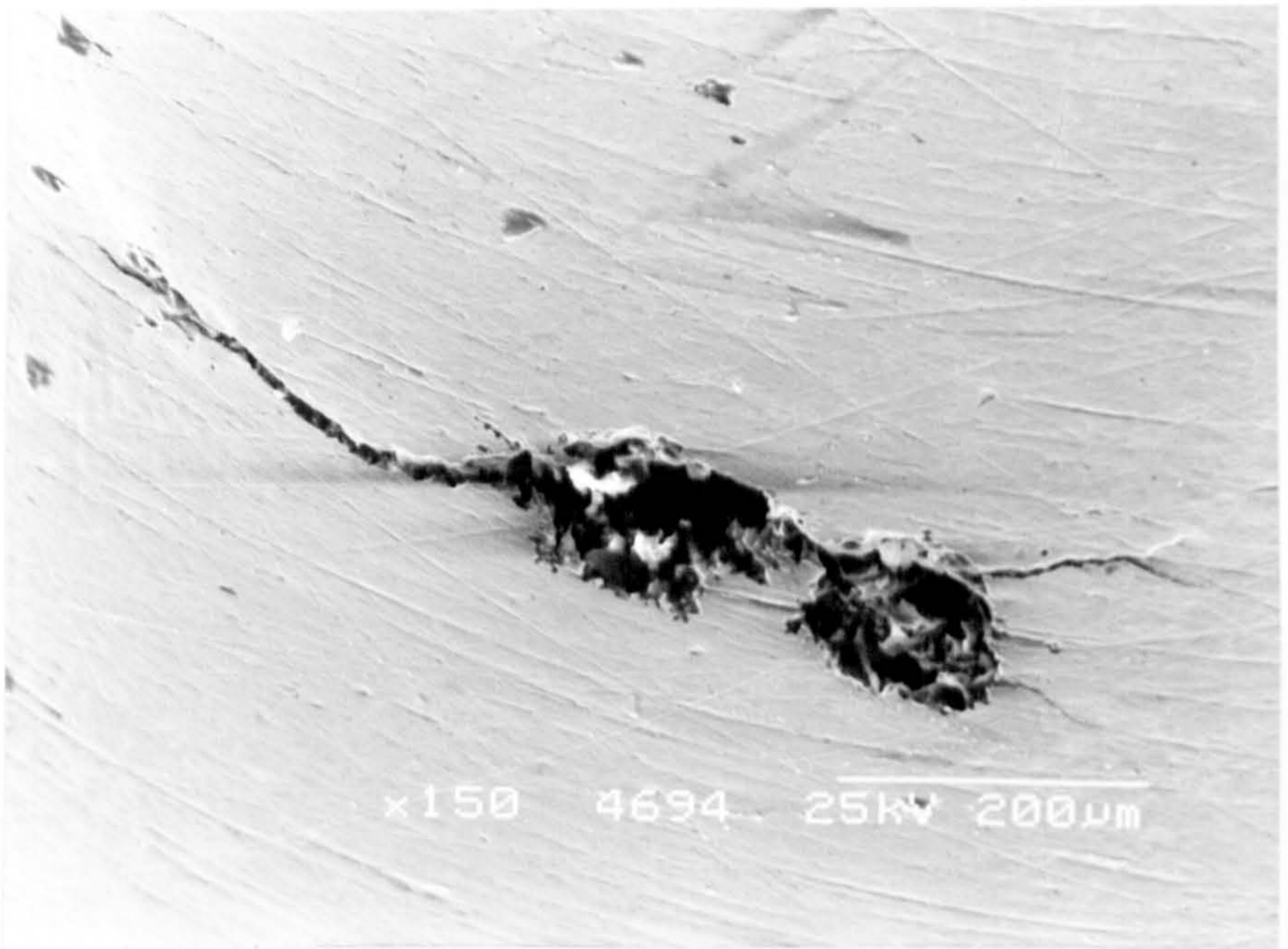
Figure 4.44 Cracks initiated at pits in a specimen strained to failure in NACE-01-77 solution at 80°C.
