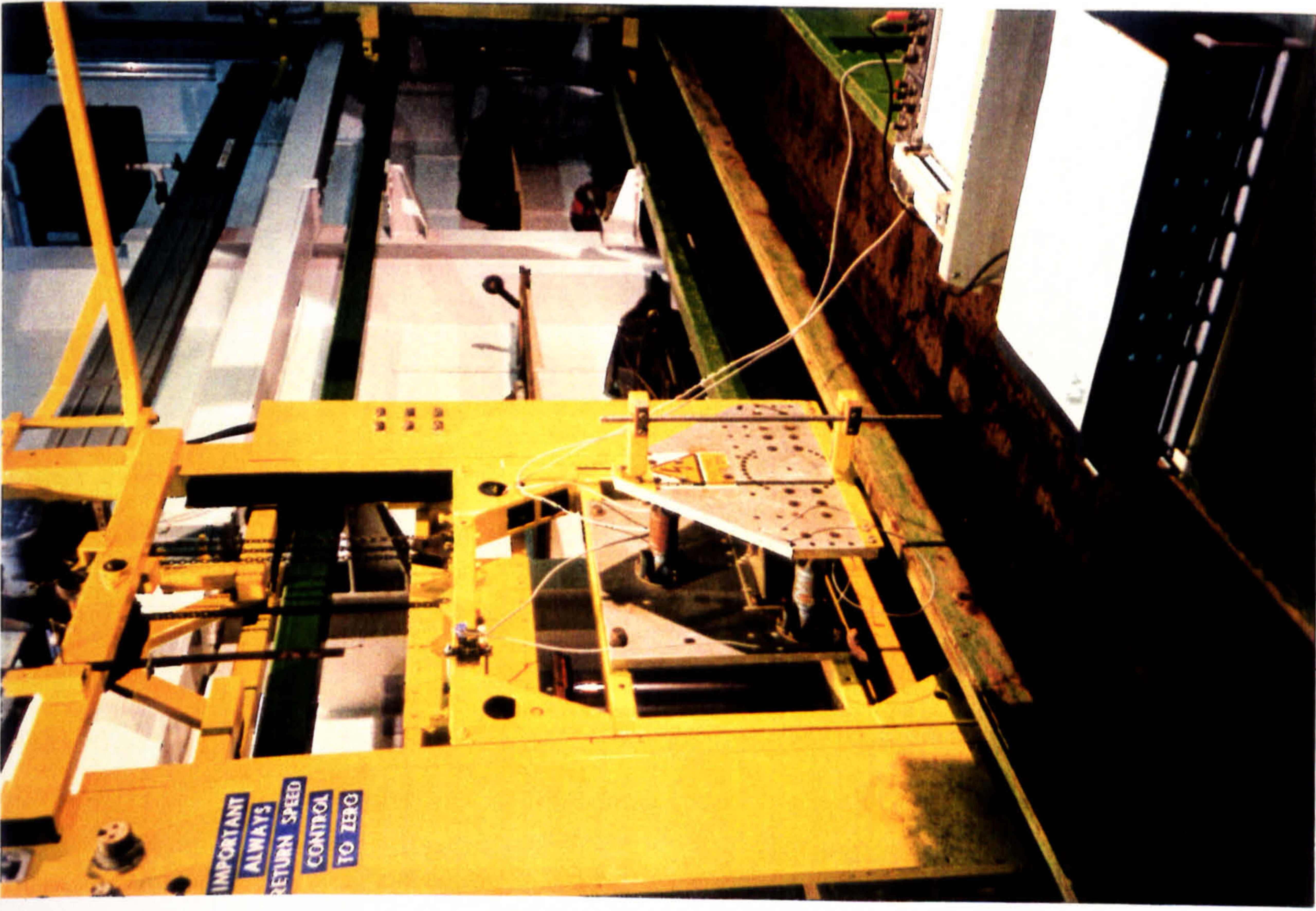
Fig. 7.32 (a) Cones with different geometry and surface roughness used in the Soil-tank experiment. (b) The complete experimental set-up of the cone penetrometer test in the Soil-tank.
