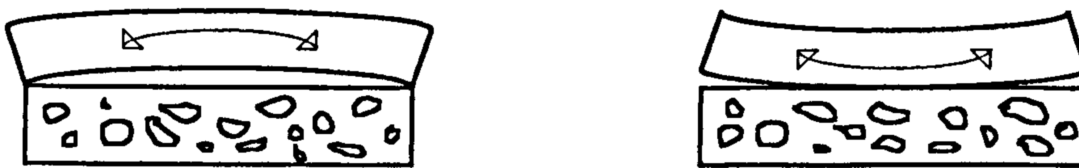
Figure 3-4: Curling and debonding of the screeds due to the thermal shock Mwape, in his research, has concluded that in most cases, the bond strength has not been affected by the thermal shock experiments. [ Mwape 1990 ]
